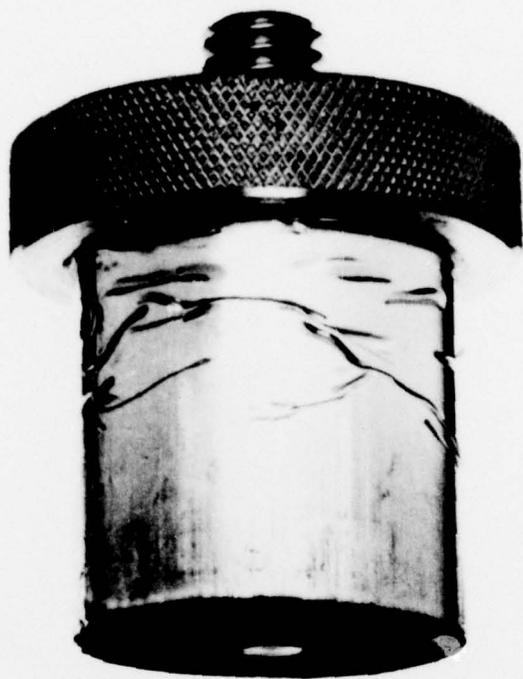
FIG. 3(b) - External appearance of the exothermic compact.
