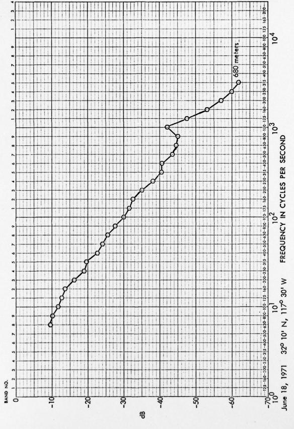
SOUND PRESSURE SPECTRUM LEVEL (reduced from 1/3 octave) as re 1 dyne/cm $^2$
