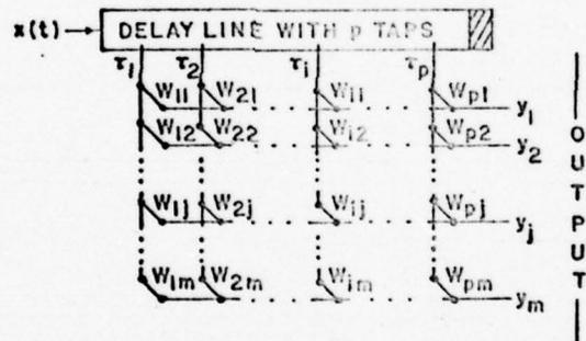
Fig. 7. Multiple-Output-Port Transversal Filter.
