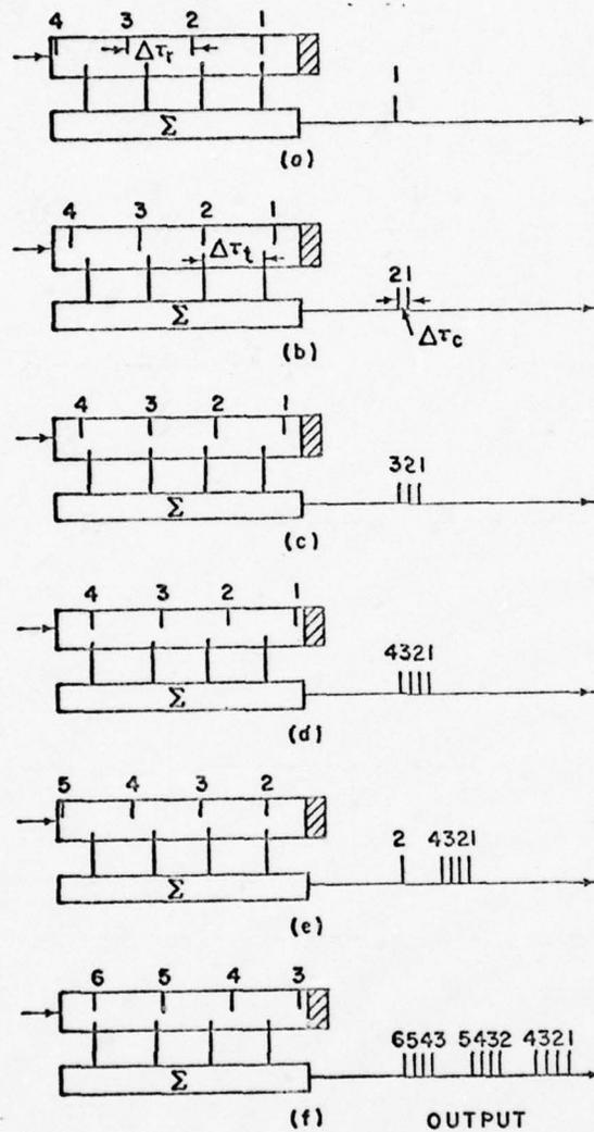
Fig. 6. Transversal Filter Time Compressor,  $p = 4$ . Relative positions in space of the output samples are shown on the right for specified time delays: (a)  $t = 0$ ; (b)  $t = \Delta\tau_c$ ; (c)  $t = 2\Delta\tau_c$ ; (d)  $t = 3\Delta\tau_c$ ; (e)  $t = \Delta\tau_r$ ; (f)  $t = 2\Delta\tau_r + 3\Delta\tau_c$ .
