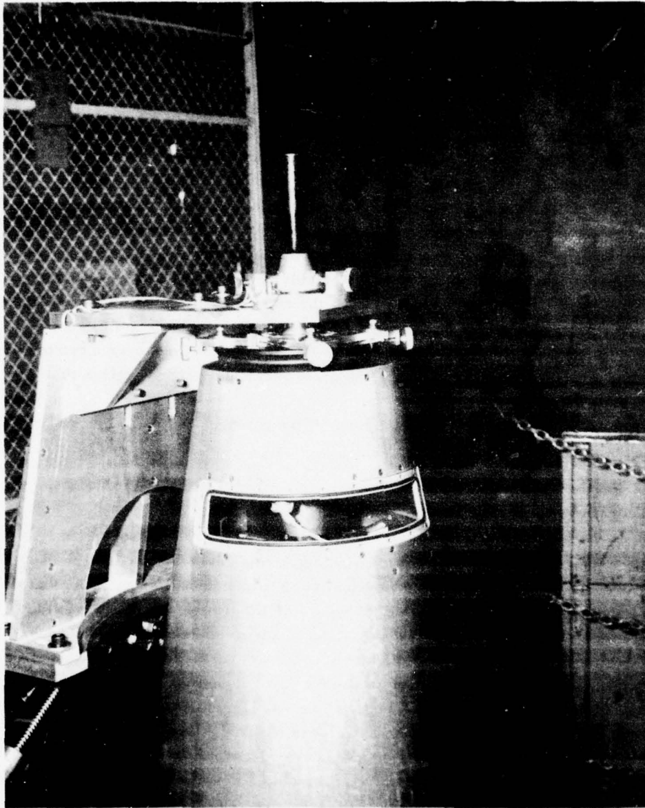
Figure 5. The Constraining Fixture for the Balancer. The payload on the balance is prevented from tipping over by a fixture which limits the travel of the top end of the payload. Also seen are the two precision levels mounted in the payload which are used for the initial static balance
