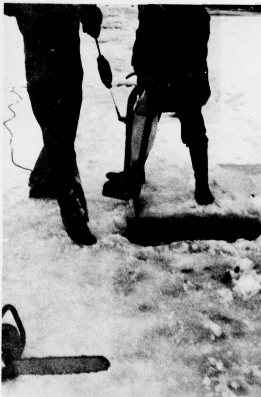
Figure B4. Preparing to lower Helley-Smith bed-load sampler.
