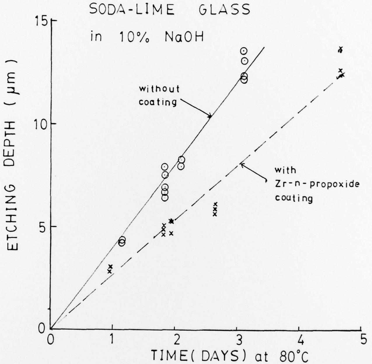
NaOH etching rate of soda lime glass with and without Zr-alcoxide coating.
