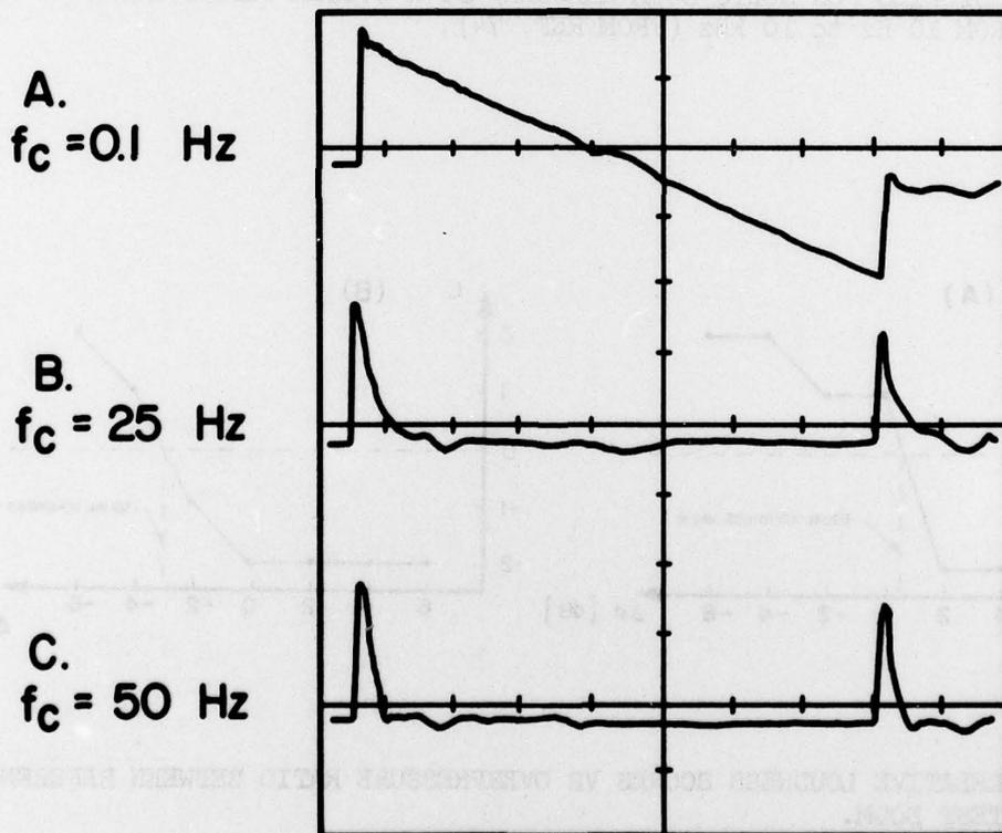
FIG. 13 EFFECT OF HIGH PASS FILTERING ON SONIC BOOM SIGNAL (PRESSURE WAVEFORMS RECORDED IN UTIAS SIMULATION BOOTH). N-WAVE SIGNATURE:  $\tau = 1$  ms;  $D = 150$  ms;  $\Delta p = 1$  psf.
