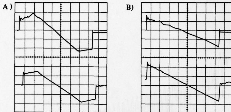
FIG. 8 EFFECT OF "PREDISTORTION" OF ELECTRICAL INPUT SIGNALS (TOP) TO UTIAS SONIC BOOM IN ACHIEVING DESIRED WAVEFORMS (BOTTOM) RECORDED BY MICROPHONE IN BOOTH.
