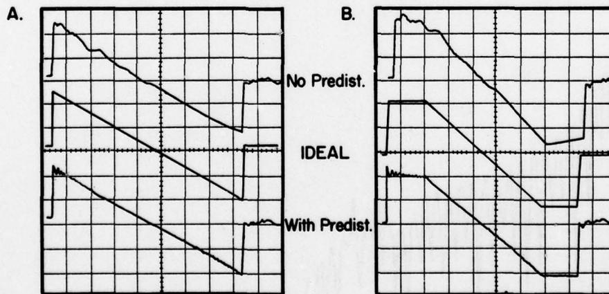
FIG. 9 EXAMPLES OF PRESSURE SIGNALS RECORDED BY MICROPHONE IN UTIAS SIMULATION BOOTH WITHOUT (TOP) AND WITH (BOTTOM) PREDISTORTION OF INPUT SIGNAL.
