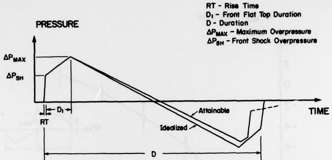
FIG. 20 IDEALIZED VS ATTAINABLE "LOW-BOOM" SONIC-BOOM SIGNATURES. "ATTAINABLE" SIGNIFIES REALIZABLE VIA AIRCRAFT DESIGN AND FLIGHT PROCEDURE.
