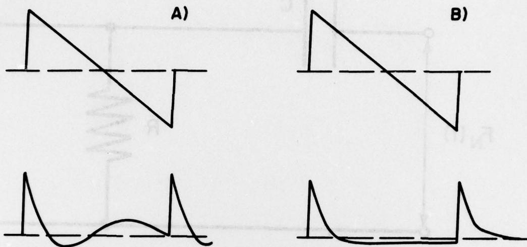
FIG. 14 COMPARISON BETWEEN EXPERIMENTAL (ANALOG) (A) AND PREDICTED (B) TIME HISTORIES FOR SONIC BOOM MEASURED BY A SYSTEM WITH FREQUENCY RESPONSE FROM 10 Hz to 10 kHz (FROM REF. 74).
