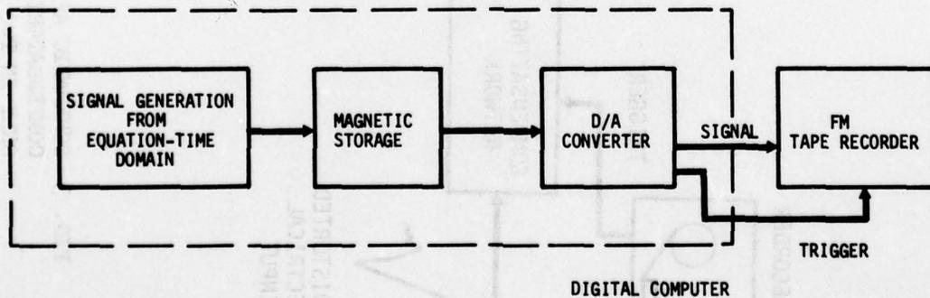
FIG. 5 FLOW CHART FOR TEST SIGNAL GENERATION WITHOUT PREDISTORTION PROCEDURE.
