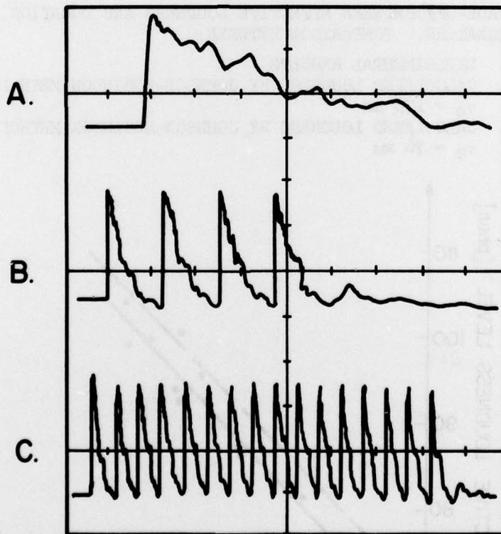
FIG. 29 REPRODUCTION OF "IDEALIZED" BLAST WAVEFORMS BY UTIAS SIMULATION BOOTH AS USED IN THE SUBJECTIVE TEST. RISE TIME = 0.22 ms, OVERPRESSURE = 1 psf (48 N/m<sup>2</sup>).
