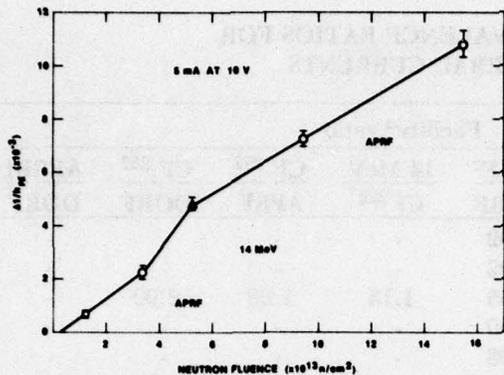
Figure 15. Damage curves of transistor type 2N2857 at fast-burst reactor (O) and 14-MeV neutron generator ( $\Delta$ ).
