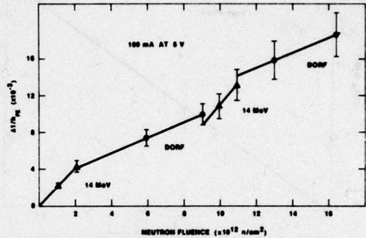
Figure 8. Damage curves of transistor type 2N5320 at TRIGA reactor (●) and 14-MeV neutron generator (Δ).
