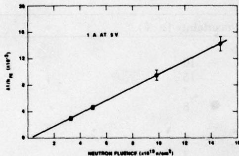
Figure 3. Damage curve of transistor type 2N3055 at Californium 252 source.
