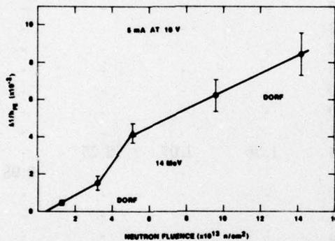
Figure 16. Damage curves of transistor type 2N2857 at TRIGA reactor ( $\bullet$ ) and 14-MeV neutron generator ( $\blacktriangle$ ).
