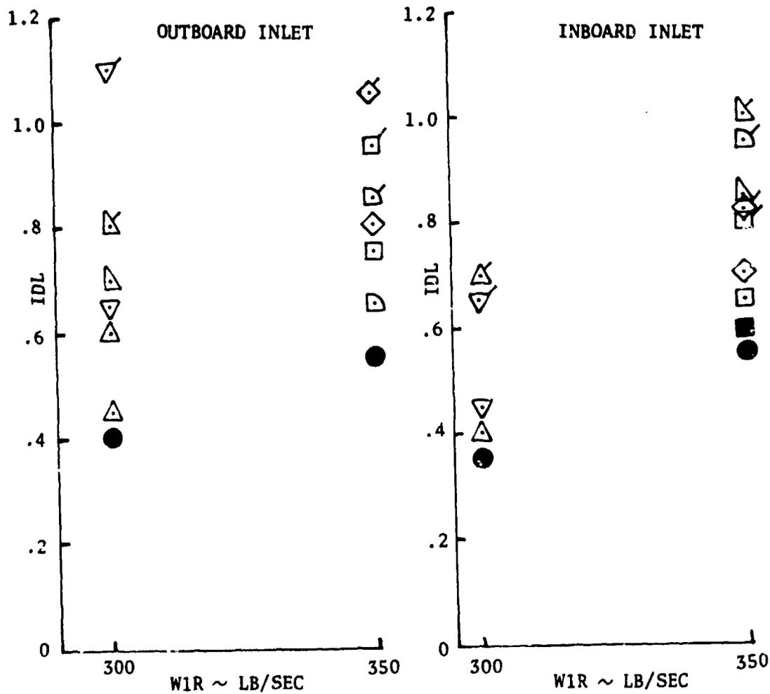
Figure 19(c) Effect of Incident Shock Upon Stall Margin Index
