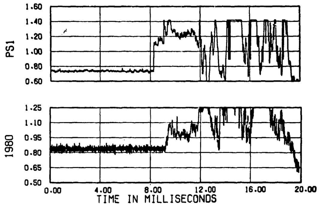
Figure 7 Comparison of Qualitative Characteristics of Claw Probe Static Pressure and Duct Static Pressure Histories For Shock Tube #2
