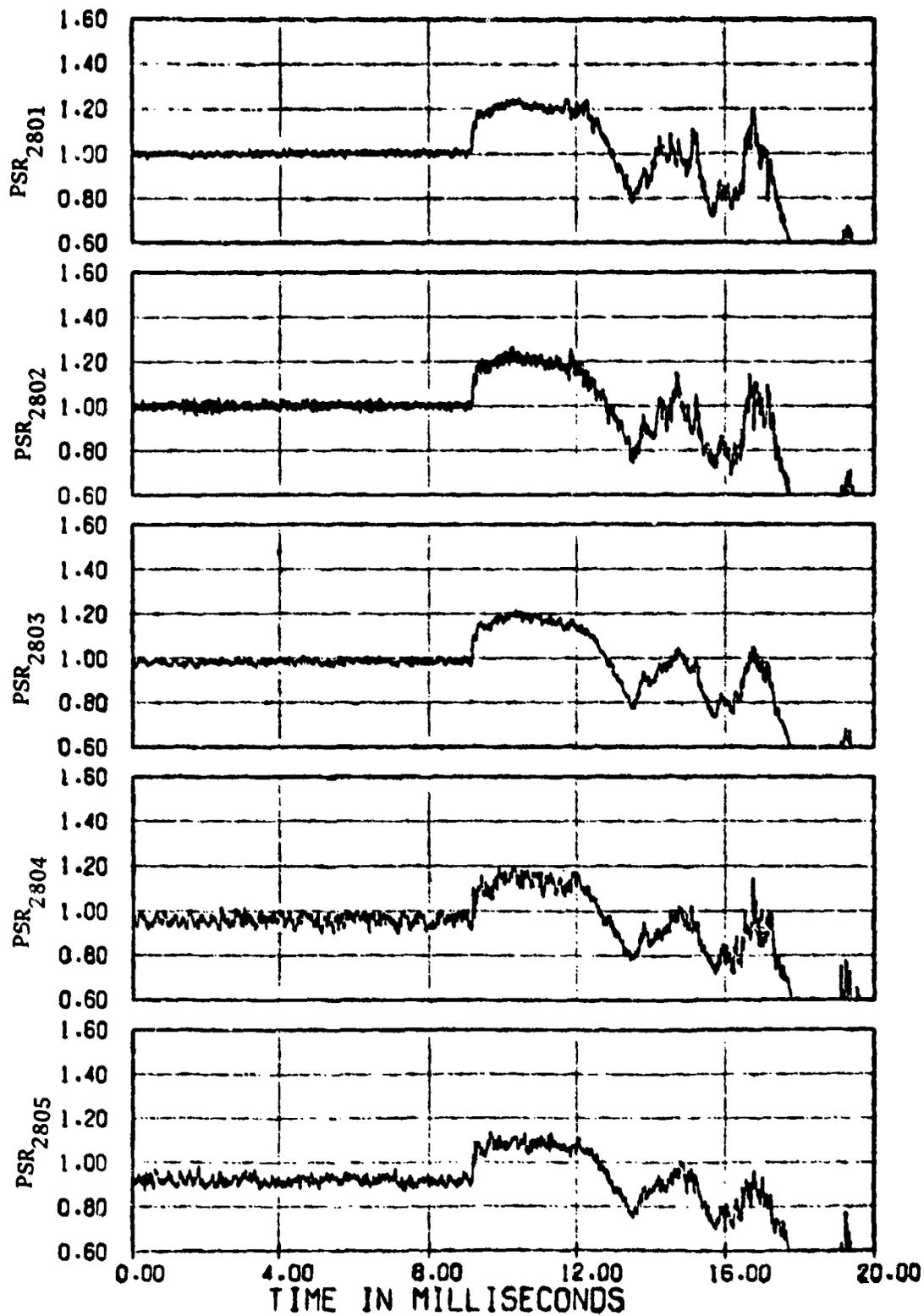
Figure 10(a) Inboard Inlet AIP Total Pressure Ratio Across the Incident Shock,  $M_0 = 0.85$  Part 546 Tube No. 1
