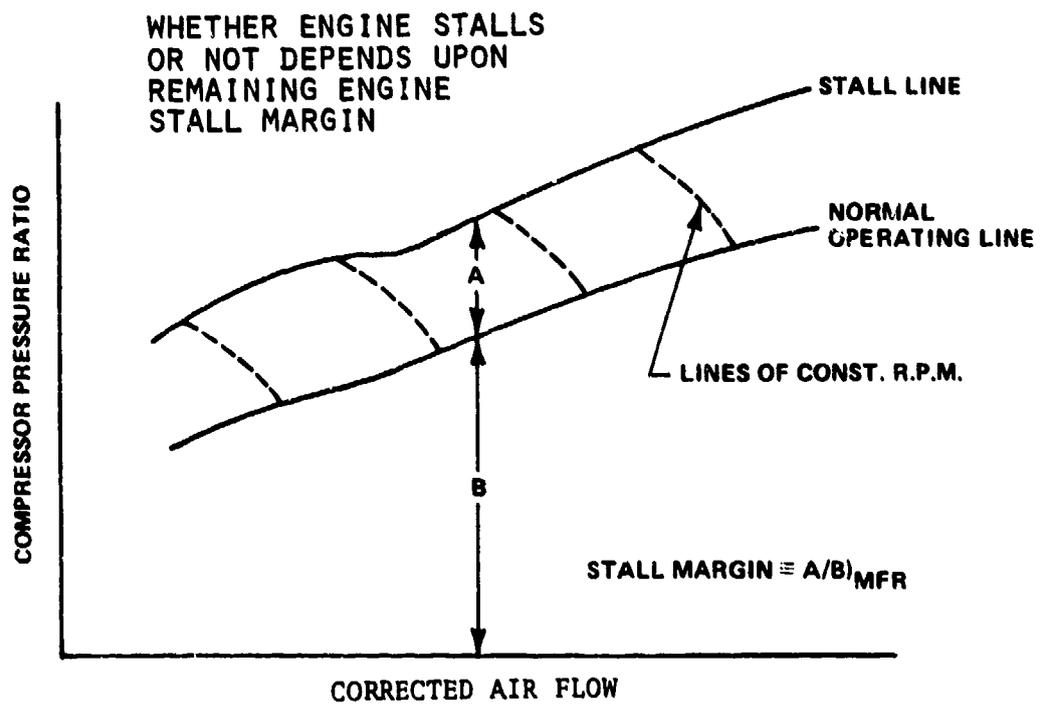
Figure 1 Typical Compressor Stall Map
