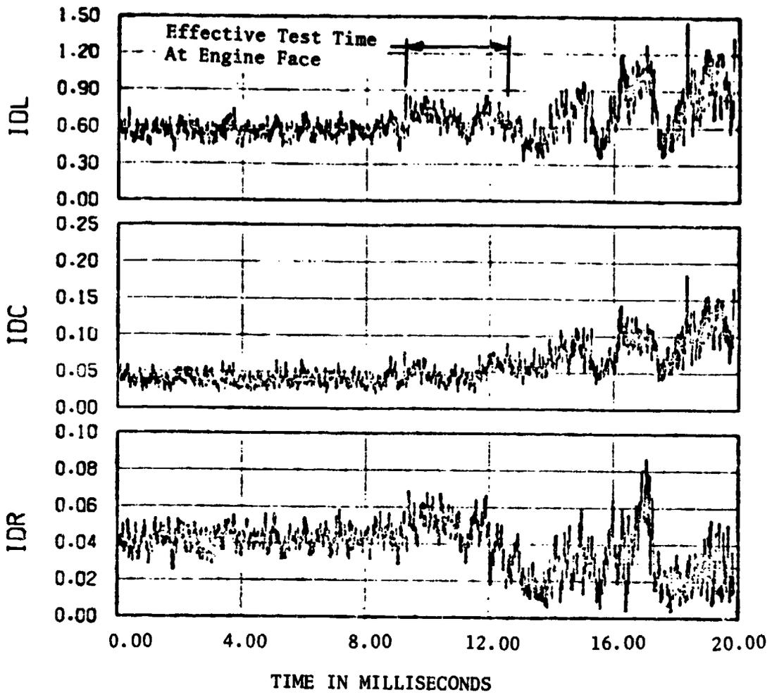
Figure 12(b) Inboard Inlet Distortion Indices,
