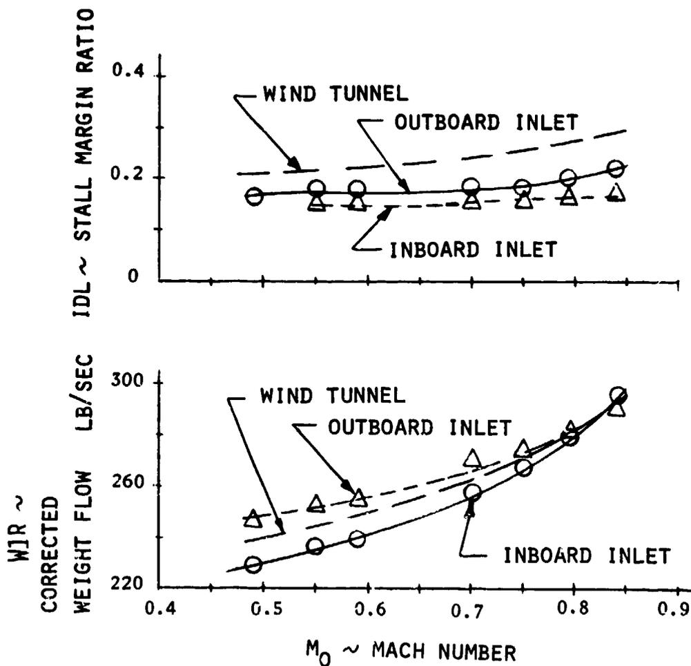
Figure 20(a) Steady-State Inlet Flight Performance
