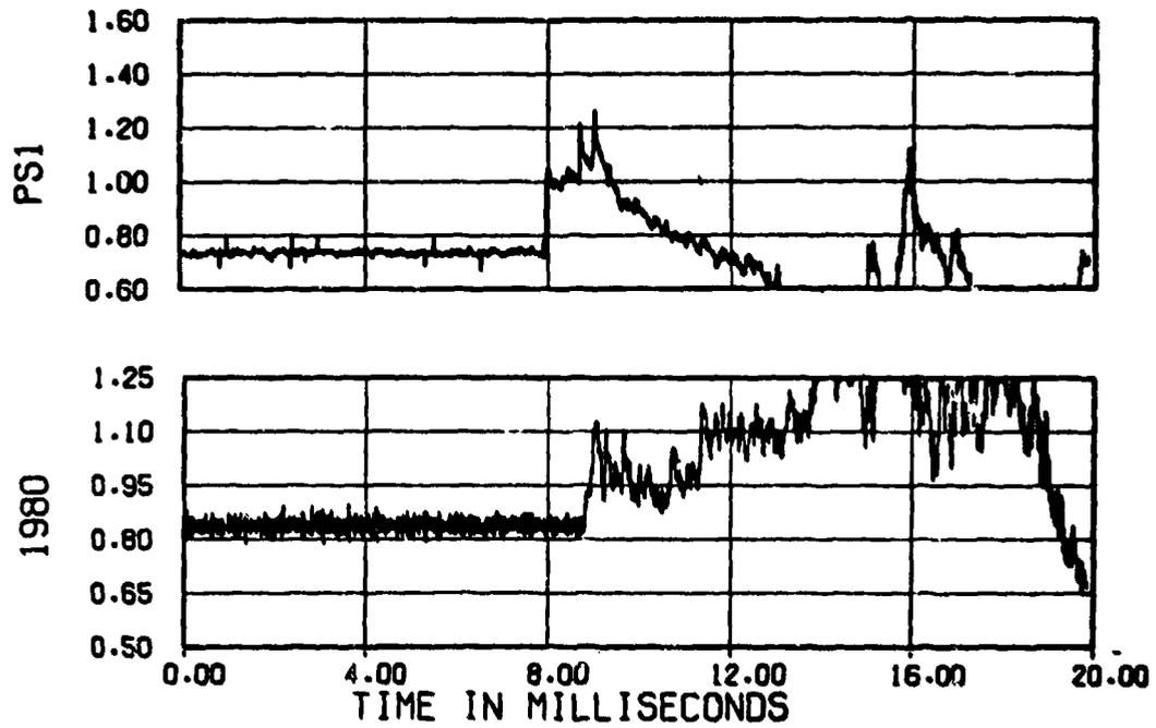
Figure 6 Comparison of Qualitative Characteristics of Claw Probe Static Pressure and Duct Static Pressure Histories For Shock Tube #1
