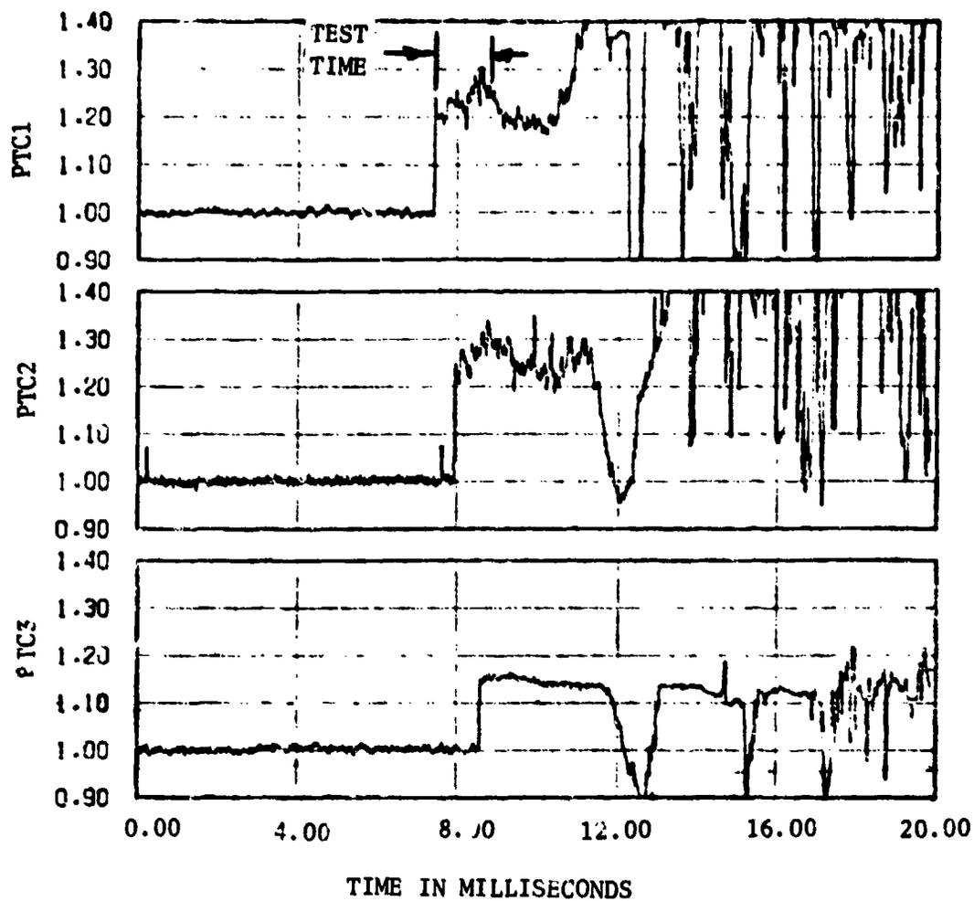
Figure 5 Claw Probe Total Pressure Ratios
