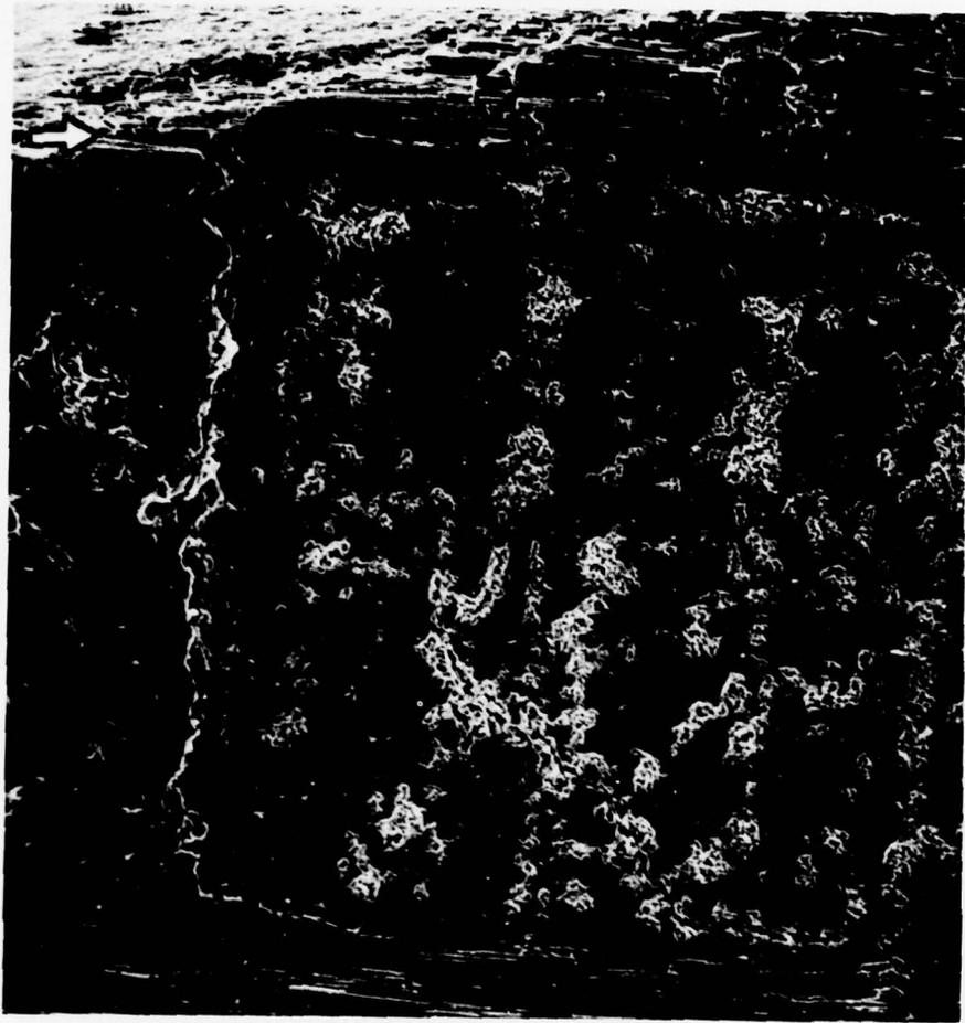
FIGURE 40. SEM PHOTOGRAPH (SPECIMEN SEM-14) SHOWING CRACK WHICH INITIATED IN SHEAR (WHITE ARROW), PROPAGATED OPENING MODE, AND FINALLY TURNED  $90^\circ$  (TO SHEAR MODE AGAIN) AND RAN ALONG FIBER BUNDLE. 120X, 73 MPa (10.5 ksi). (LOADING DIRECTION IS OUTWARD IN HORIZONTAL DIRECTION).
