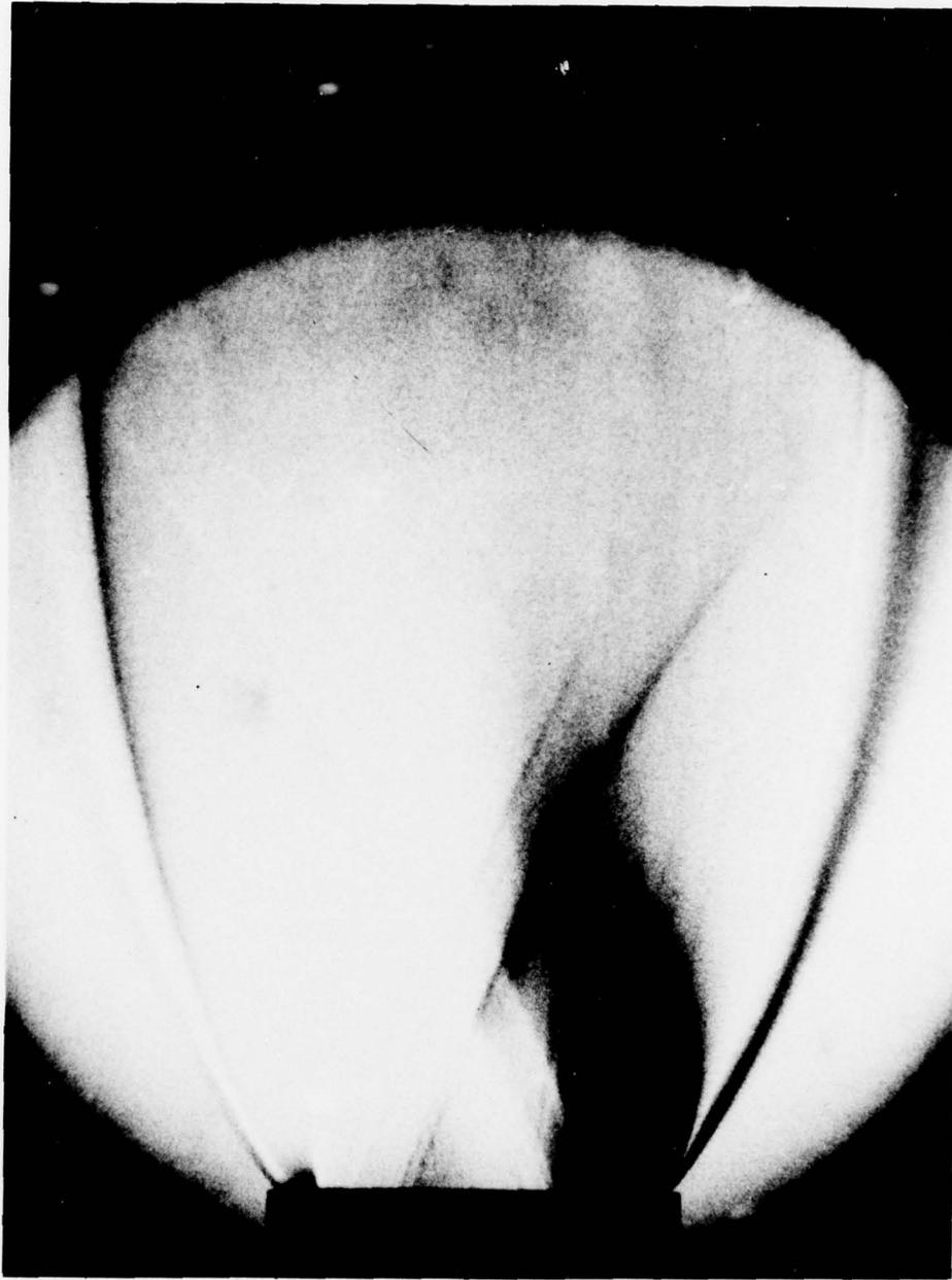
Figure 21. - The experimental plume boundary for the 10° contoured nozzle,  $P_{t1} = 8.715 \times 10^6 \text{ N/m}^2 \text{ (psia)}$
