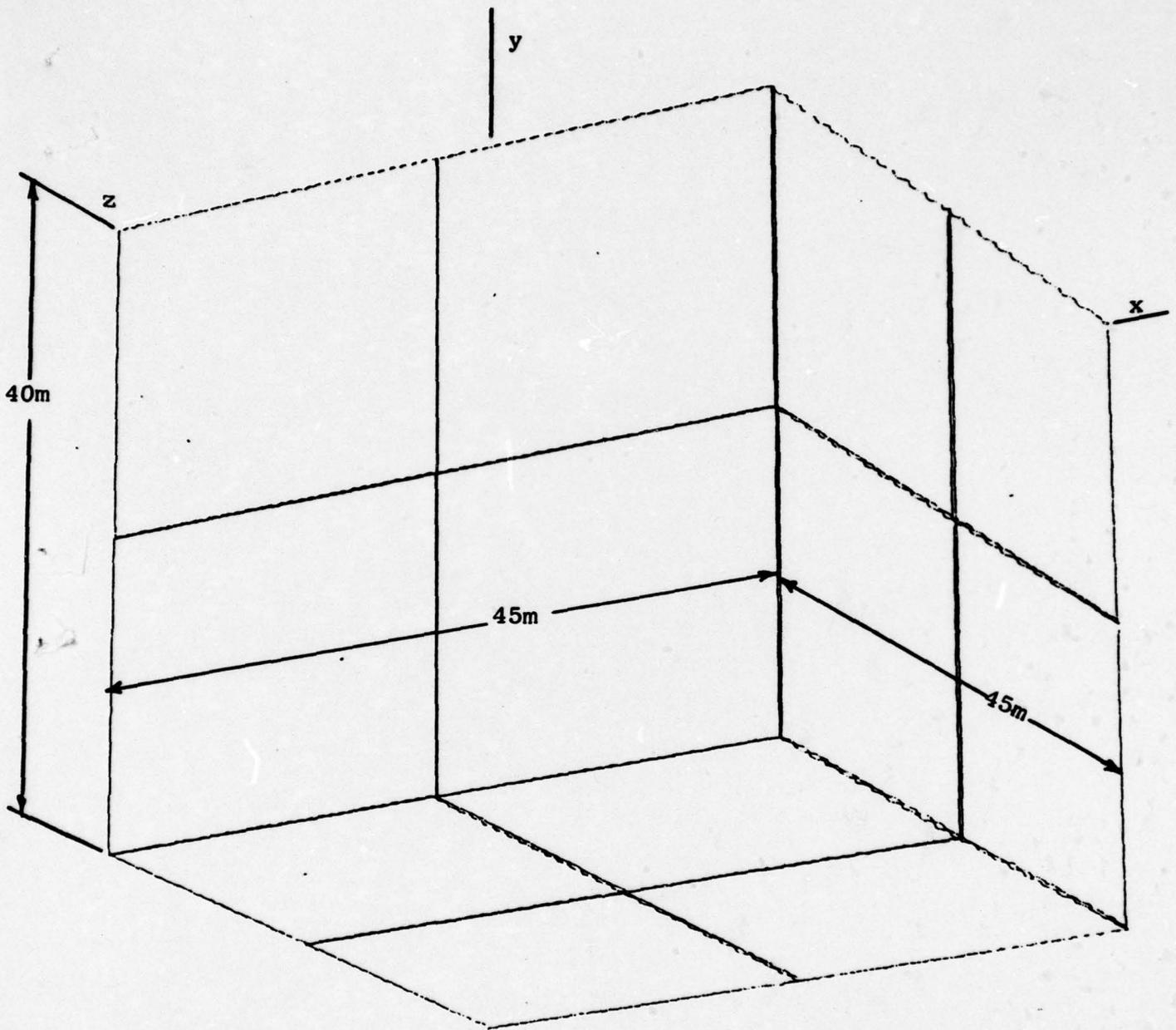
FIGURE 10: FLOATING BOX, 90M x 90M x 40M. NB=48 PANELS
