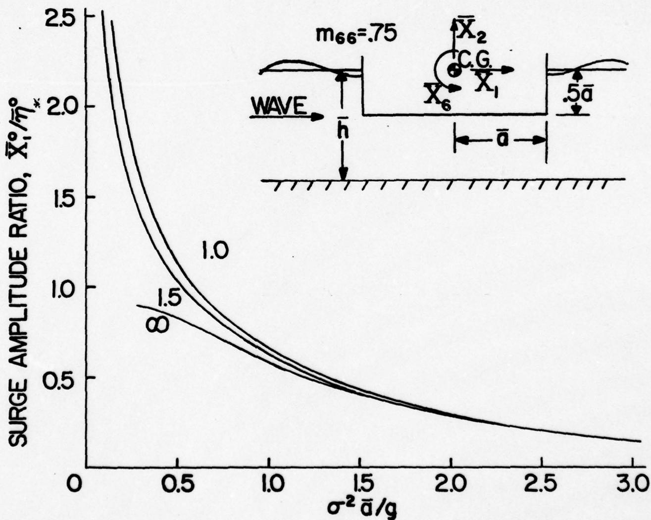
FIGURE 31 SURGE RESPONSE OF A FLOATING VERTICAL CIRCULAR CYLINDER.
