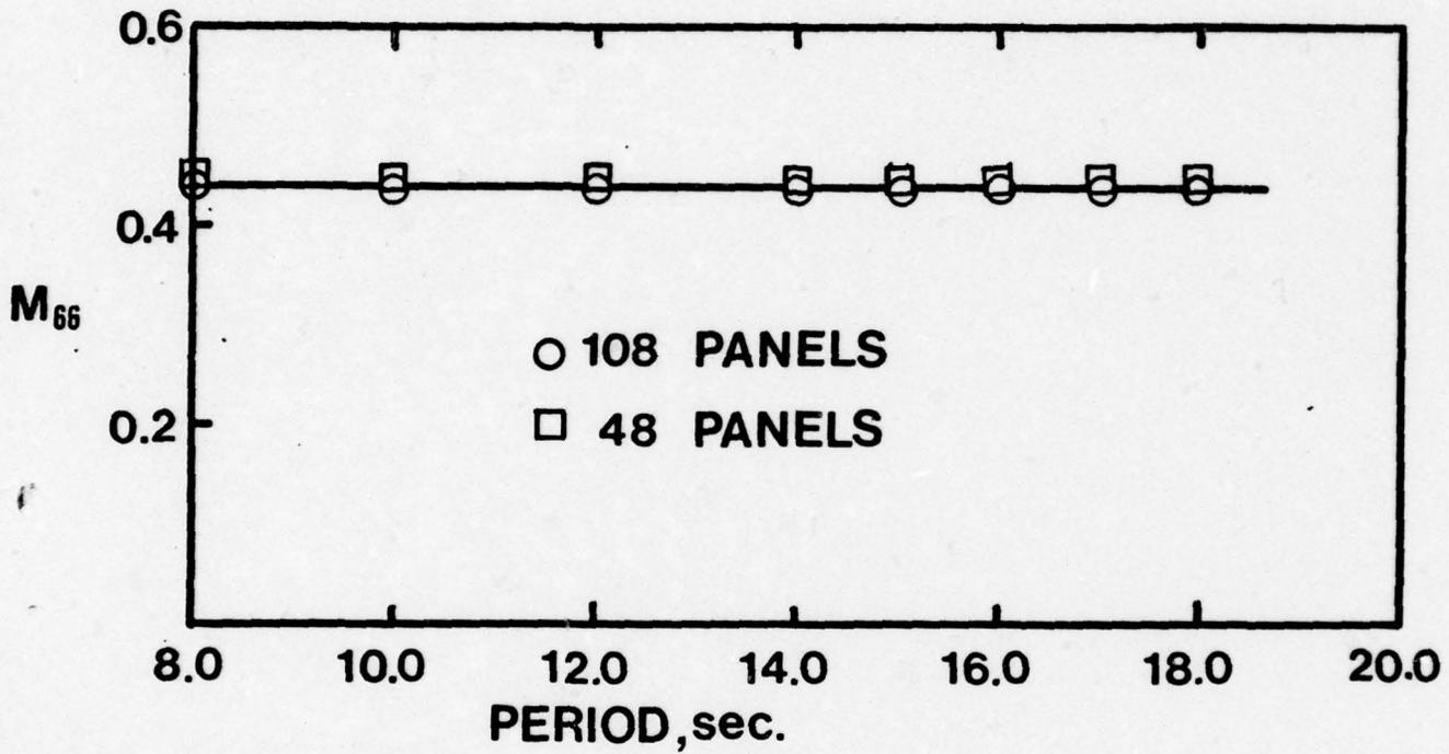
FIGURE 18 PITCH ADDED MOMENT OF INERTIA COEFFICIENT
