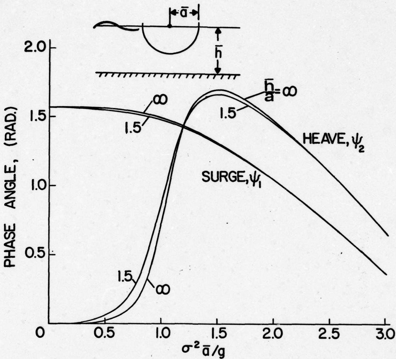
FIGURE 28 PHASE SHIFT ANGLES OF THE HEAVE AND SURGE RESPONSE OF SEMI-SUBMERGER SPHERE.
