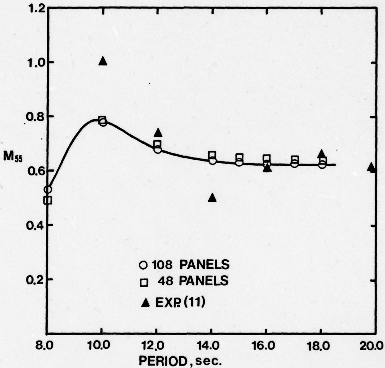
FIGURE 19 YAW ADDED MASS COEFFICIENT
