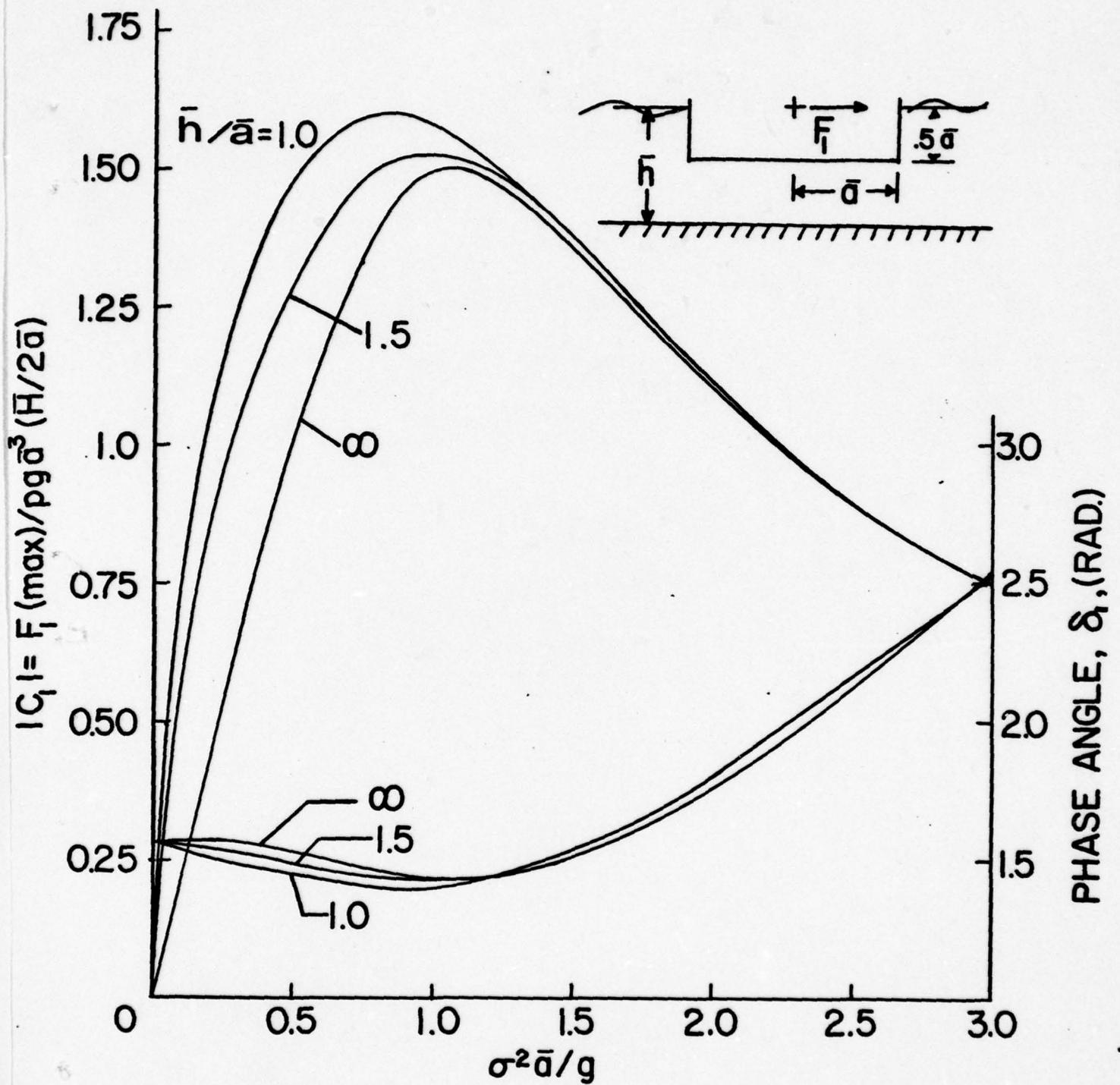
FIGURE 30 HORIZONTAL FORCE COEFFICIENT FOR A FLOATING VERTICAL CIRCULAR CYLINDER.
