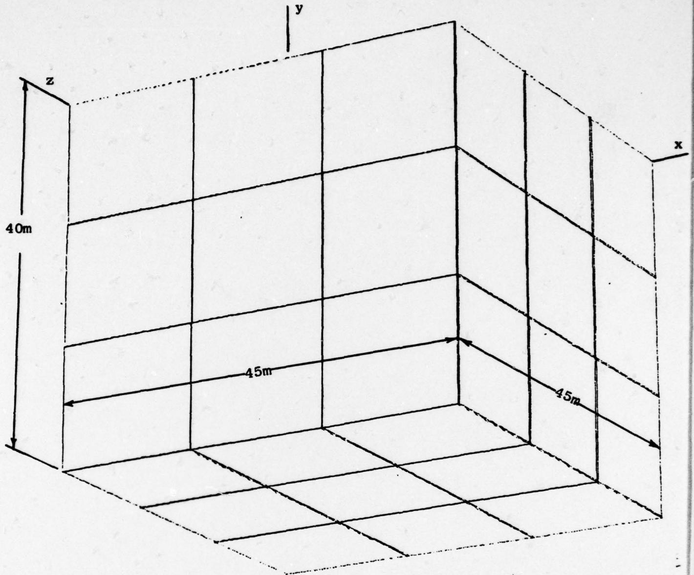
FIGURE 11: FLOATING BOX, 90M x 90M x 40M. NB=108 PANELS
