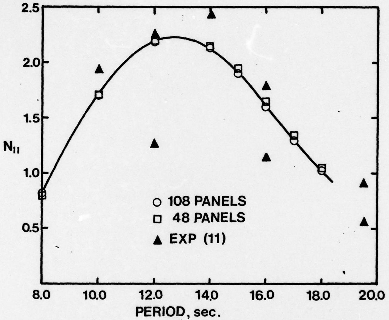
FIGURE 15 SURGE DAMPING COEFFICIENT
