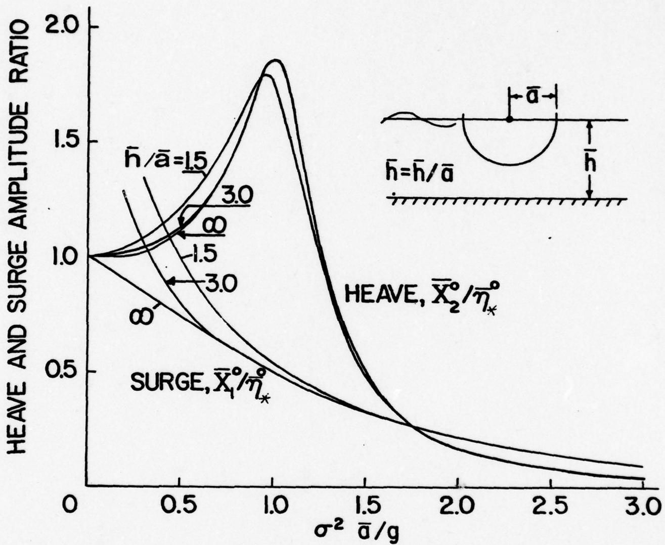
FIGURE 27 HEAVE AND SURGE RESPONSE OF A SEMI-SUBMERGED SPHERE.
