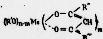
3. The method in section 1 is distinguished by the fact that the chelate compounds of metals are used in a solution of silane with the general formula  $(R'''O)_4Si$ , where  $R'''$  - alkyl with the carbon atom number from 1 to 5, in the ratio of 2:1-1:5.
