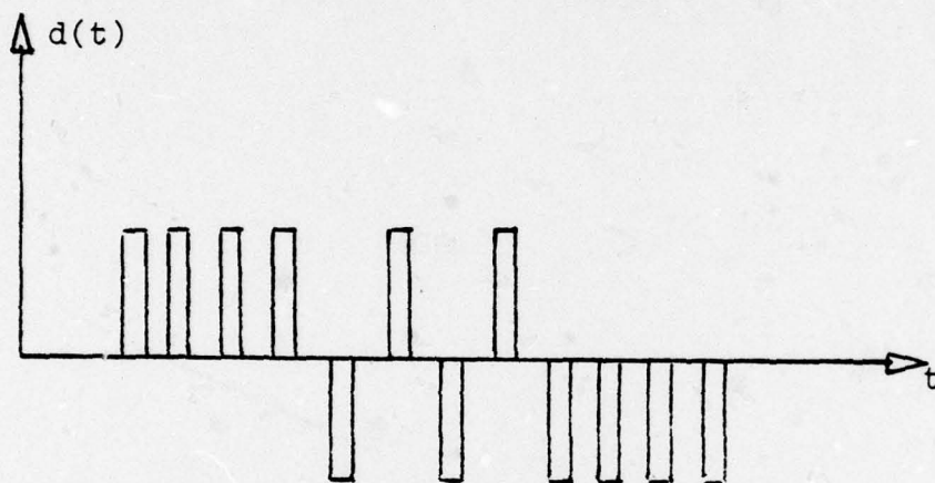
b) Output of Delta Modulator
