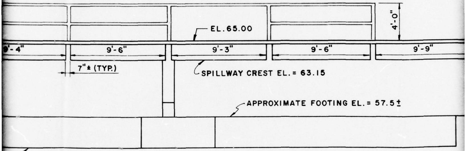
FIXED CONCRETE WEIR SPILLWAY
