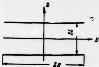
Fig. 1. Open resonator, formed by disks.
