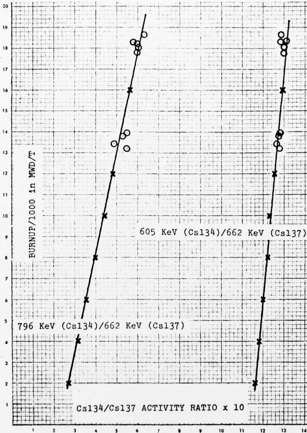
Fig. 3. Burnup Versus Cs134/Cs137 Activity Ratio at 0.42 Years Cooling Time for Different Gamma Lines of Cs134
