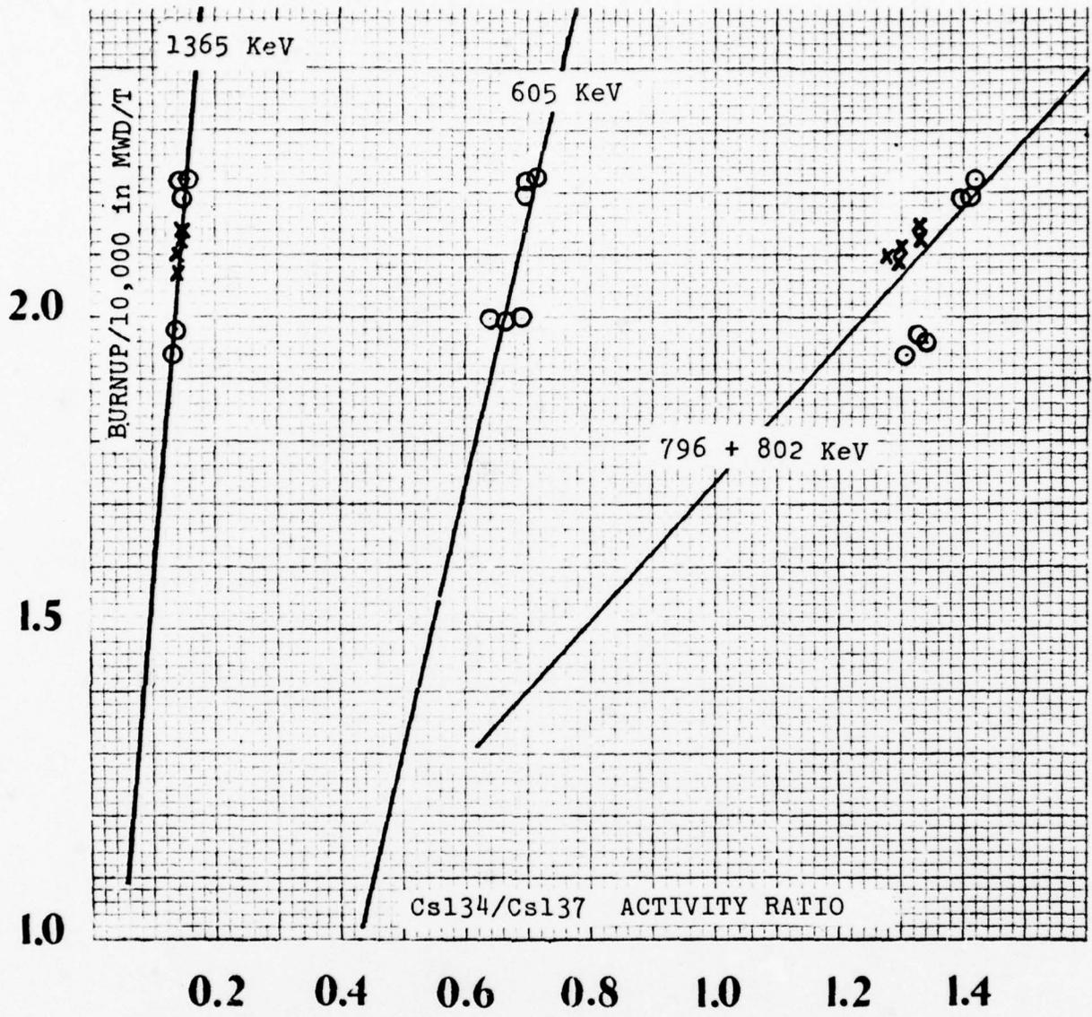
Fig. 5. Burnup Versus Cs134/Cs137 Activity Ratio for different Gamma Lines of Cs134
