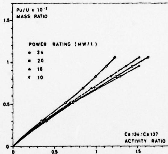
Fig. 7. Influence of the Power Rating on the Correlation between Cs134/Cs137 and Pu/U (Ref. 26:619)
