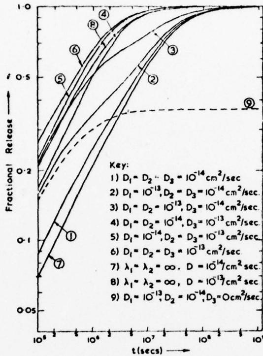
Fractional release vs time for the final stable isotope (3) in the chain:
