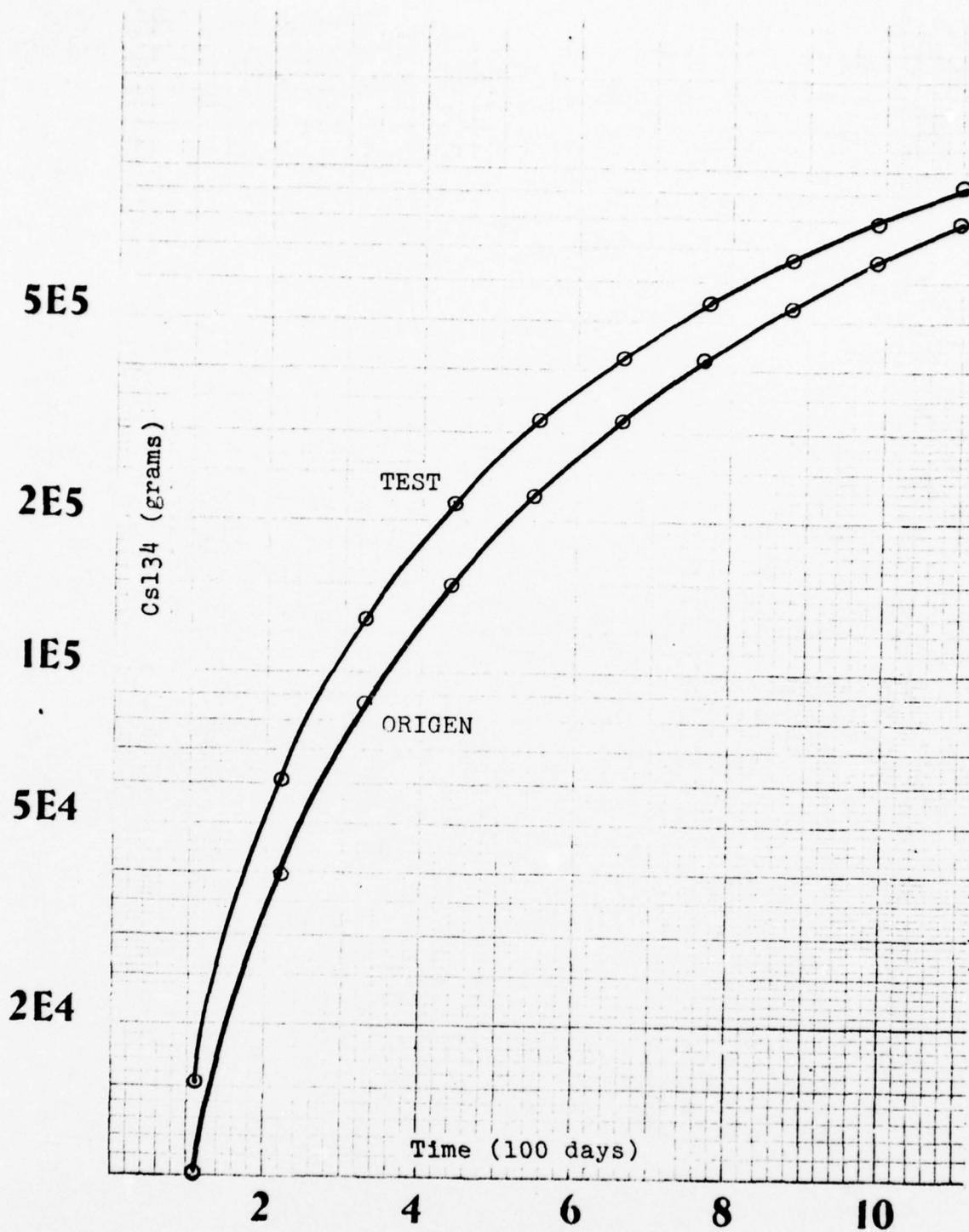
Fig. 12. Cs134 Buildup Versus Time for Codes TEST and ORIGIN
