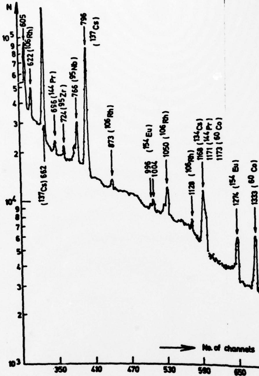
Fig. 2. Partial Gamma Spectrum for Vak Fuel Assembly (Ref. 20:34)
