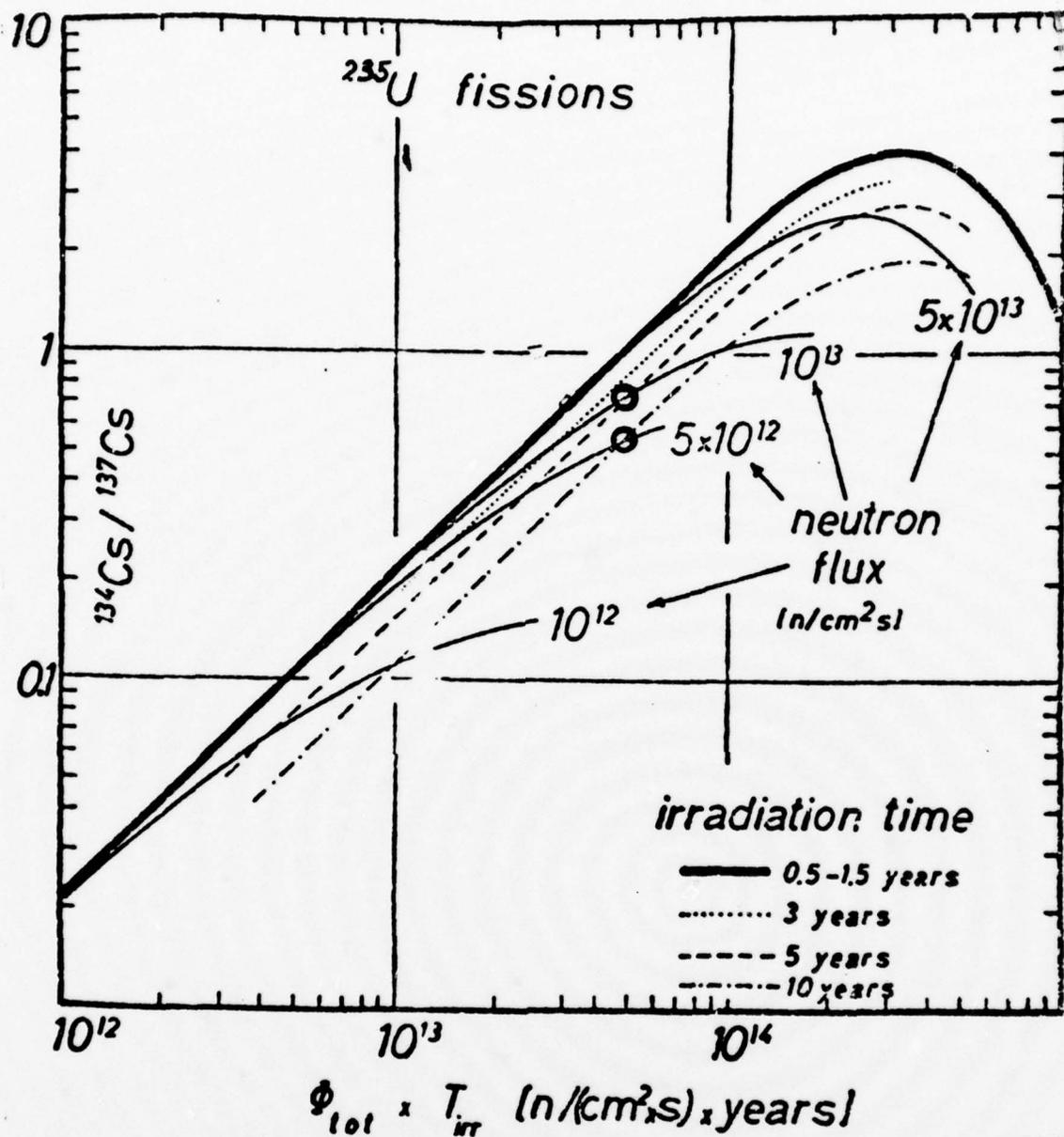
Fig. 1. Cs134/Cs137 Activity Ratio at Shutdown Versus Integrated Neutron Flux for Different values of Neutron Flux and Irradiation Time (Ref. 15:241)
