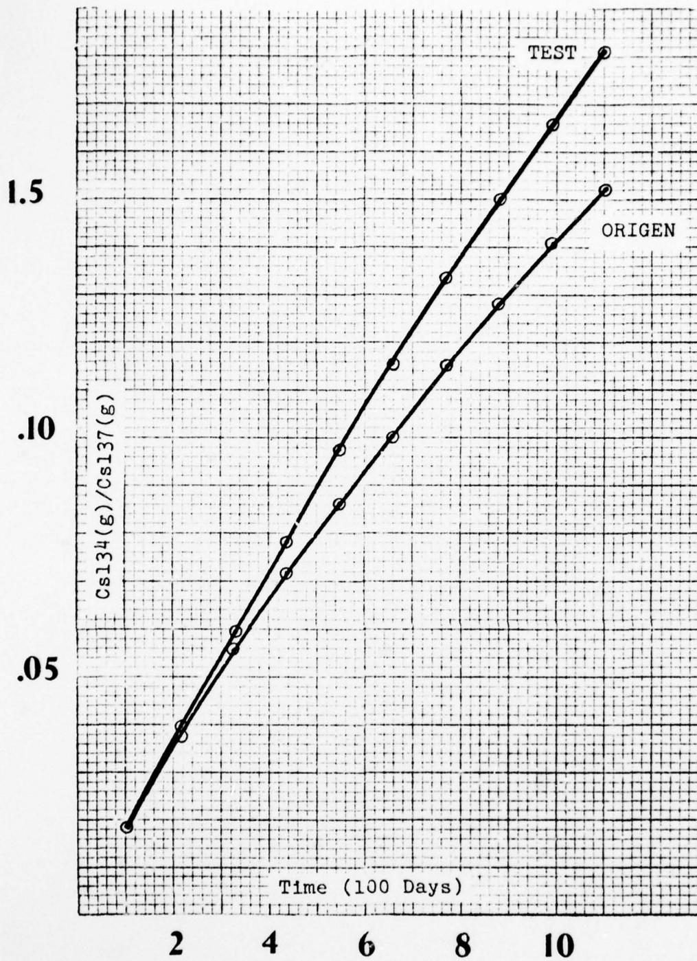
Fig. 14. Cs134/Cs137 Versus Time for Codes TEST and ORIGIN
