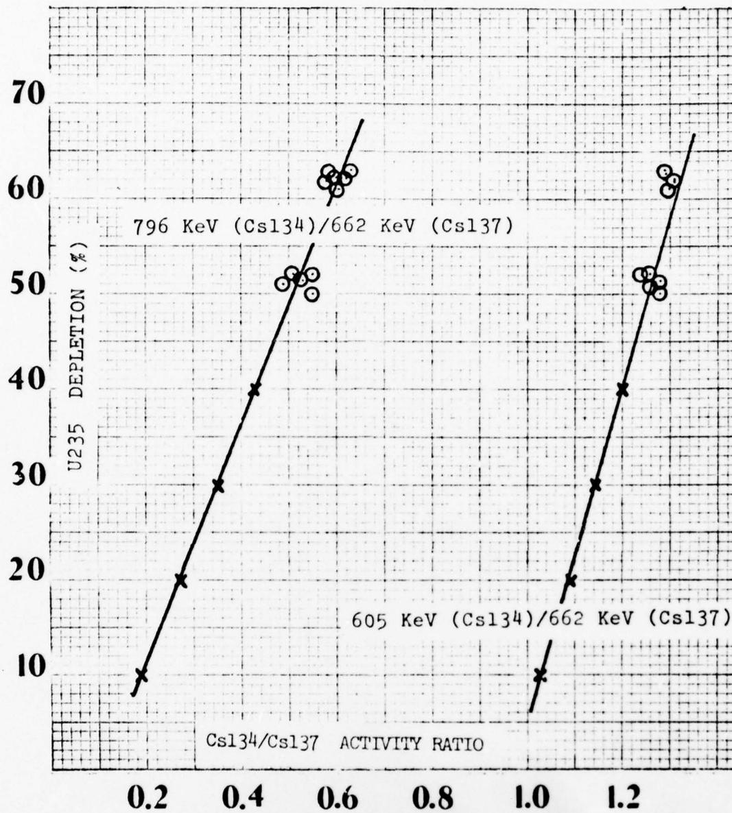
Fig. 4. U235 depletion versus Cs134/Cs137 activity ratio at 0.42 years cooling time for different gamma lines of Cs134
