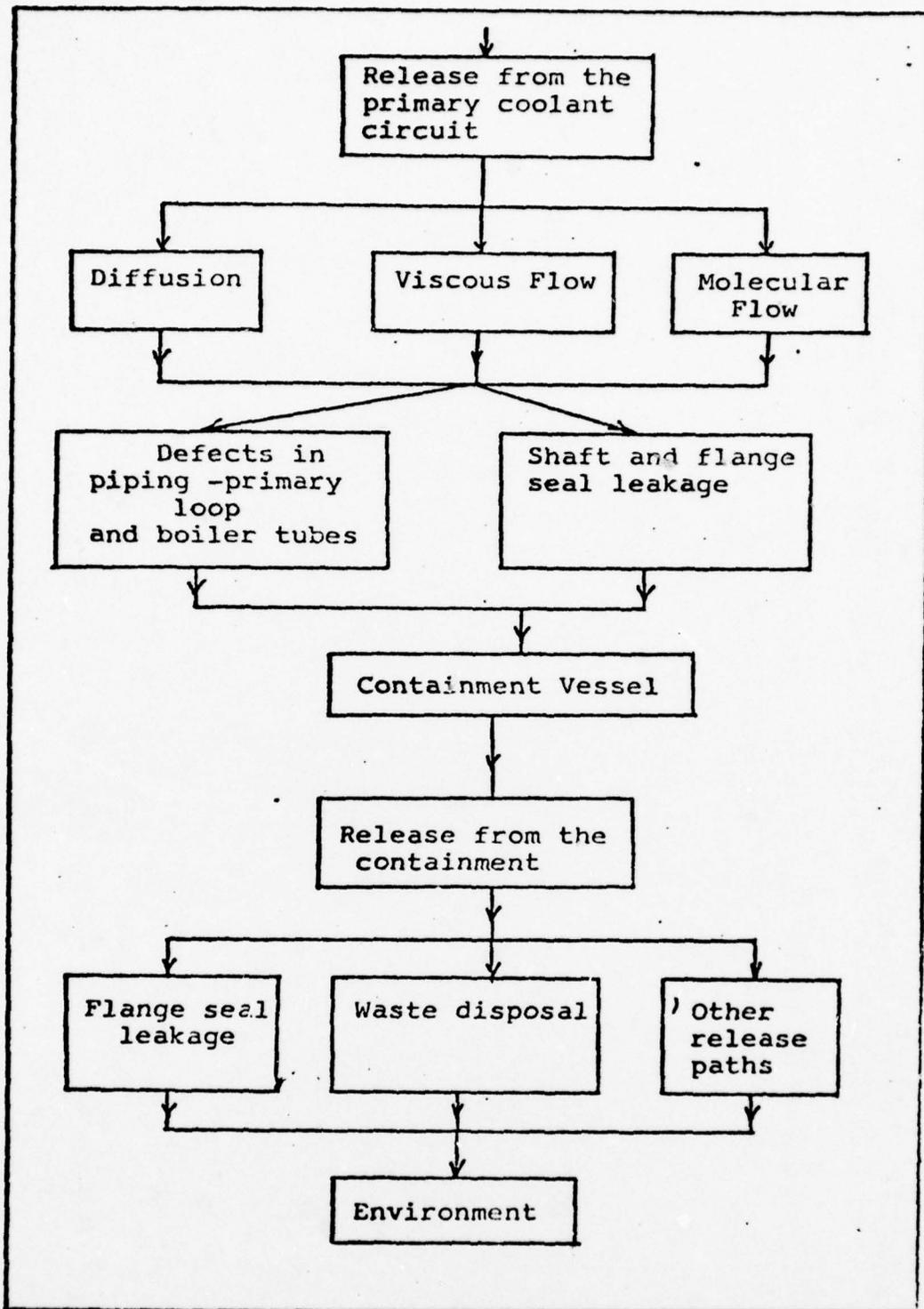
Fig. 17. Fission Product Escape Mechanisms for Primary Coolant to Environment (Ref. 32:6)
