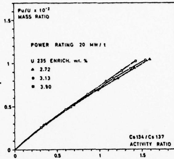
Fig. 6. Influence of the Fuel Enrichment on the Correlation Between Cs134/Cs137 and Pu/U (Ref 26:618)
