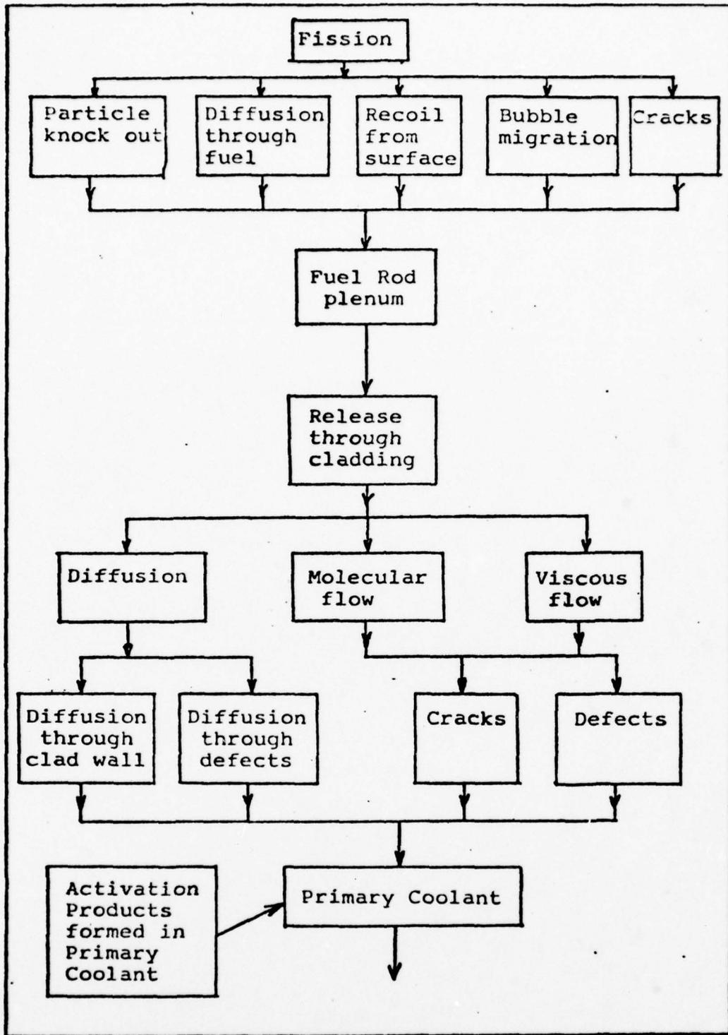
Fig. 15. Fission Product Escape Mechanisms for Fuel Matrix to Primary Coolant (Ref. 32:5)
