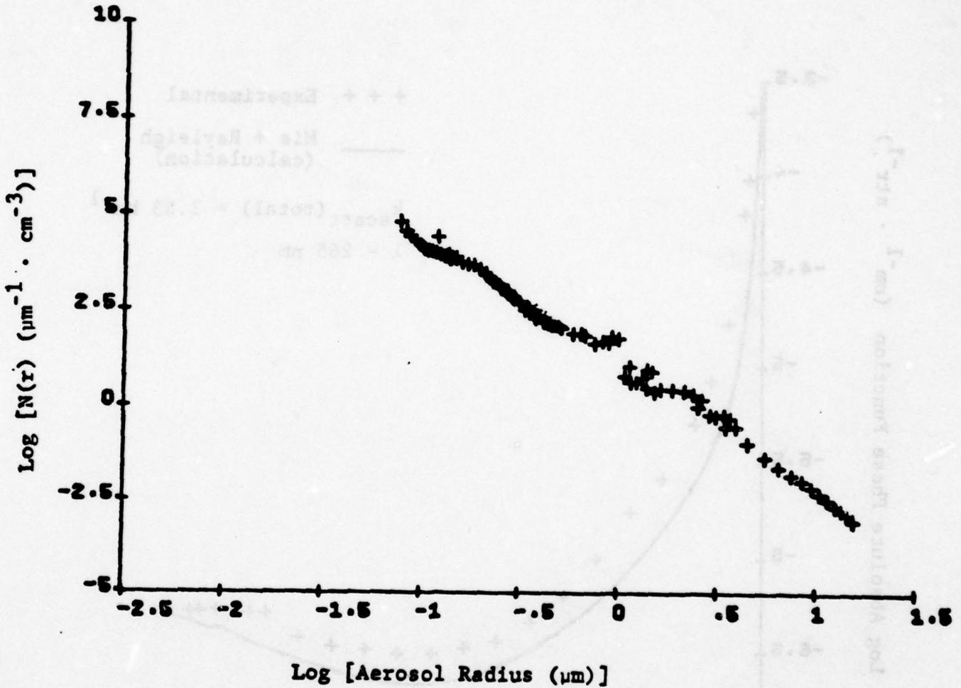
Particle size distribution for phase function measured
