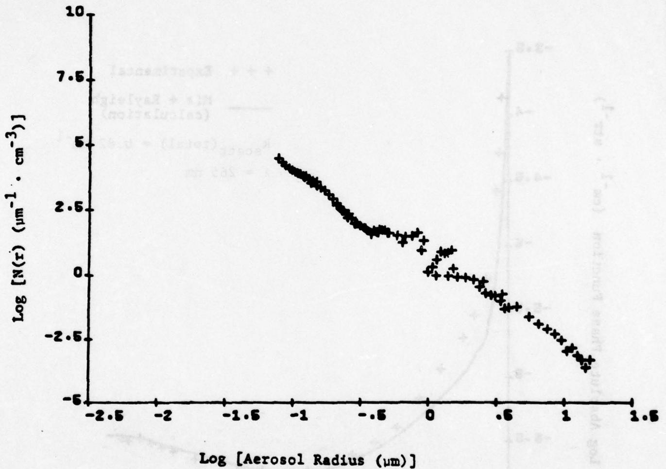
Particle size distribution for phase function measured
