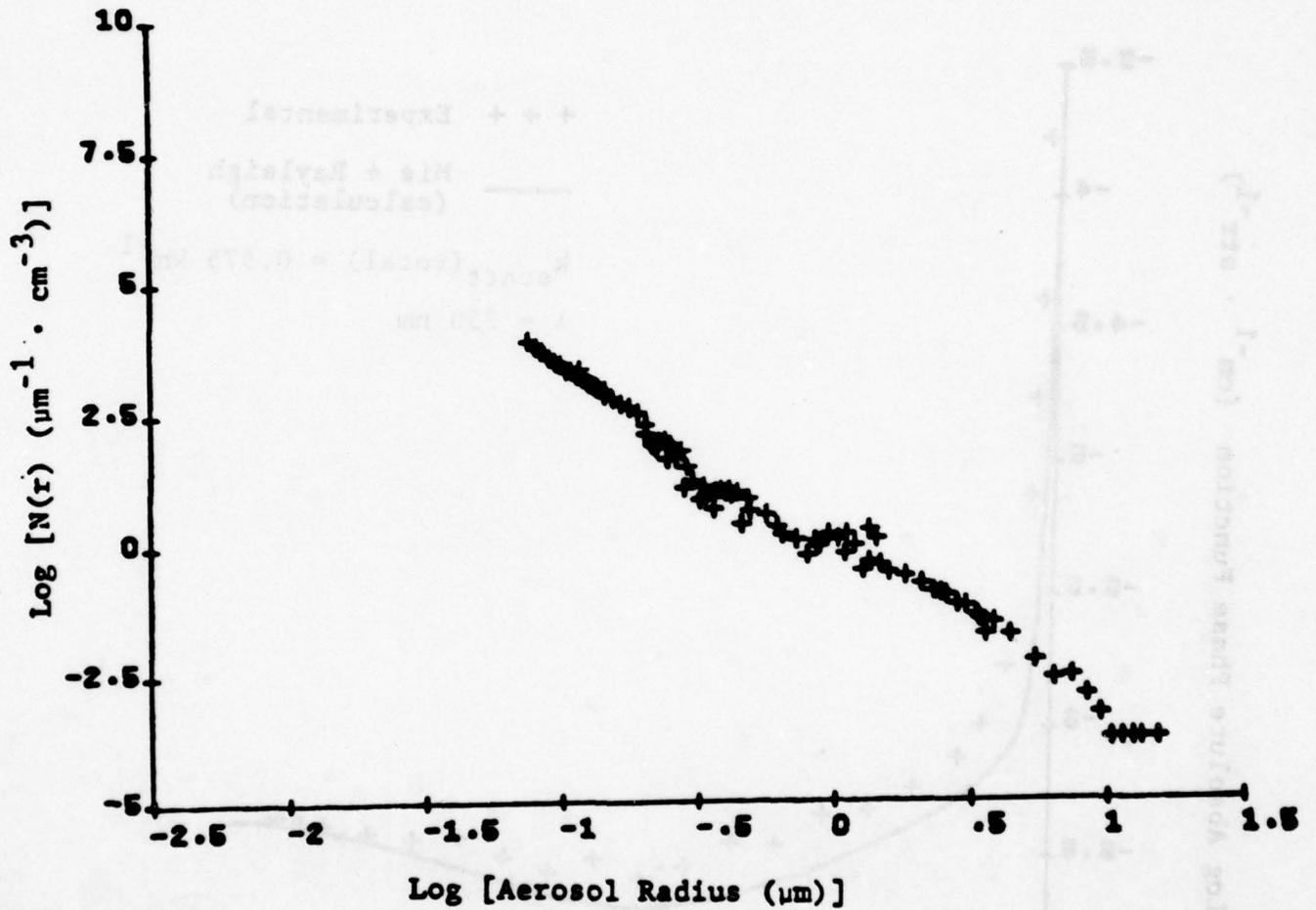
Particle size distribution for phase function measured
