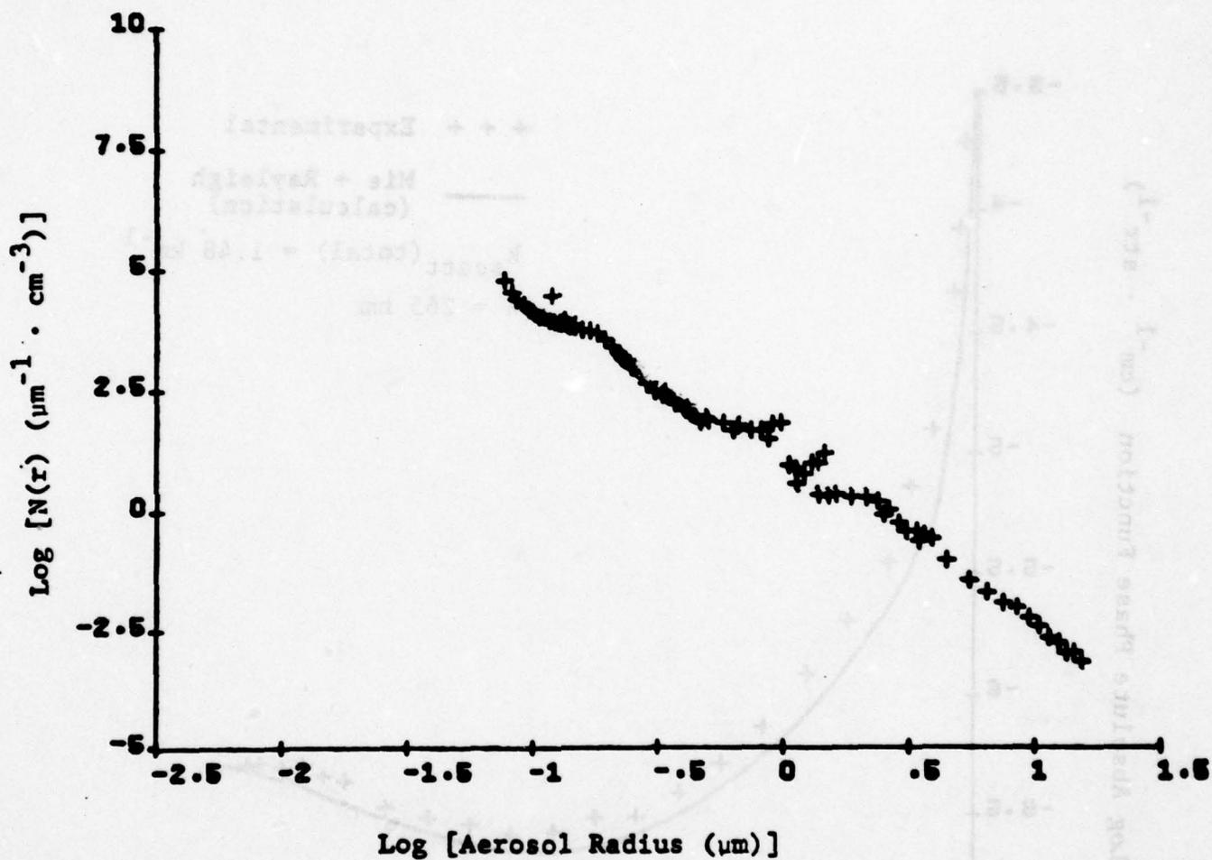
Particle size distribution for phase function measured
