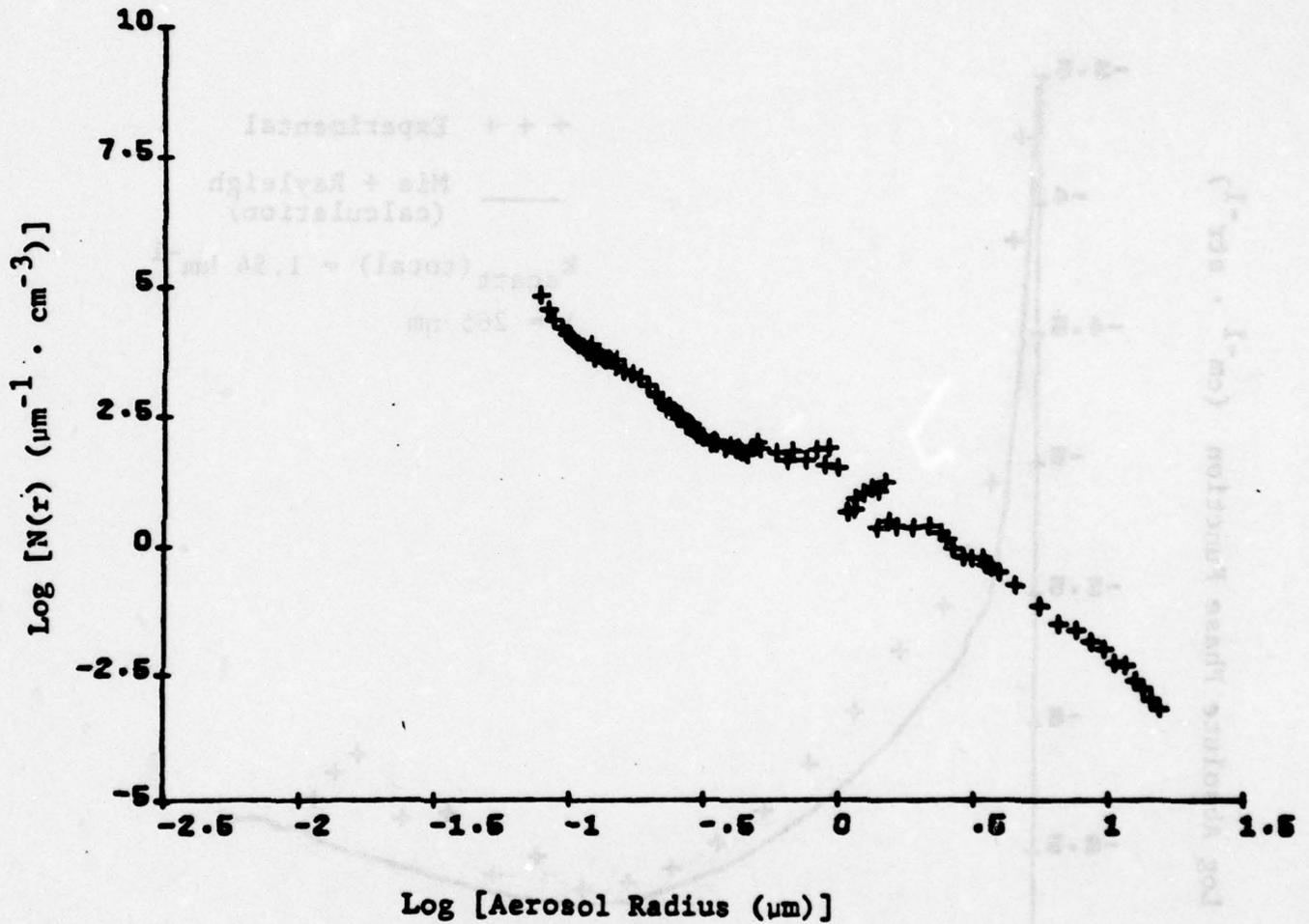
Particle size distribution for phase function measured
