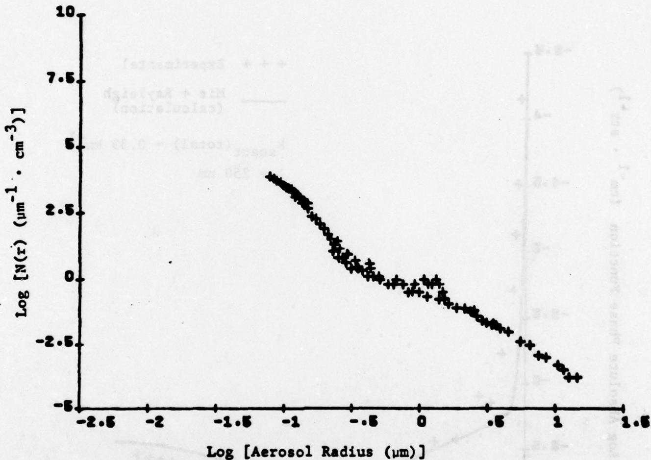
Particle size distribution for phase function measured
