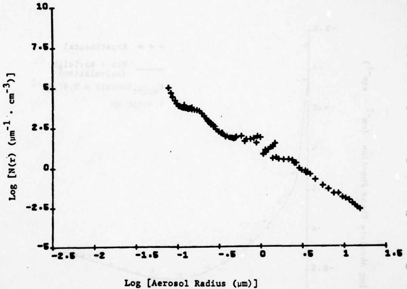
Particle size distribution for phase function measured
