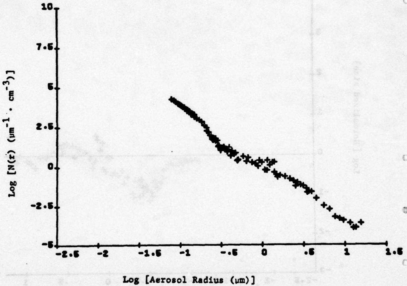
Particle size distribution measured at 2:20 p.m. on
