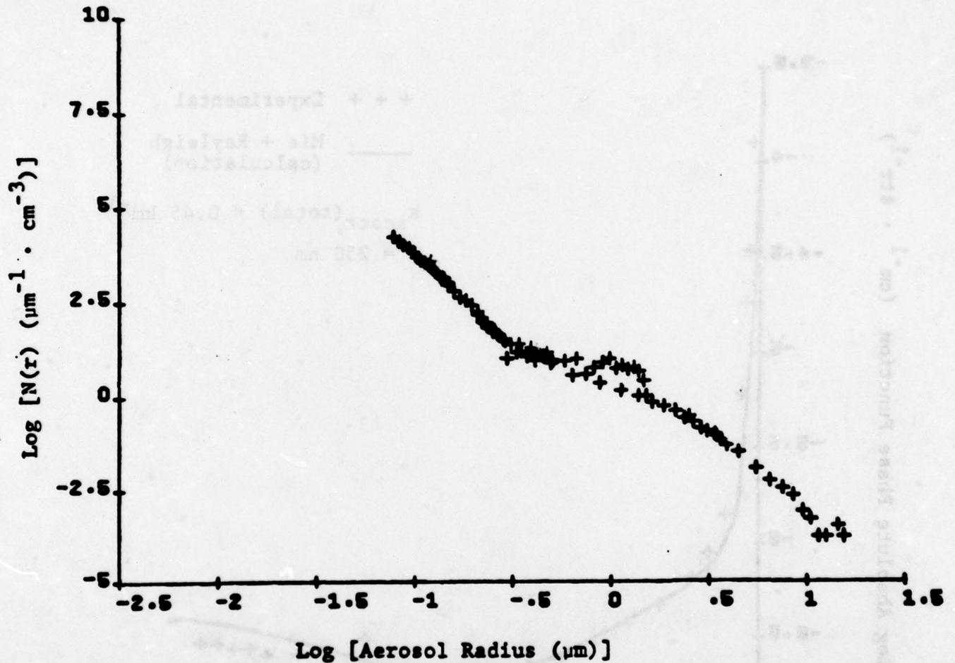
Particle size distribution for phase function measured
