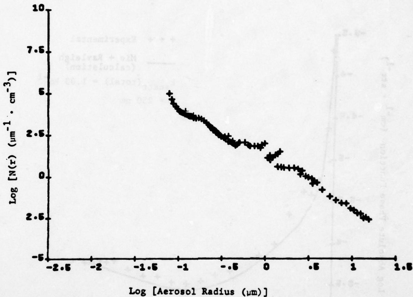
Particle size distribution for phase function measured
