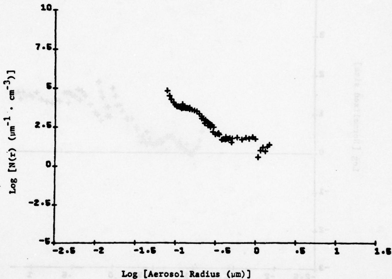
Particle size distribution for phase function measured
