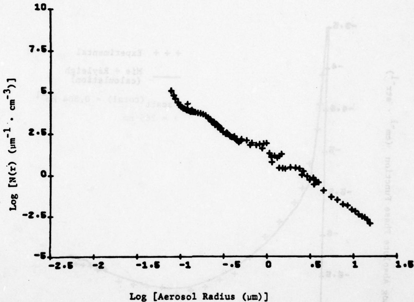
Particle size distribution for phase function measured
