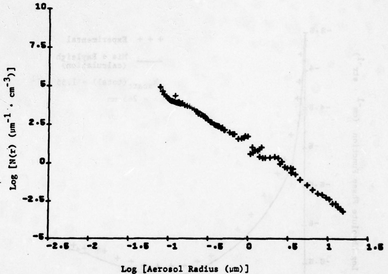
Particle size distribution for phase function measured
