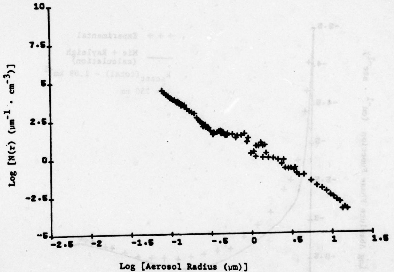
Particle size distribution for phase function measured
