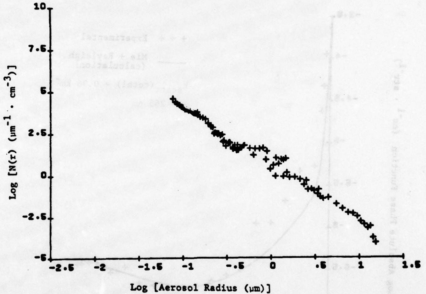
Particle size distribution for phase function measured
