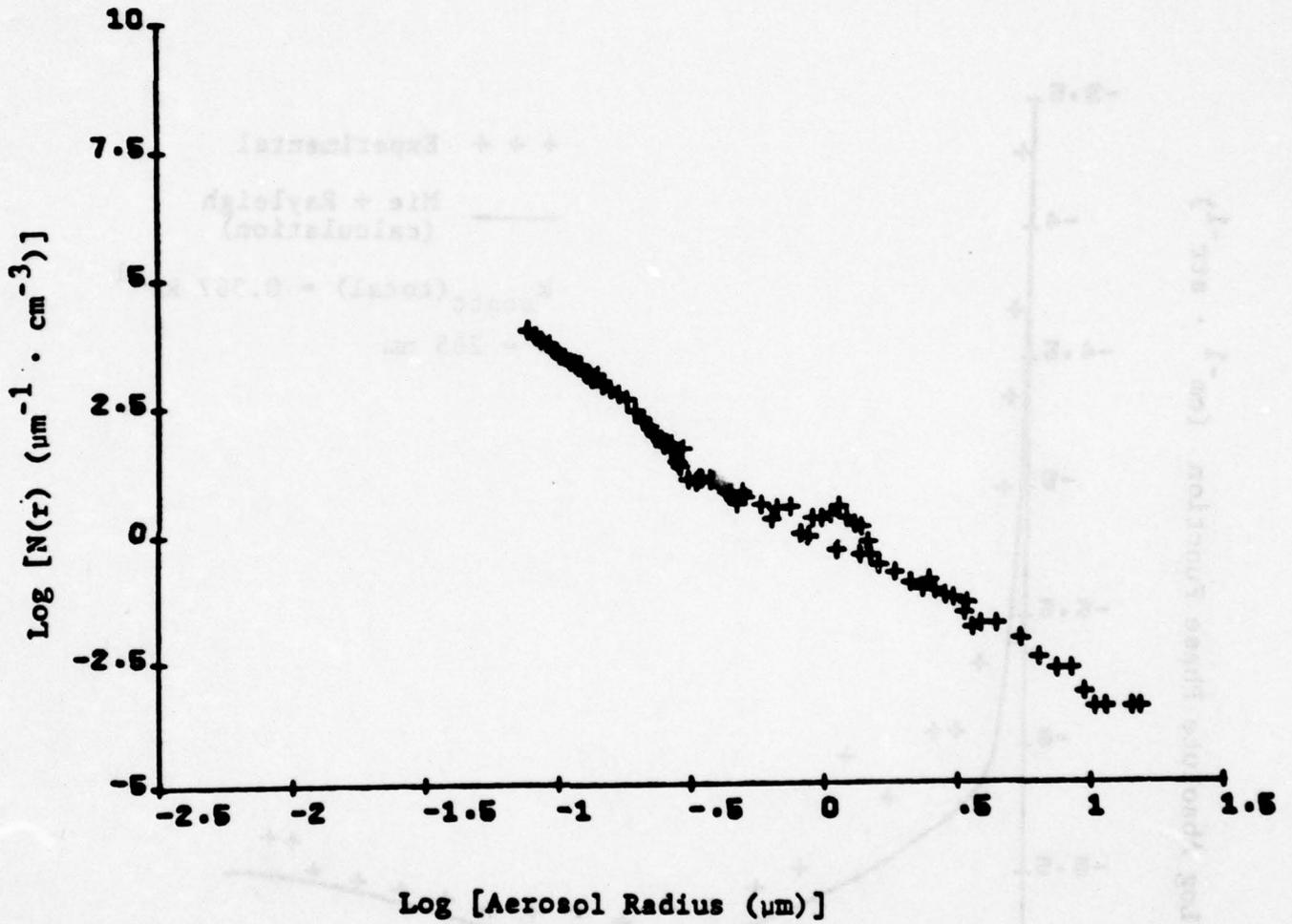
Particle size distribution for phase function measured at 8:25 p.m. on October 18, 1978.
