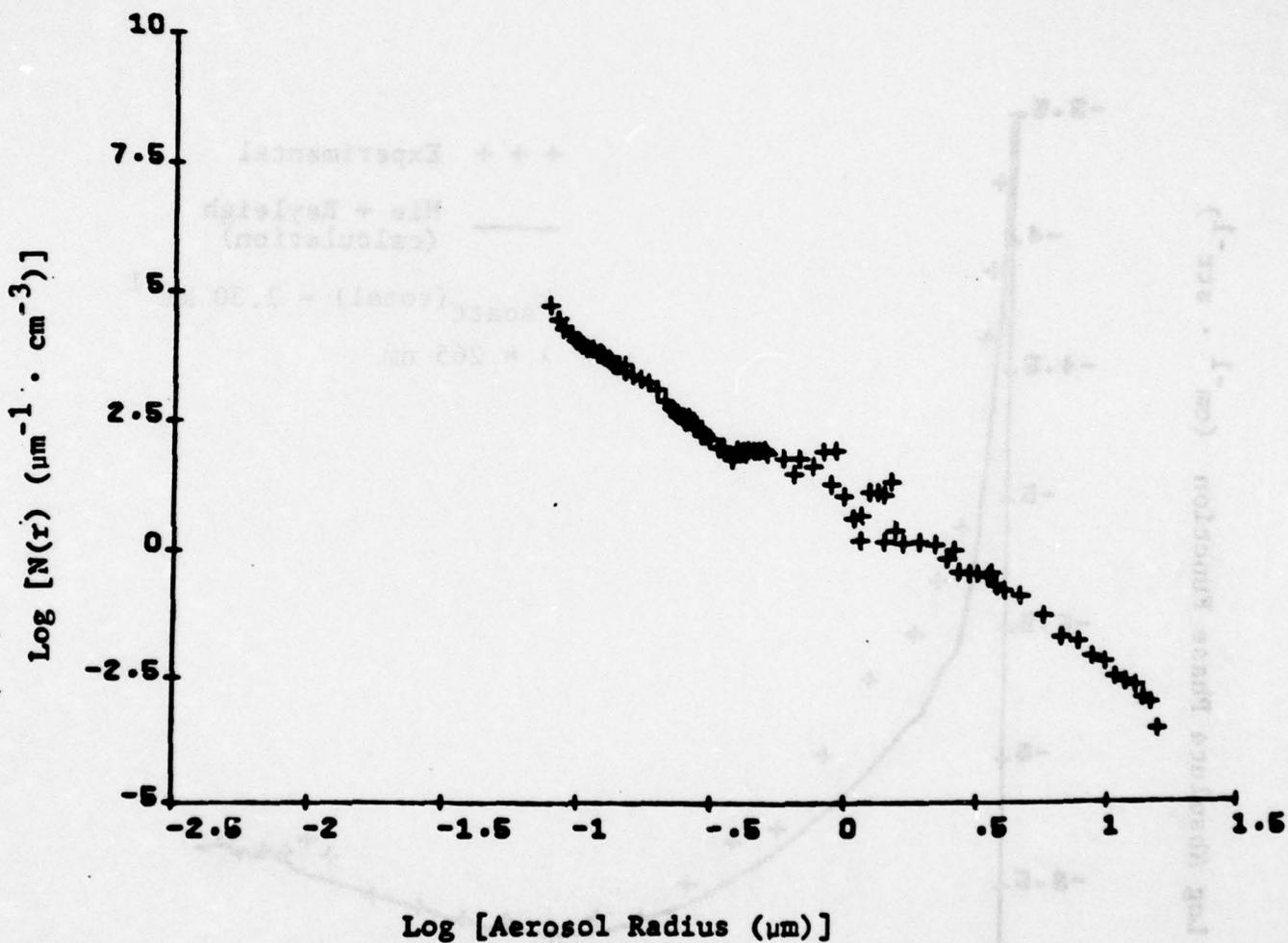
Particle size distribution for phase function measured
