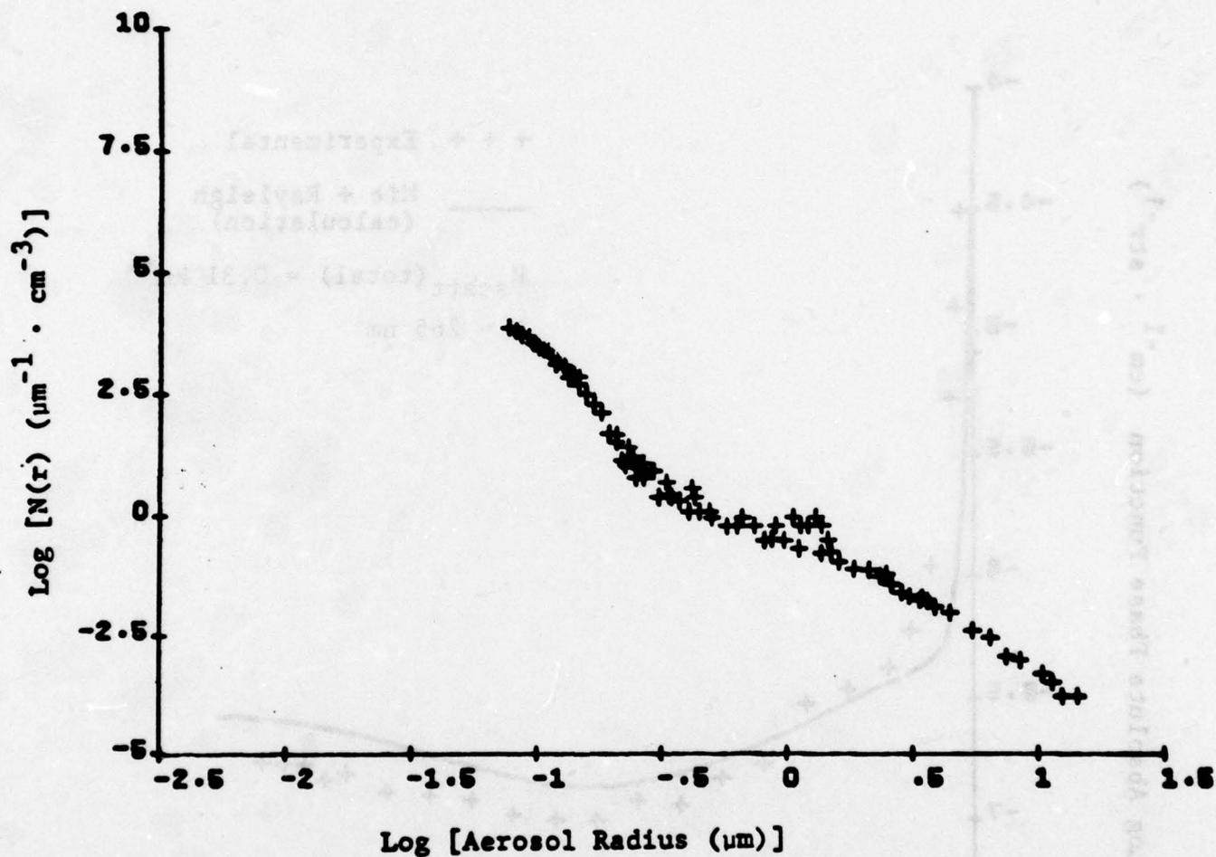
Particle size distribution for phase function measured
