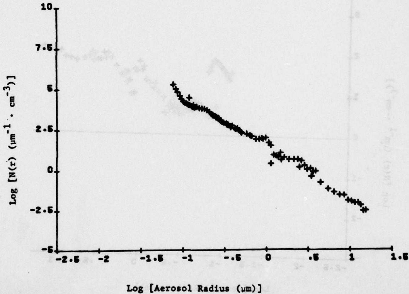
Particle size distribution for the phase function measured at 8:25 a.m. on October 13, 1978.
