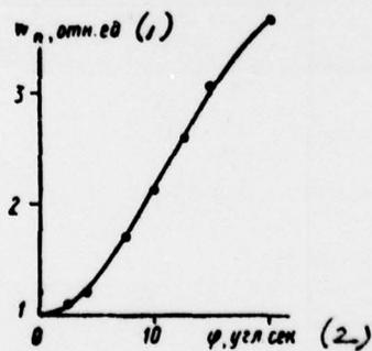
Fig. 4. Dependence of threshold pumping  $w_n$  on the angle of misalignment of the mirrors  $\phi^\circ$ . KEY: (1) relative units, (2) angular s.
