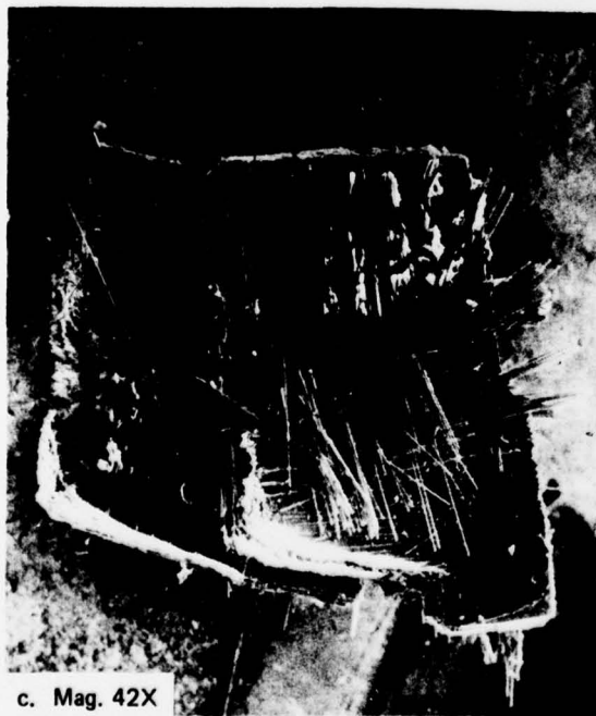
Figure 18. Comparison of low and high magnification scanning electron micrographs of 400 C isothermal aging residues from epoxy- and polyimide-based combinations.
