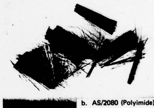
Figure 17. Photomicrographs of residues of epoxy- and polyimide-based combinations after 400 C isothermal aging for approximately one day. Mag. 7X.
