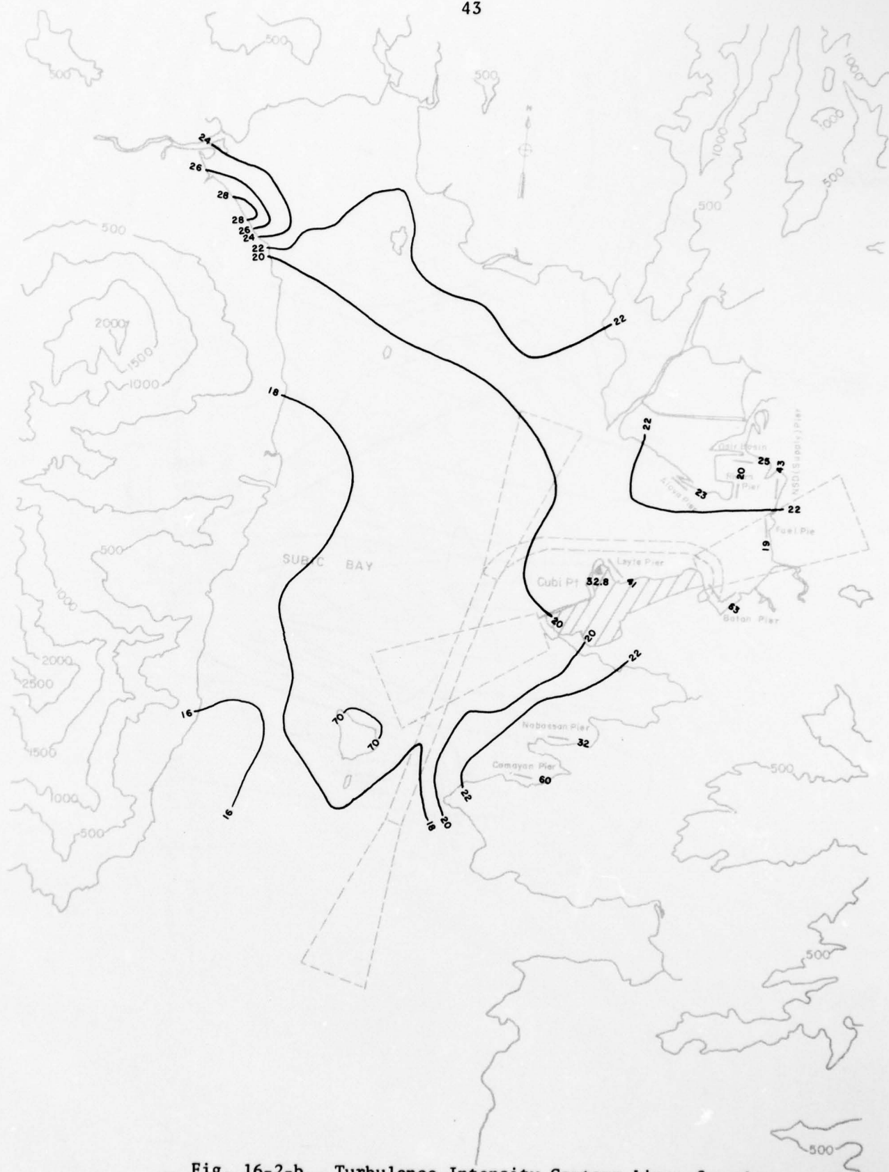
Fig. 16-2-b. Turbulence Intensity Contour Lines for the Subic Bay Basin at 195^{\circ}\text{T} , z = 150\text{ ft (45.7 m)}
