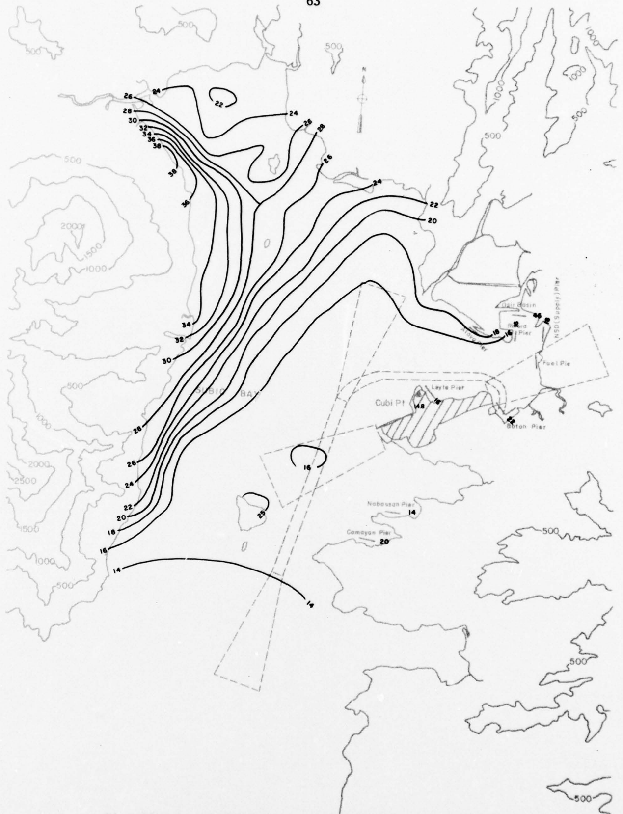
Fig. 18-4-b. Turbulence Intensity Contour Lines for the Subic Bay Basin at 225°T, z = 275 ft (83.9 m)
