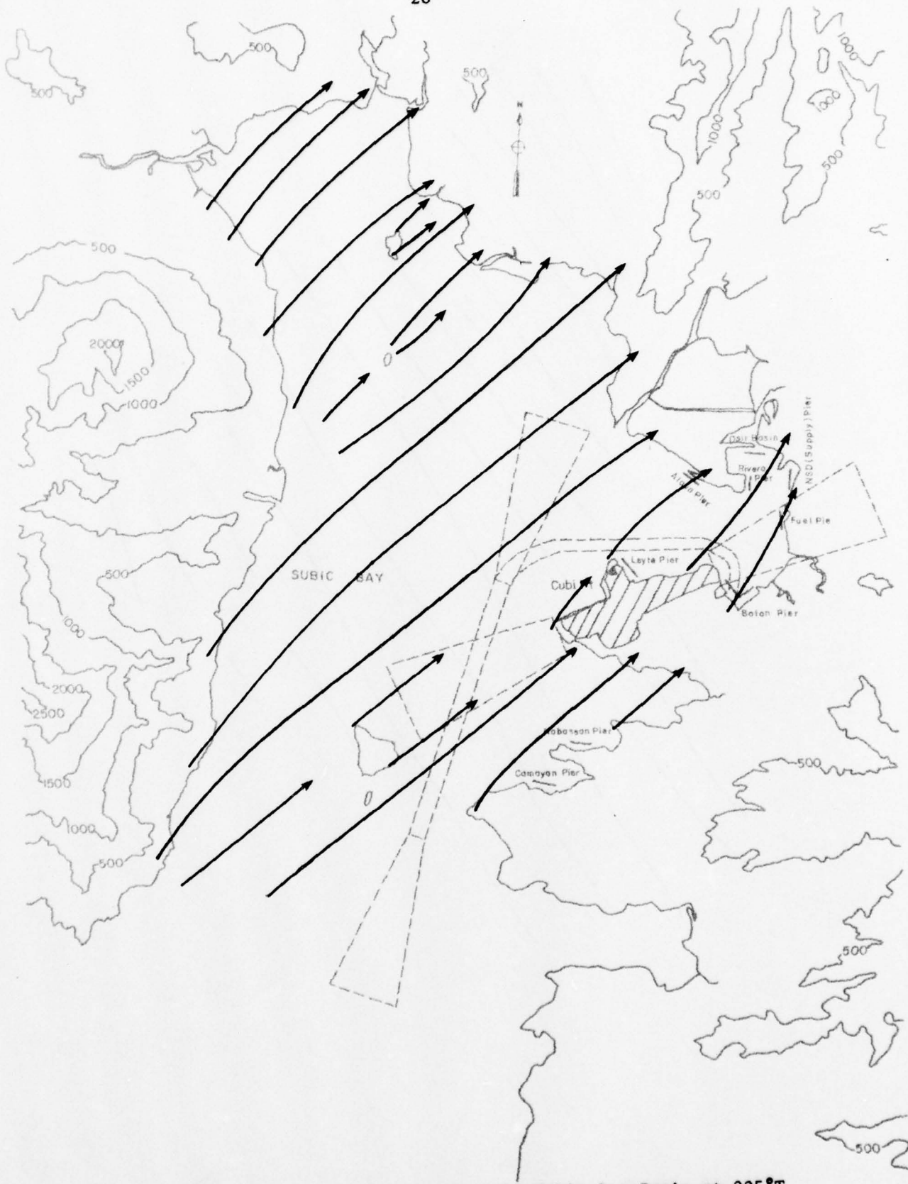
Fig. 11. Surface Streamlines for the Subic Bay Basin at 225°T
