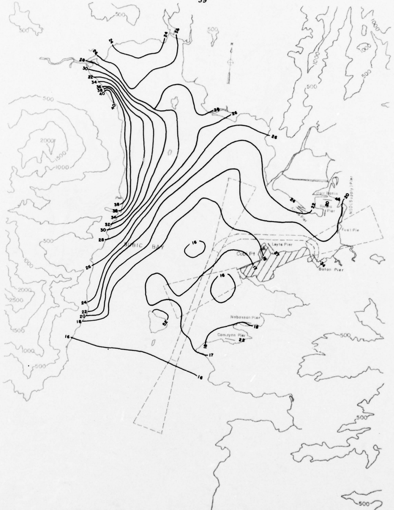
Fig. 18-2-b. Turbulence Intensity Contour Lines for the Subic Bay Basin at 225°T, z = 150 ft (45.7 m)
