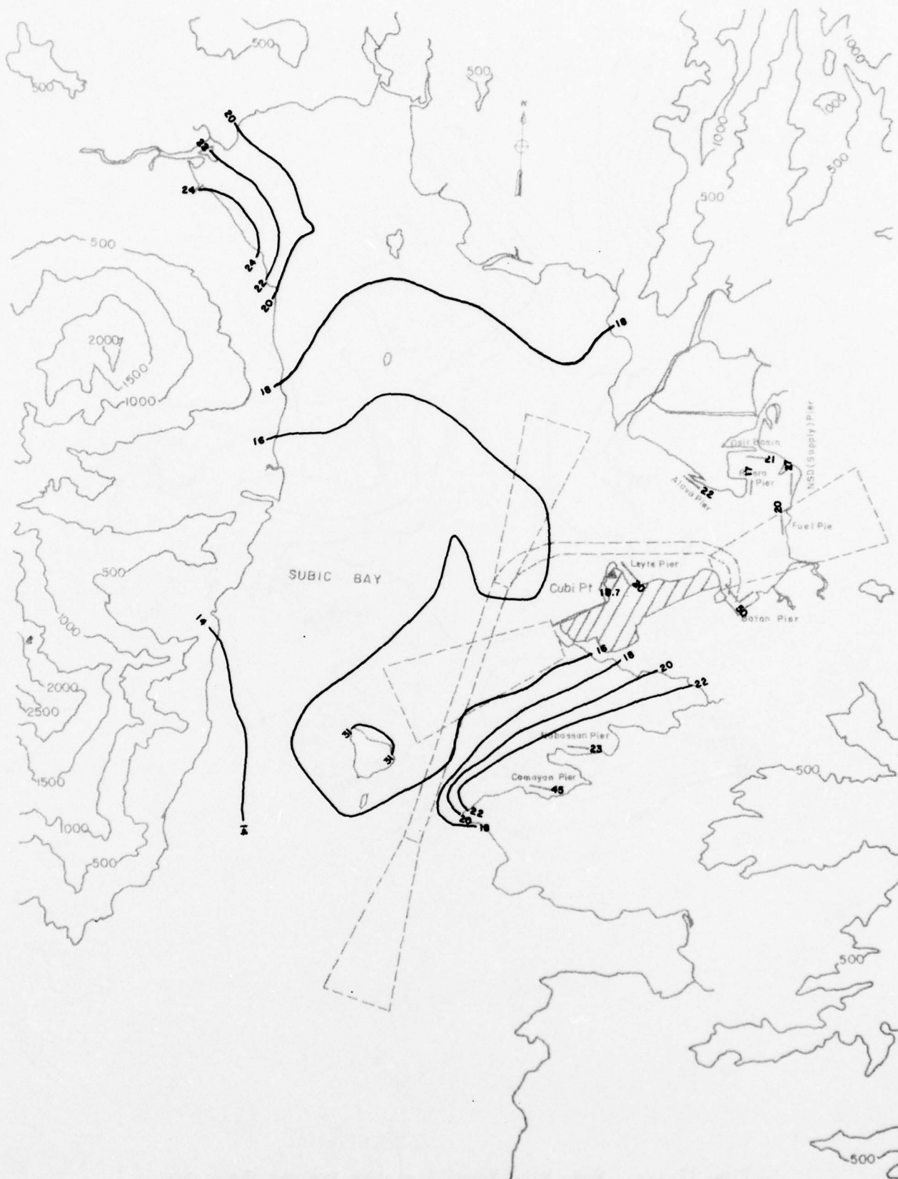
Fig. 16-4-b. Turbulence Intensity Contour Lines for the Subic Bay Basin at 195^{\circ}\text{T} , z = 275 \text{ ft (83.9 m)}
