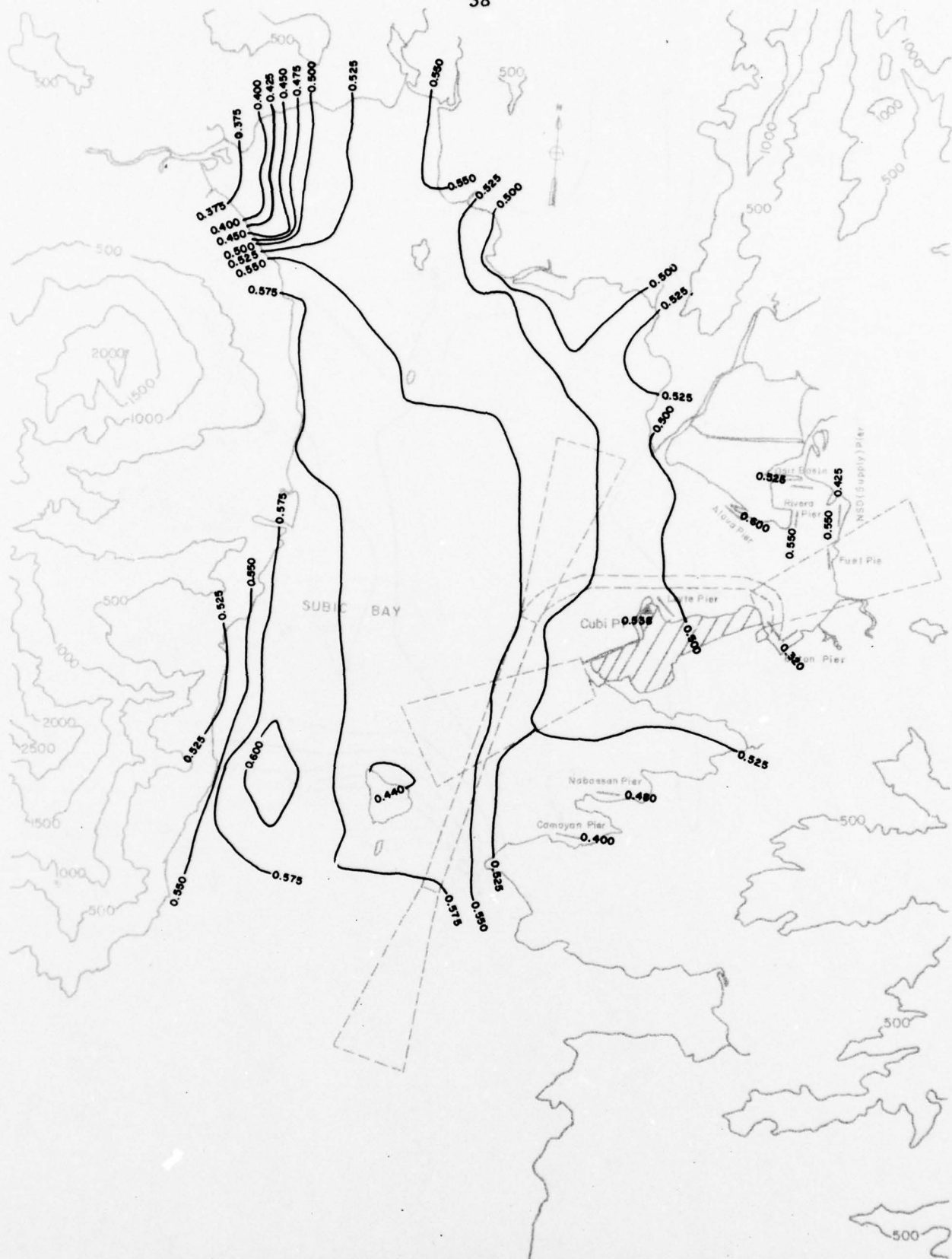
Fig. 15-4-a. Mean Wind Speed Isotachs for the Subic Bay Basin at 180°T, z = 275 ft (83.9 m)
