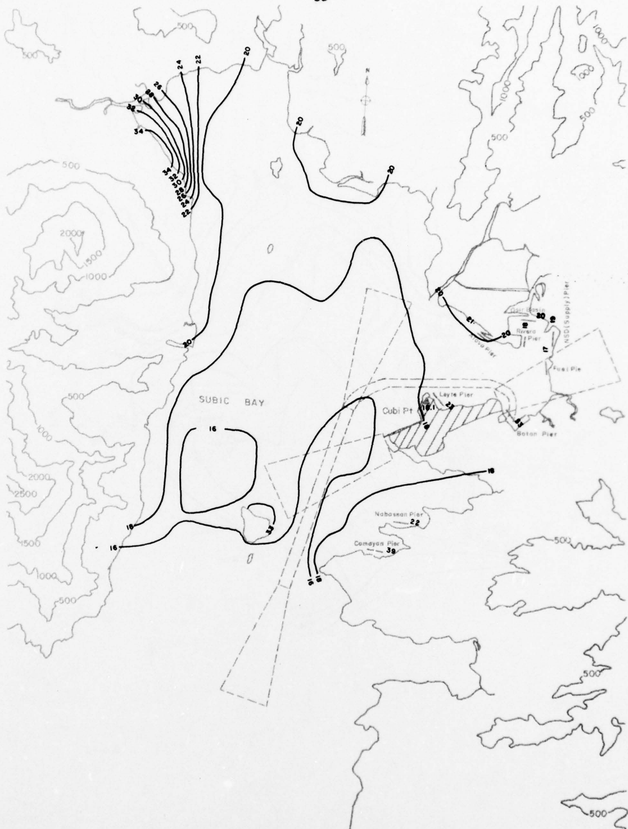
Fig. 17-4-b. Turbulence Intensity Contour Lines for the Subic Bay Basin at 210°T, z = 275 ft (83.9 m)
