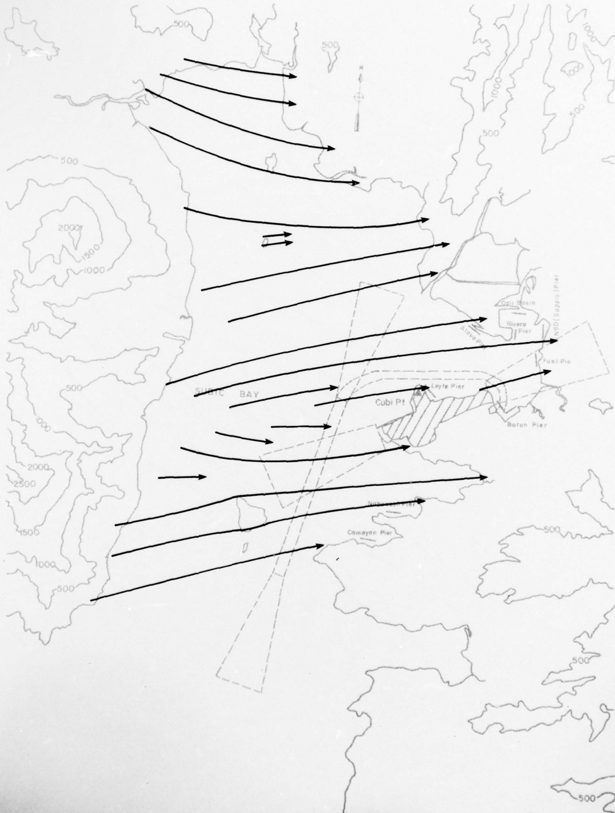
Fig. 13. Surface Streamlines for the Subic Bay Basin at 255°T
