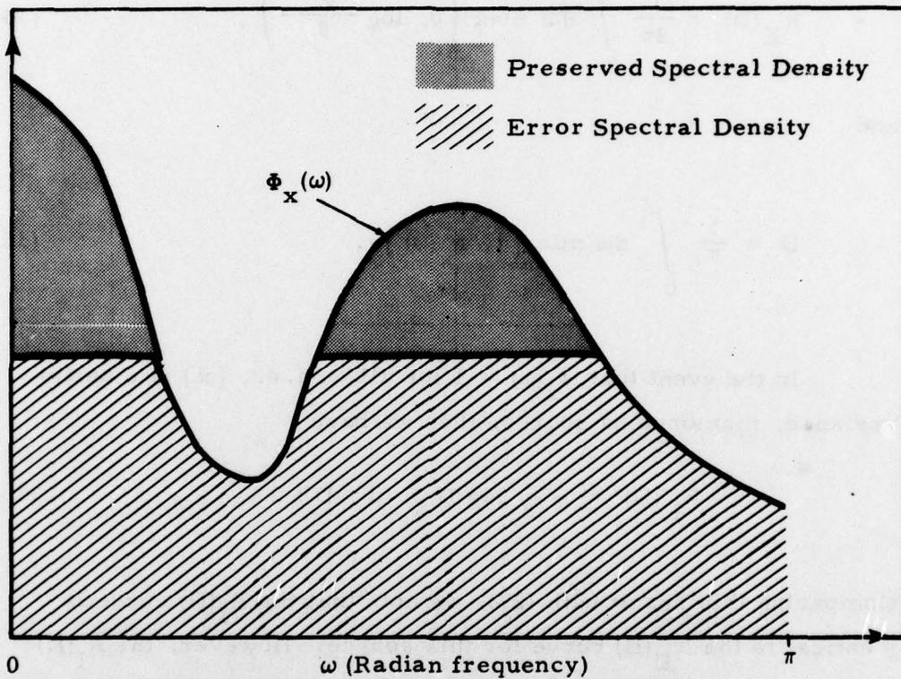
Figure 3. Illustration of preserved source and error spectral densities for optimum MSE encoding (see Berger [1], p. 122).
