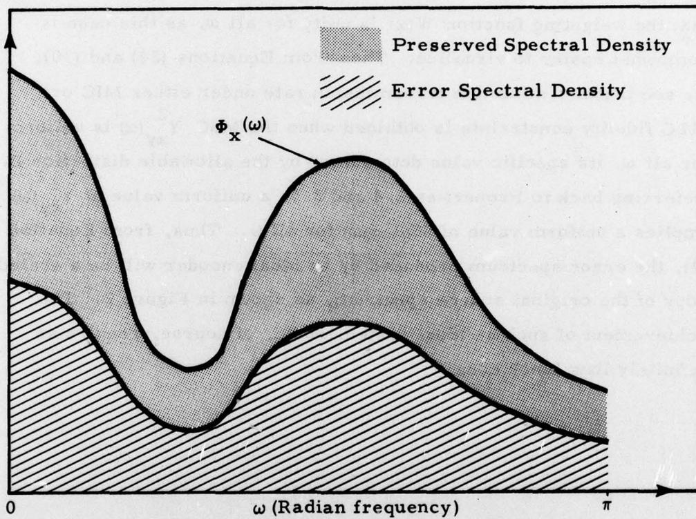
Figure 2. Illustration of preserved source and error spectral densities for optimum MIC or MLC encoding.
