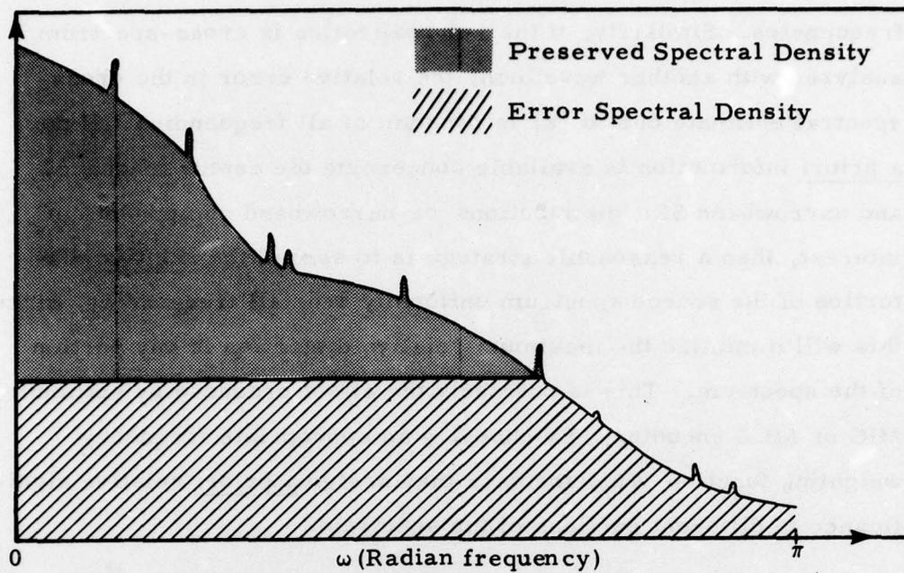
Figure 4(a). Example of optimum MSE encoding effects.
