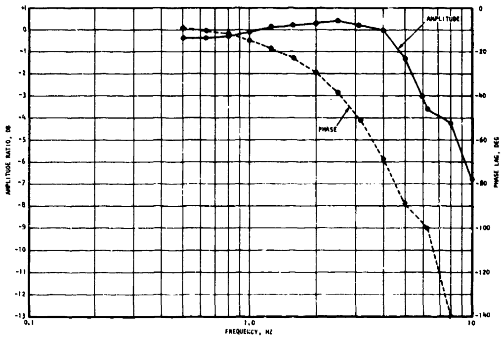
Figure 115. Frequency Response for Tachometer Feedback Servo, Dual-Channel 13,310 in.-lb Load, \pm 1 deg Amplitude
