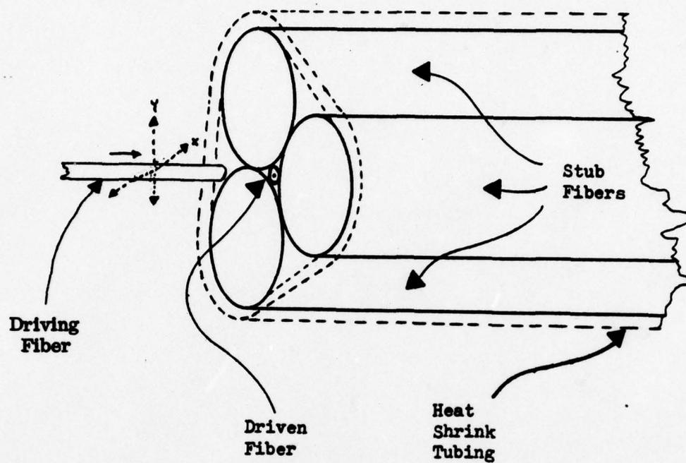
Figure 26. Experimental fiber coupling fixture.
