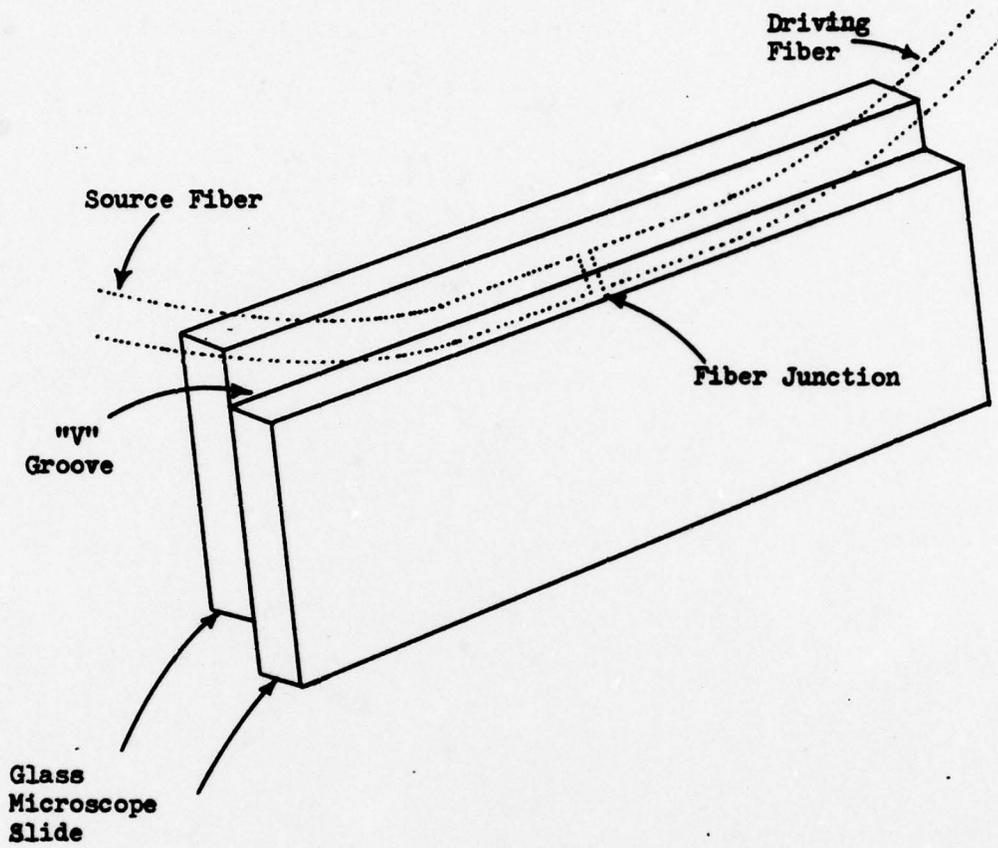
Figure 25. "V" Groove connecting device.
