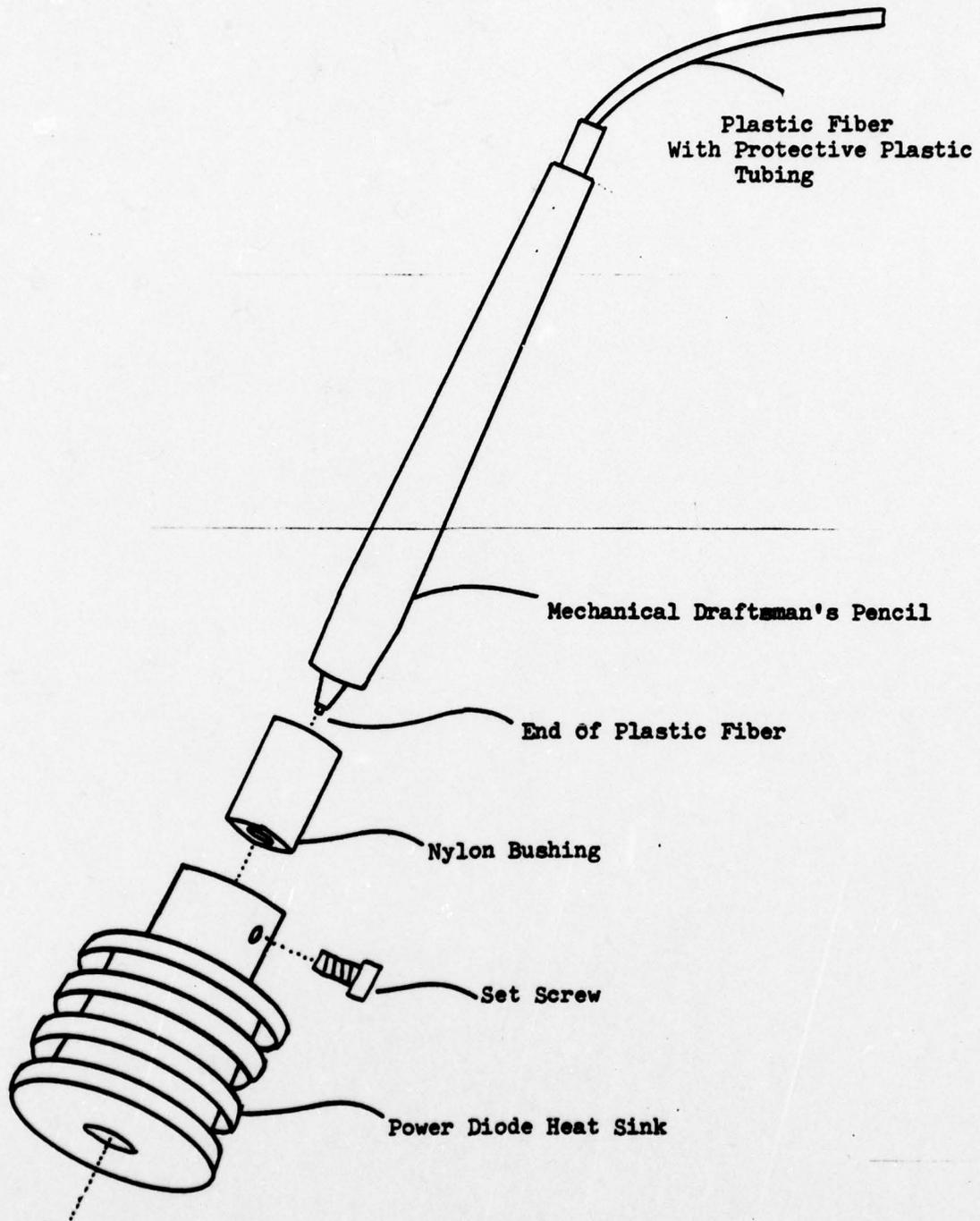
Figure 27. Plastic fiber polishing fixture.
