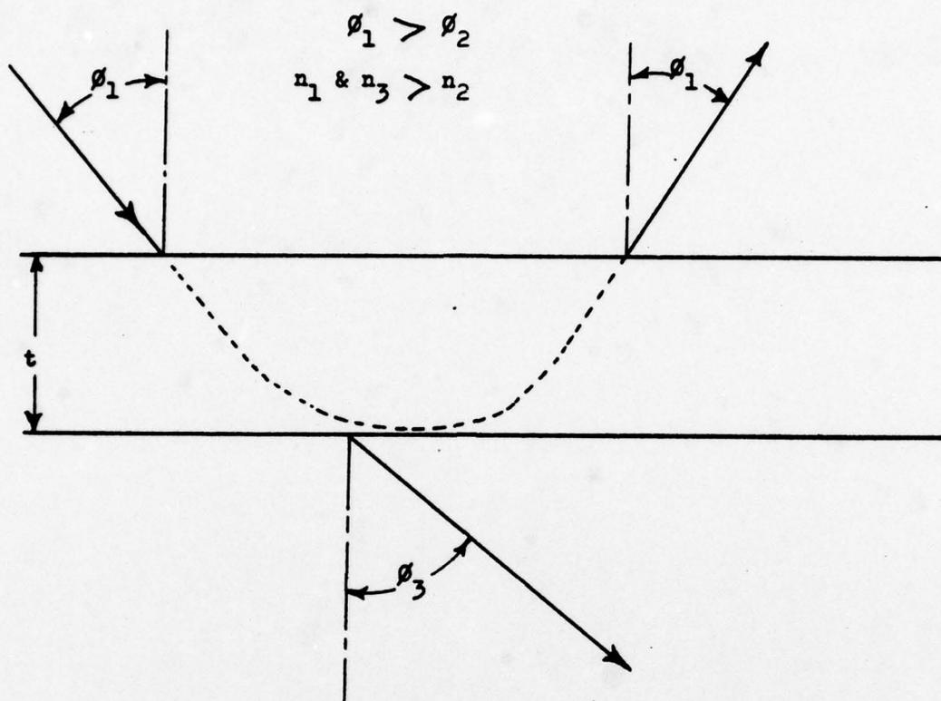
Figure 20. Frustrated total internal reflection of a light ray.
