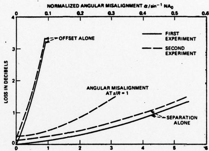
Figure 10. Loss in dB vs. normalized offset  $d/R$ , separation  $s/R$ , and angular misalignment  $\alpha/\sin^{-1} NA_0$ . (From Chu and McCormick)<sup>46</sup>
