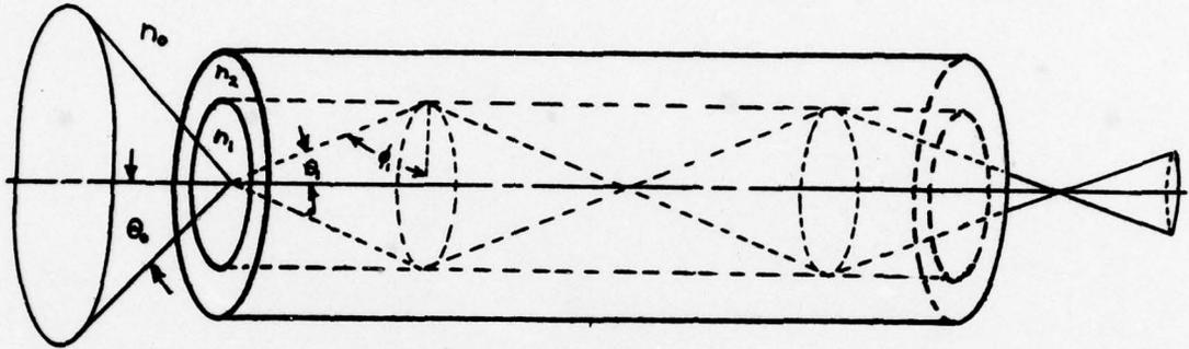
Figure 4. The cylindrical geometry of an optical fiber waveguide.
