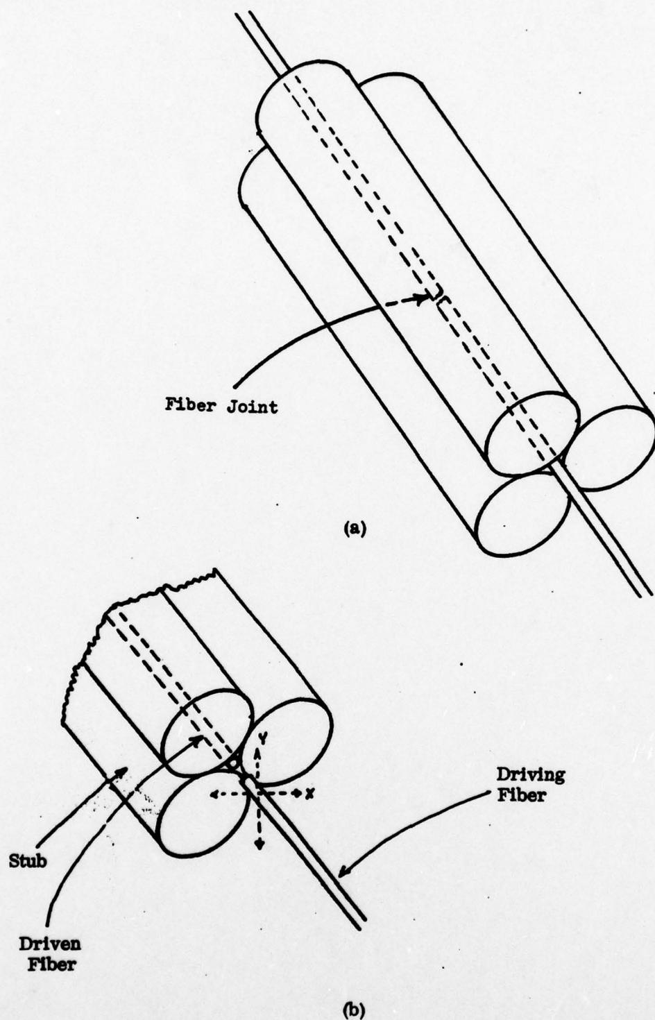
Figure 12. (a) The three rod fiber connector
