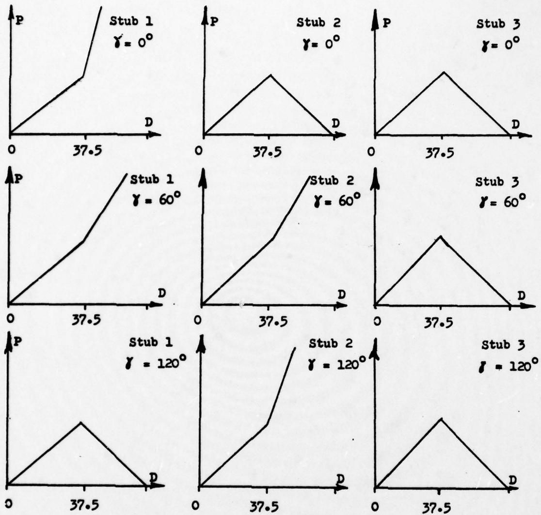
Figure 23. Estimated trends of stub power versus radial displacement for radial orientations of  $0^\circ$ ,  $60^\circ$ ,  $120^\circ$ .
