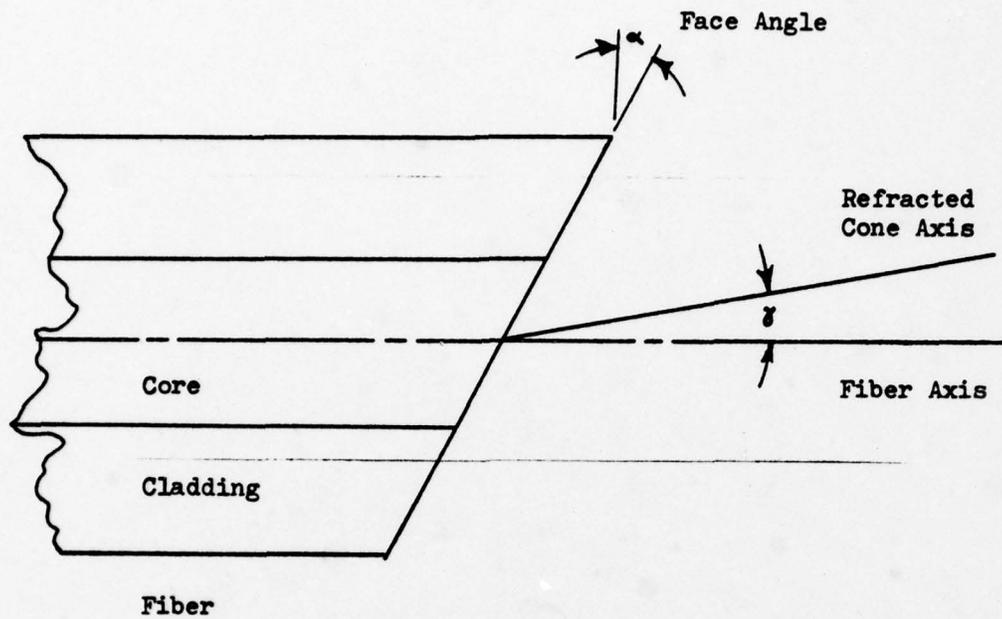
Figure 7. Relationship between fiber break angle and refracted cone axis. (From Gordon, Rawson, and Norton)<sup>37</sup>
