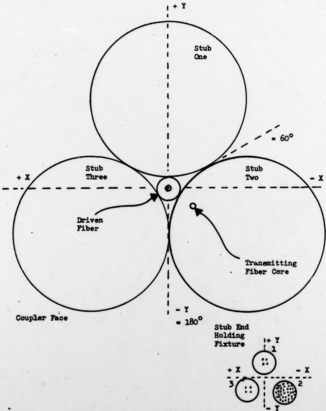
Figure 42. The offset transmitting fiber core located somewhere in the section of the coupler face bound by the  $60^\circ$  and  $180^\circ$  radials. The relative light intensity is represented by the number of dots in the circle representing a given fiber end.
