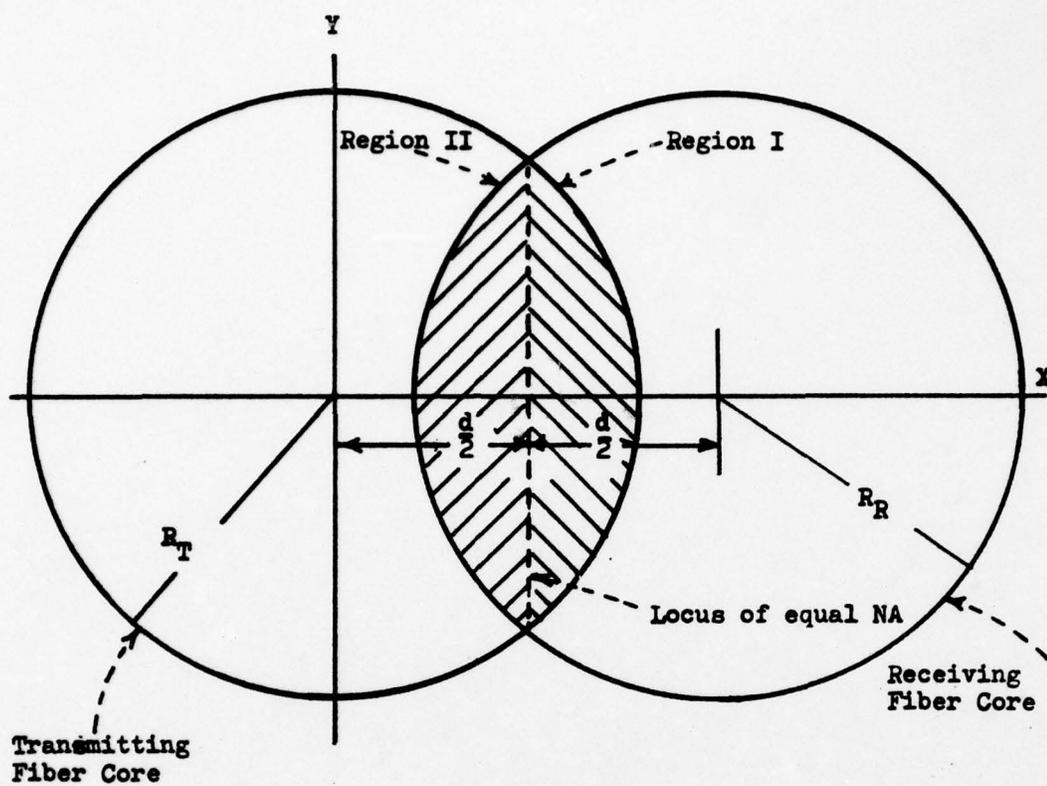
Figure 14. Overlapping regions of offset fiber cores ( $R_T = R_R$ )
