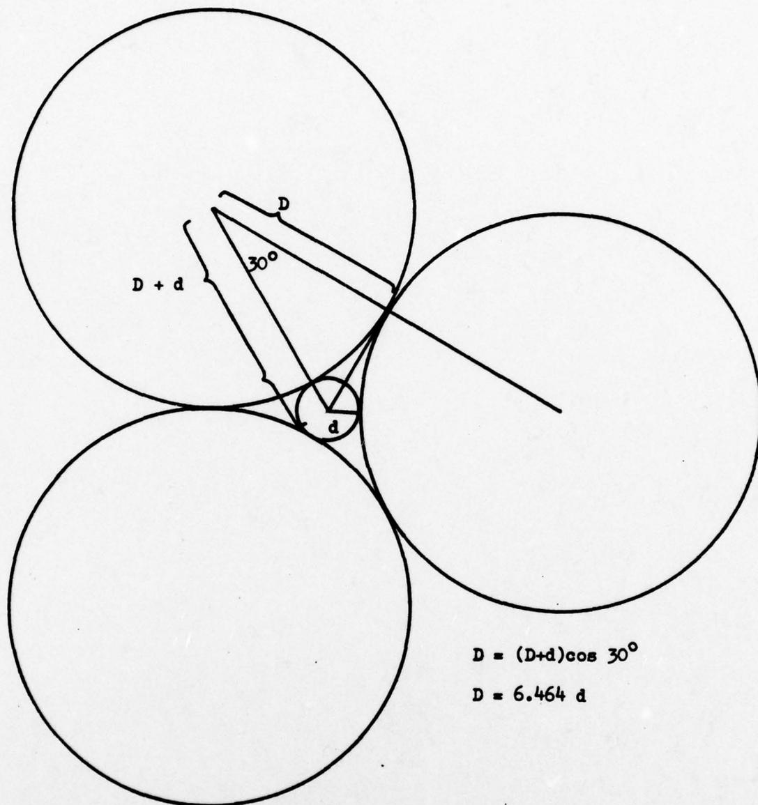
Figure 13. The three rod geometry.
