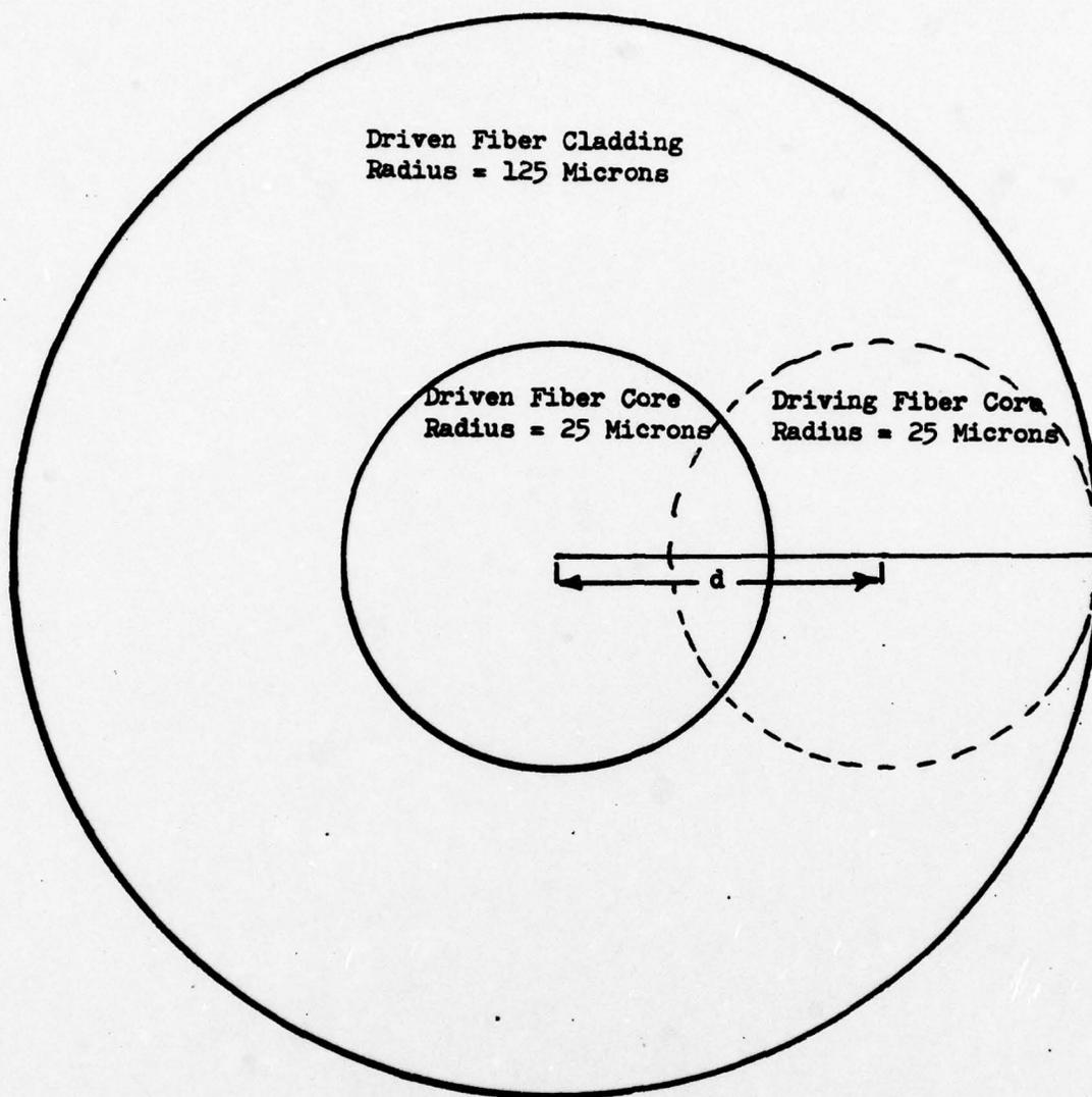
Figure 18. Driving fiber core displaced by  $d = 37.5$  microns, along radial line  $\theta = 90^\circ$ . 37.5 microns is the maximum displacement where light from the driving fiber core falls within the periphery of the driven fiber cladding.
