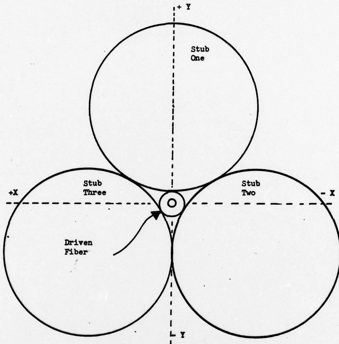
Figure 29. Orientation of X and Y axes of the coupler face.
