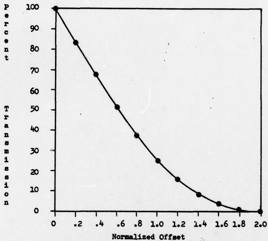
Figure 15. Calculated transmission in percent versus offset normalized to core radius.
