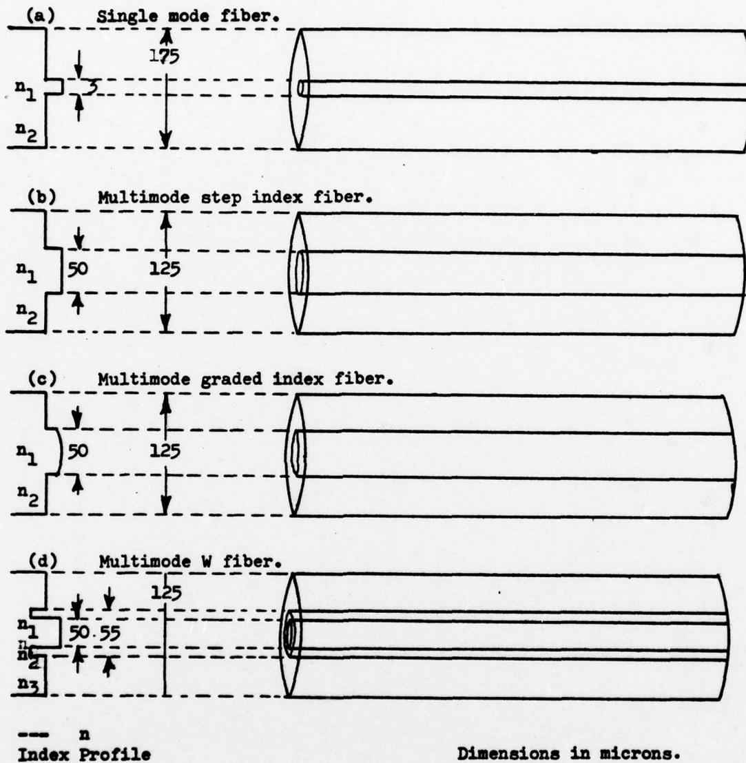
Figure 6. Types of fiber index profiles. (From Ramsay, Hockham, and Kao)<sup>25</sup>
