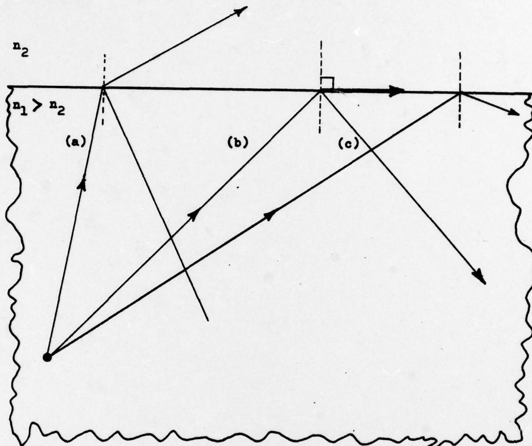
Figure 2. a) Ray prior to critical incidence, b) critical ray, and c) a totally reflected ray. (From Halliday and Resnick)<sup>9</sup>
