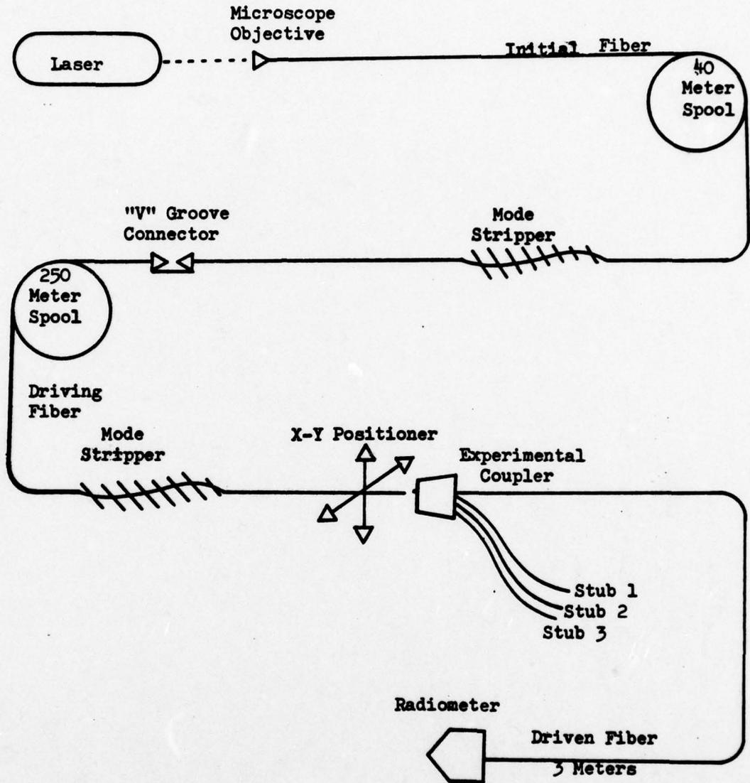
Figure 24. Schematic diagram of the experimental apparatus.
