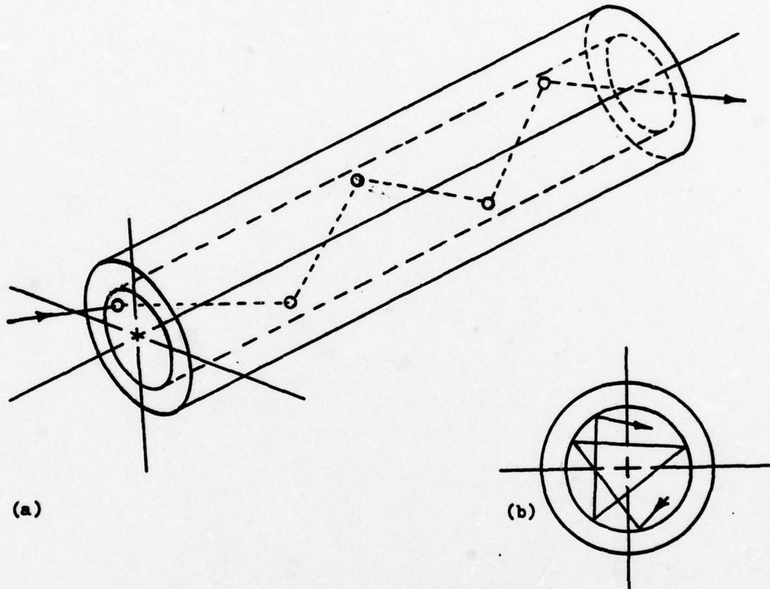
Figure 5. a) A skew ray traveling in an optical waveguide, b) helical path of the skew ray. (From Kapany)<sup>16</sup>
