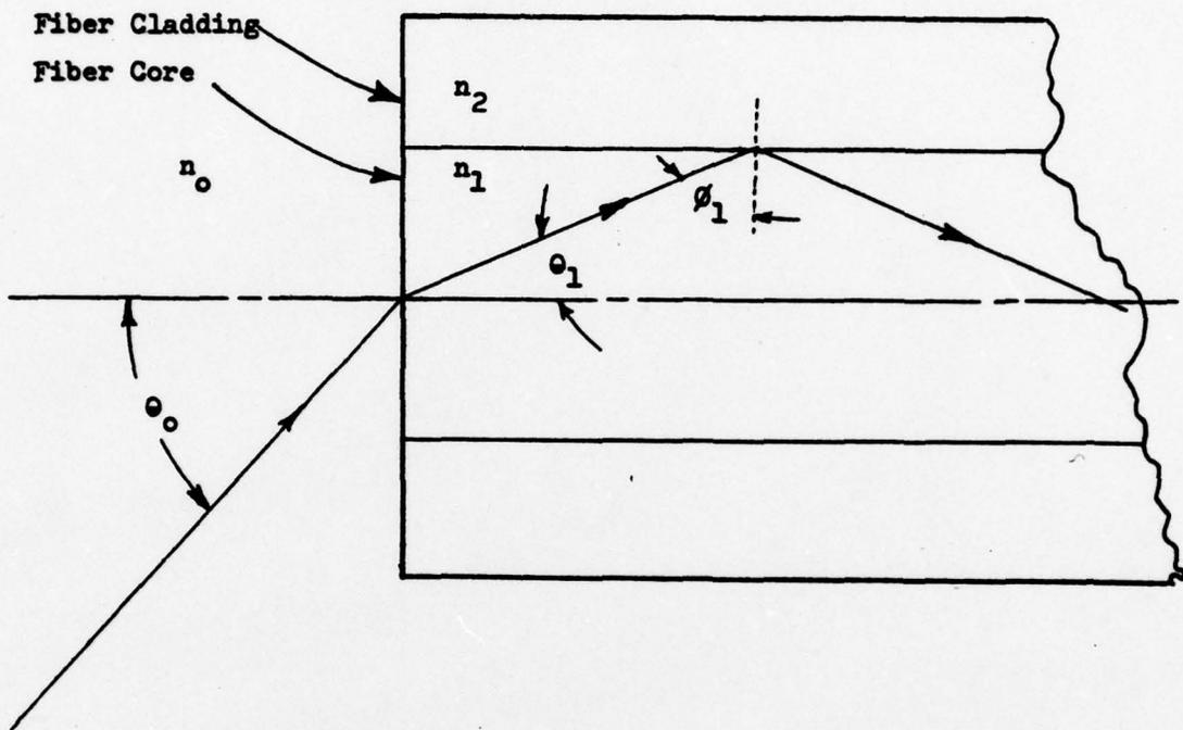
Figure 3. Angular relations for a ray of light being launched into an optical fiber. (From Kapany)<sup>10</sup>
