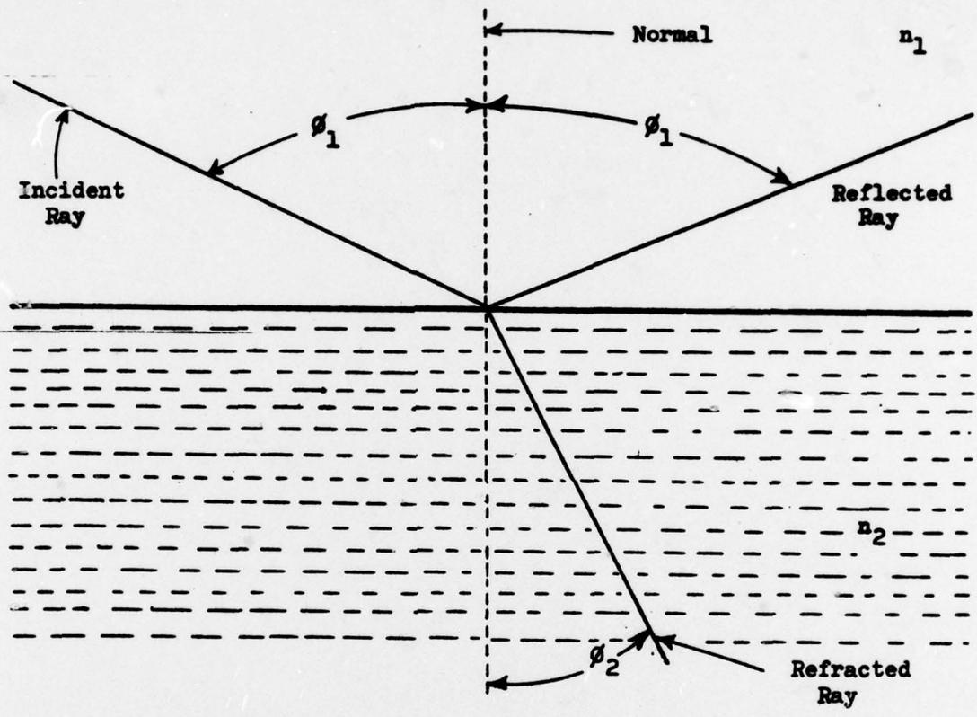
Figure 1. Incident, reflected, and refracted light rays at the interface between two optical media. (From Halliday and Resnick)<sup>6</sup>
