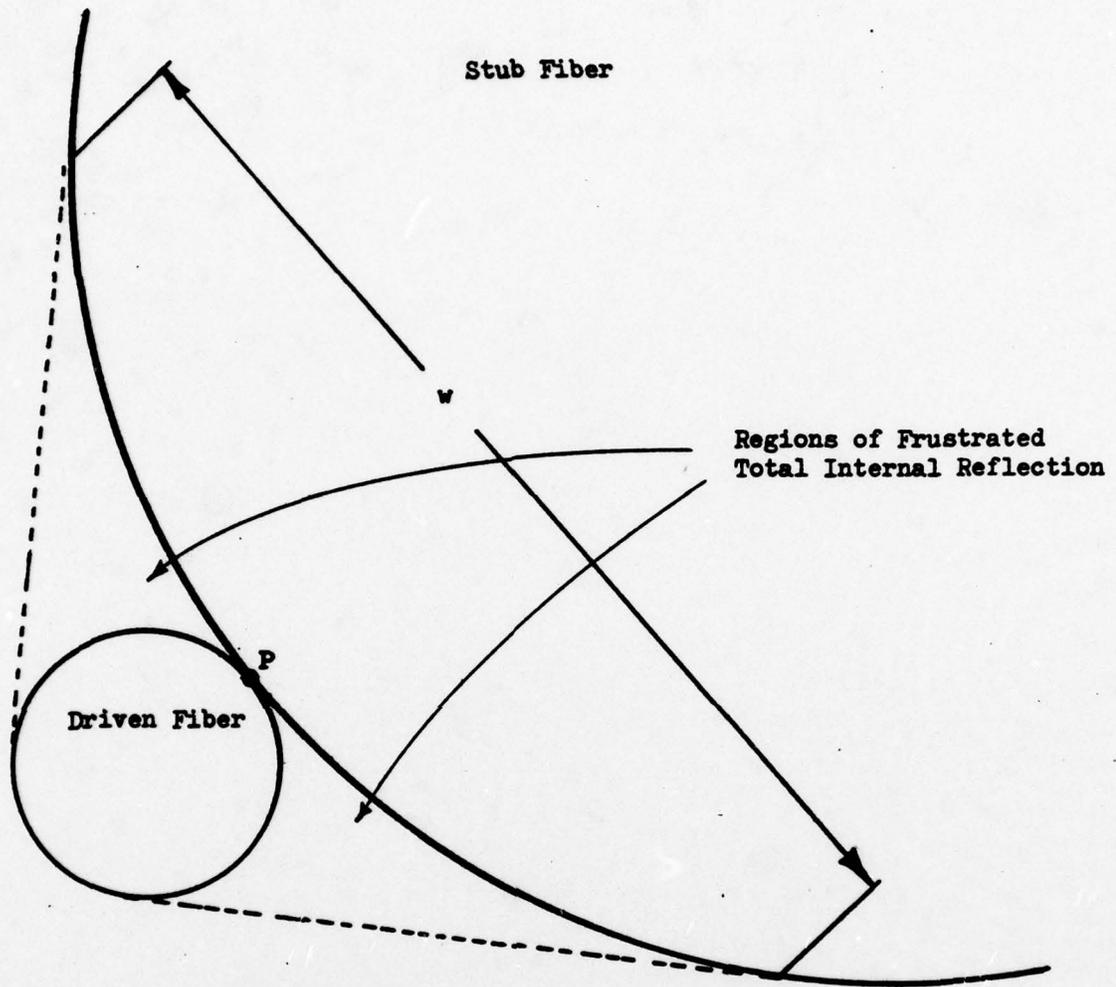
Figure 21. Regions of frustrated total internal reflection for the Stub Coupler geometry. <sup>72</sup>
