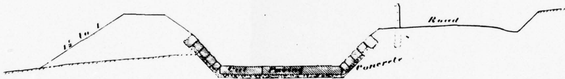
Section of Flood Water Channel and Highway
