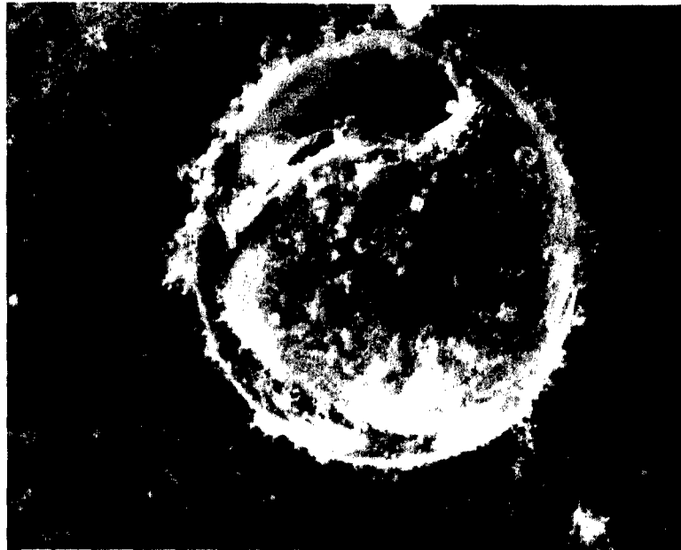
Figure 6. Scanning electron micrograph of a large particle found in the product of a SRF burn. Magnification is about 4000x.
