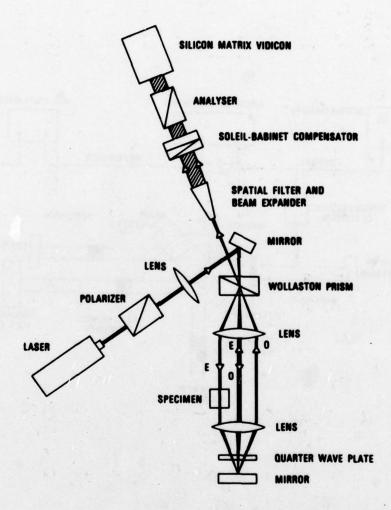
Figure 10. Modified Dyson interferometer for measuring piezo-optic constants in the visible.
