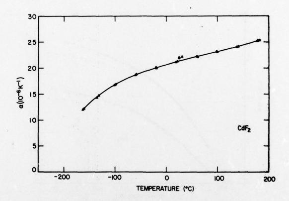
Figure 6. Linear thermal expansion coefficient of CdF<sub>2</sub> as a function of temperature. The triangles show our experimental data and the single circle is from S. S. Ballard and J. S. Browder, Appl. Opt. 5, 1873 (1966).
