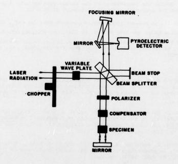
Figure 11. Double pass arrangement for measuring piezo-birefringence at 10.6  $\mu m\,.$
