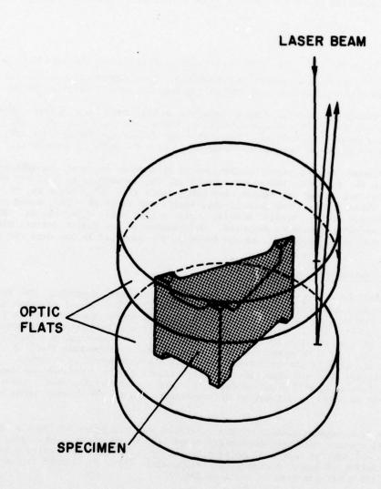
Figure 2. Fizeau interferometer for measuring linear thermal expansion.
