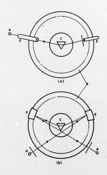
Figure 1. (a) Schematic of spectrometer used for visible region refractometry. (b) Schematic of spectrometer used for non-visible region refractometry. Symbols: A = source, B = divided circle, C = prism table, D = collimator, E = telescope, F = collimating mirror, G = movable mirror, H = detector.
