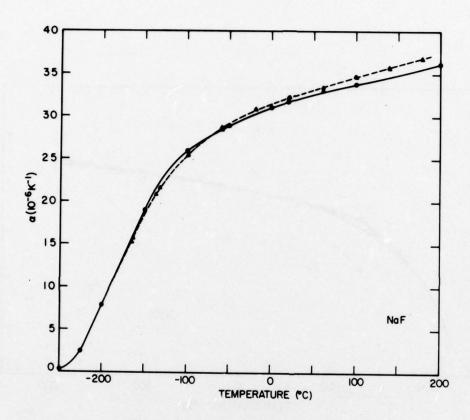
Figure 5. Linear thermal expansion coefficient of NaF. The triangles are our experimental data and the circles are from the AIP Handbook [13].
