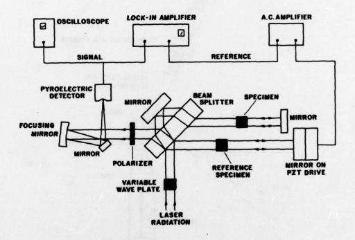
Figure 9. Modified Twyman-Green interferometer for measuring piezooptic constants at 10.6 µm.
