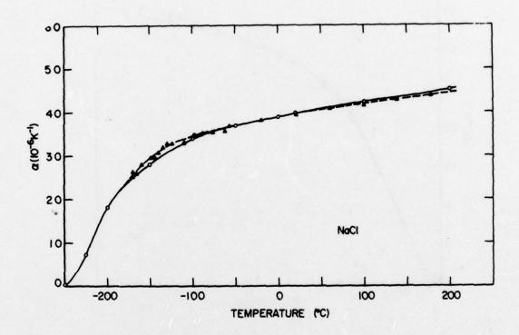
Figure 4. Linear thermal expansion coefficient of NaCl as a function of temperature. The triangles are our experimental data and the circles are from the AIP Handbook [13].
