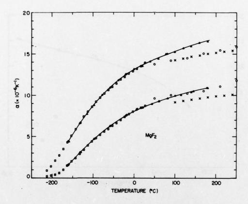
Figure 7. Linear thermal expansion coefficients of single crystal MgF as a function of temperature. The upper curve is for  $\alpha_{\parallel}$ ; the lower curve is for  $\alpha_{\parallel}$ .  $\parallel$  and  $\parallel$  refer to parallel and perpendicular to the c axis, respectively. The curves and triangles are our data; the squares are from Ref. [11], the circles from Ref. [10], and the x's from [14].
