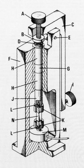
Figure 8. Stressing apparatus. A = adjustment screw with domed tip,
