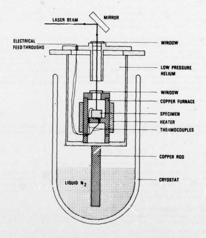
Figure 3. Apparatus for measuring linear thermal expansion and thermooptic constants as a function of temperature over the range -180 °C to 200 °C.
