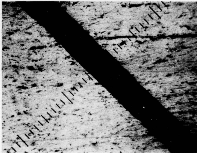
(b) 4 MIL SCARF JOINT (100X)
