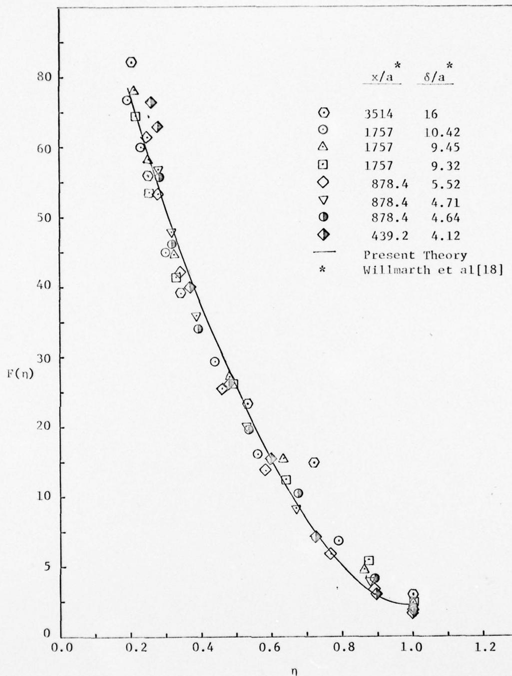
Figure 16. Velocity-Defect Law ( Mixing-Length Model )
