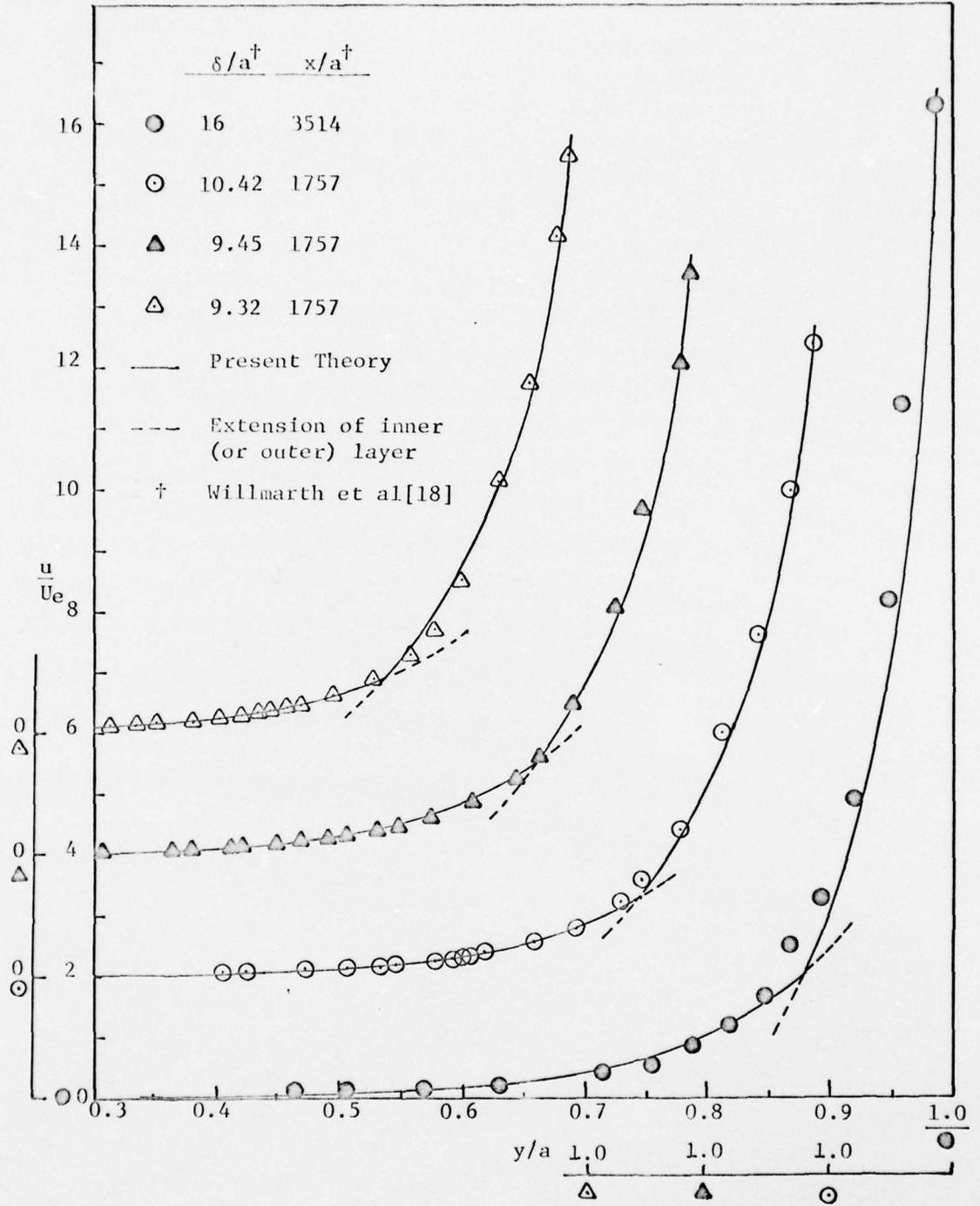
Figure 17. Comparison of Velocity Profiles
