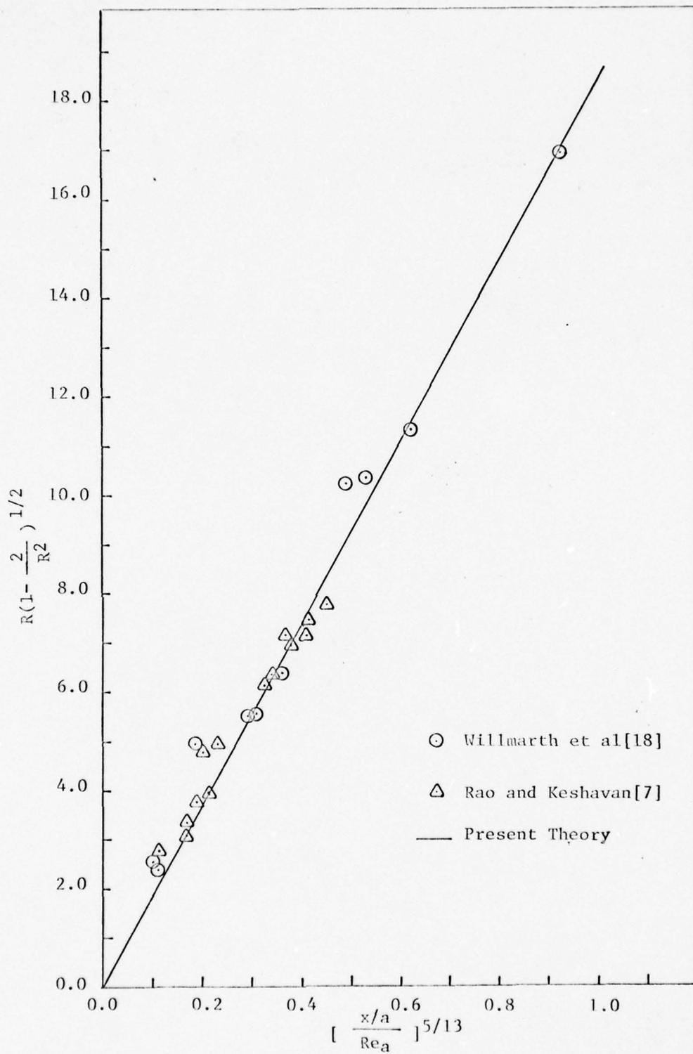
Figure 12. Boundary-Layer Thickness ( Eddy-Viscosity Model )
