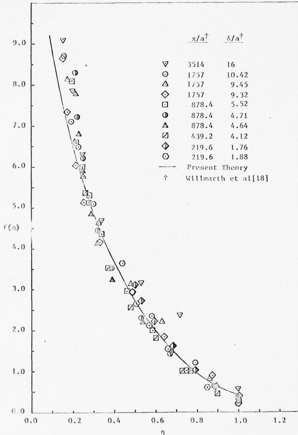
Figure 13. Velocity-Defect Law ( Eddy-Viscosity Model )
