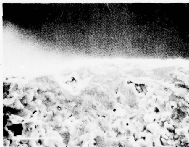
B. Fracture origin (500x)
