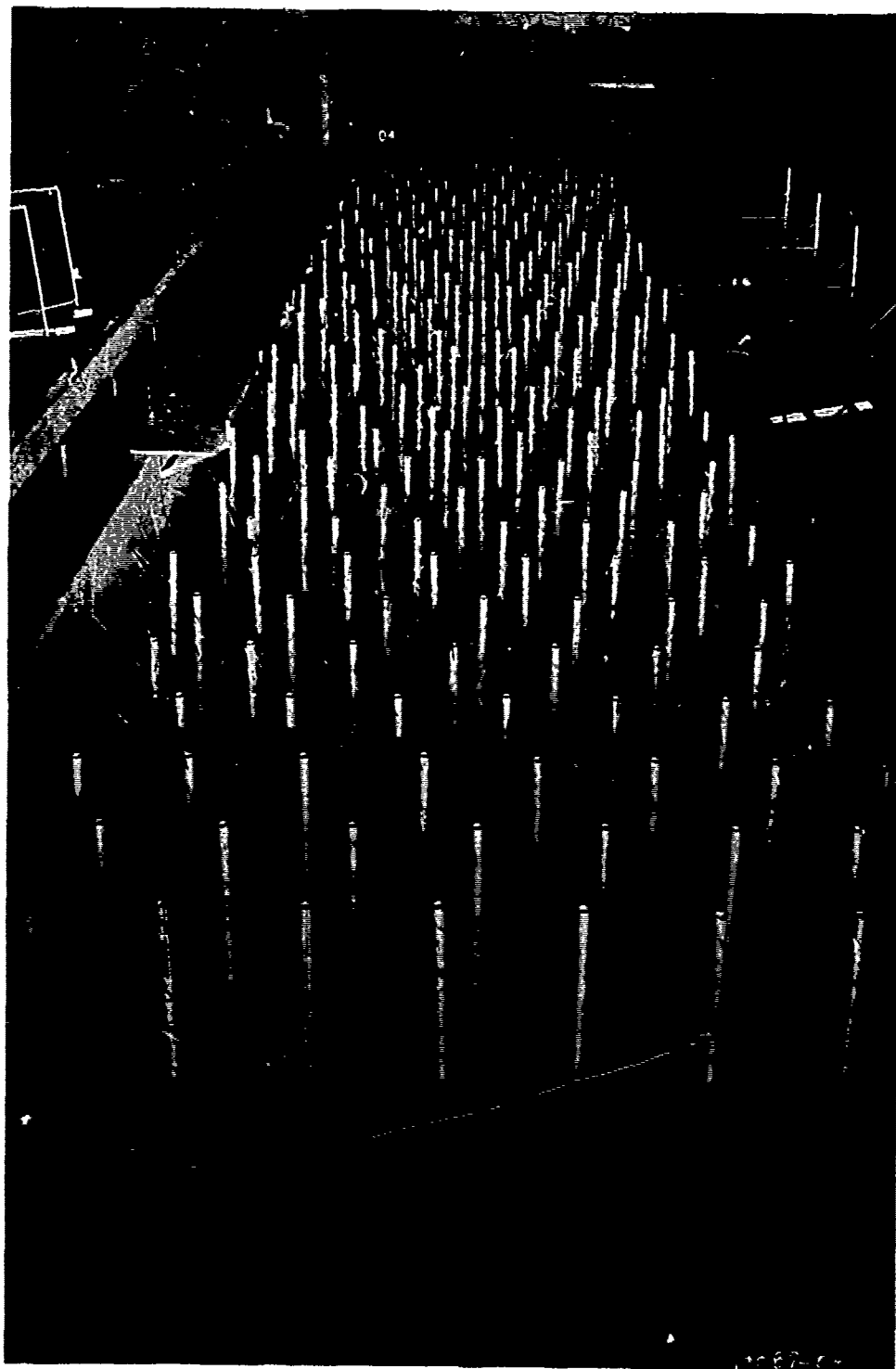
Photo 9. Plan 12, 12-in.-diameter stems with 1-1/4-in. branches without water in flume
