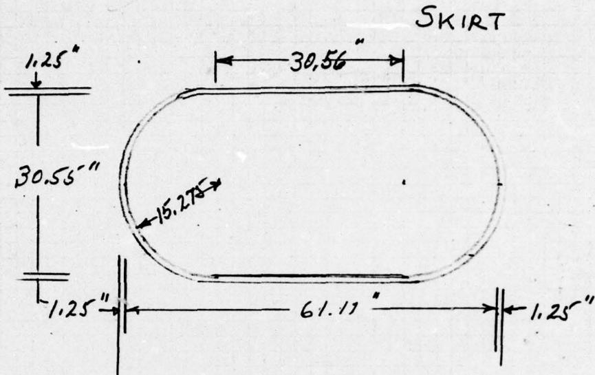
THE INTERNAL LOADS IN THE SKIRT SHOWN IN TABLE II (PAGE 6) AND DEFLECTION ( $\delta$ ) SHOWN IN TABLE III (PAGE 7) ARE BASED ON THE DIMENSIONS SHOWN ON PAGE 1. THE SIZE OF THE SKIRT WAS CHANGED TO THE DIMENSIONS SHOWN ABOVE. THIS RESULTS IN A REDUCTION IN INTERNALS LOADS AND DEFLECTION. TO  $\frac{15.275}{19.595} = .7795$  OF THE VALUES SHOWN
