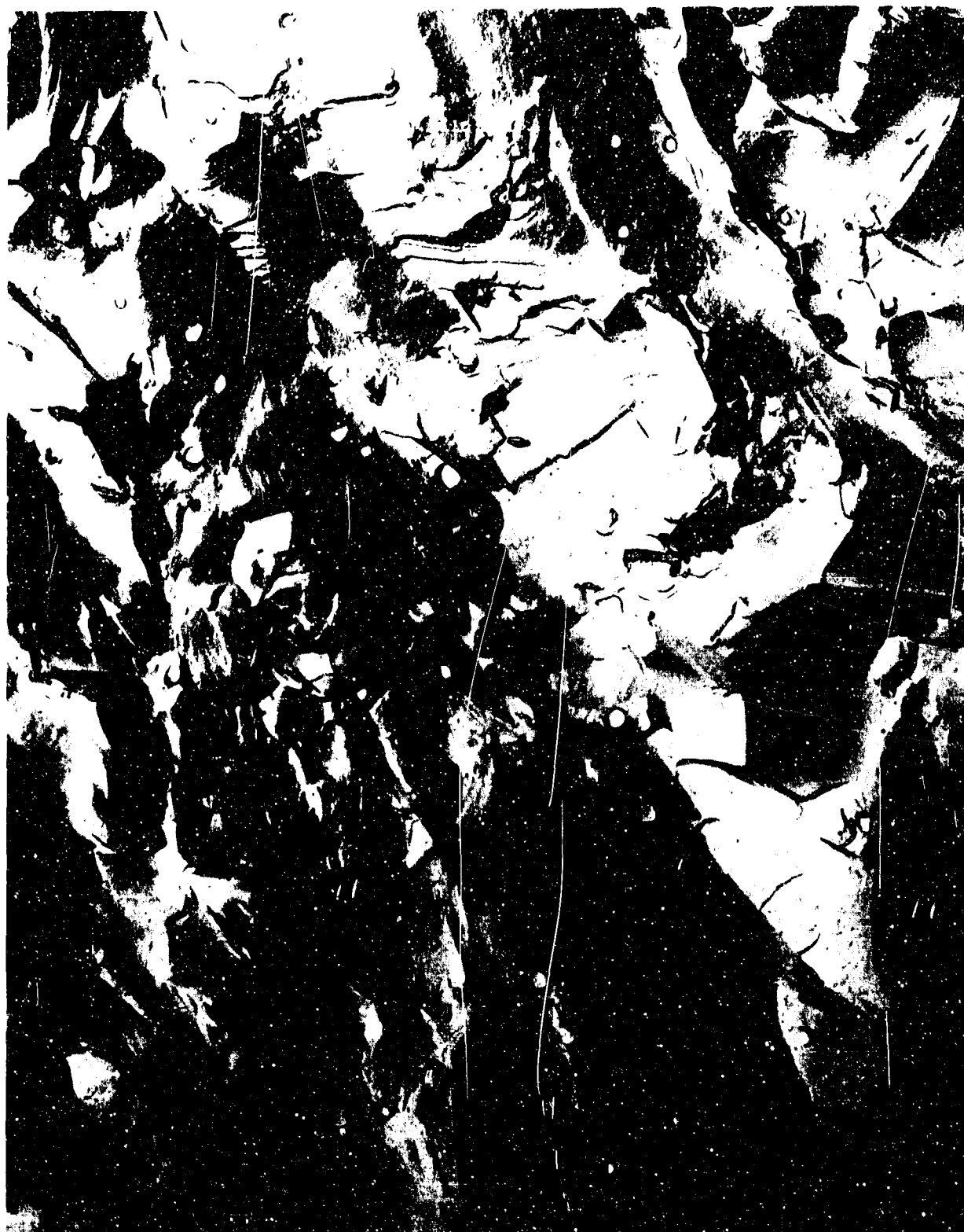
Fig. 16 Replica of Fracture Surface of HIP Be, 0.70 BeO, Upset-Forged 1033 K, Reduced 75% by Rolling at 922 K and Annealed at 977 K for 10 min. The structure mainly cleavage failure with isolated areas of fine intergranular fracture. Magnification 8000 \times .
