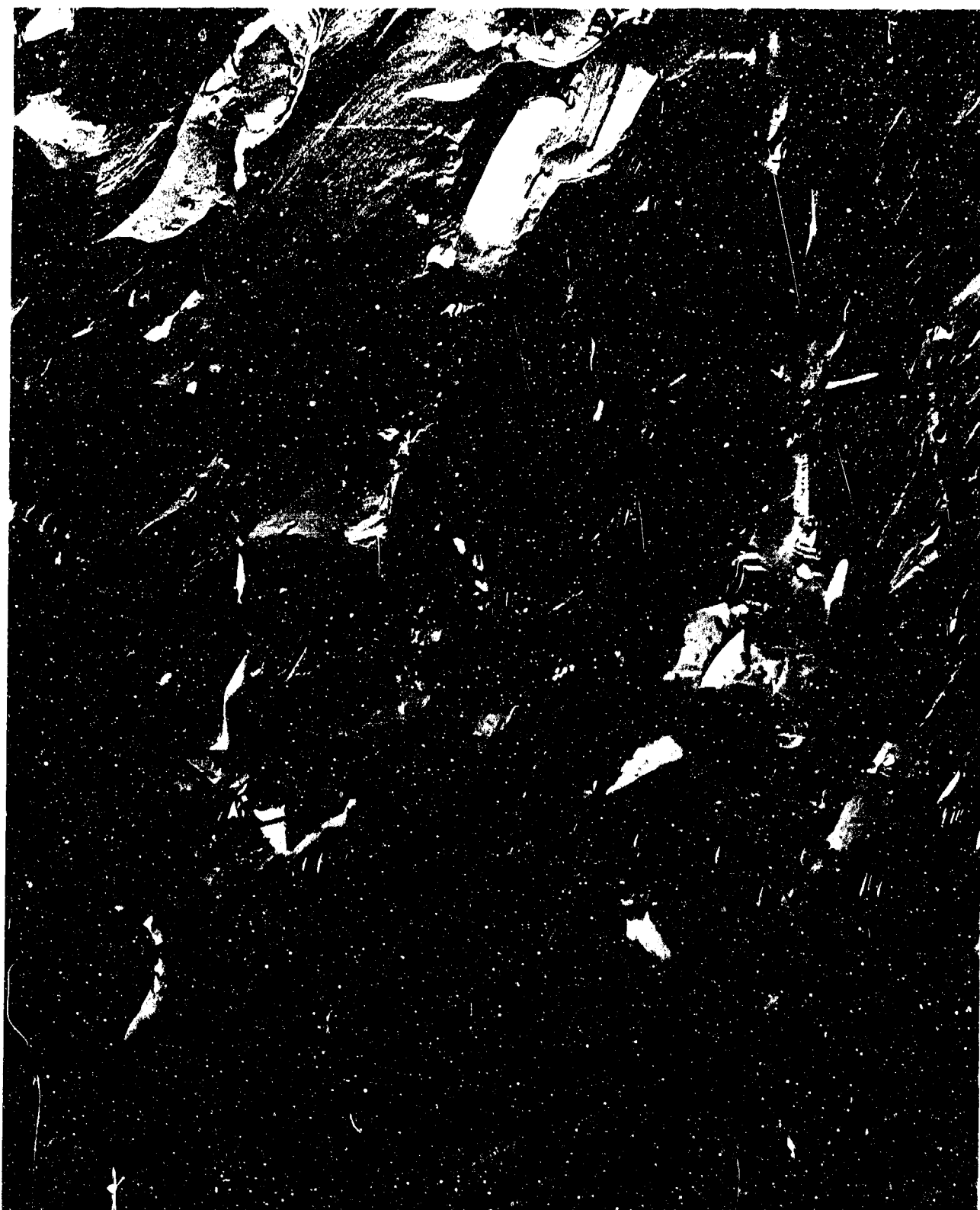
Fig. 15 Replica of Fracture Surface of HIP 1.56% BeO (RR243) Extruded 10:1 at 1033 K and Annealed for 1 hr at 1144 K. The fracture shows a mixture of fine (1-3 \mu\text{m} ) intergranular failure and coarser transgranular cleavage failure. BeO particles up to about 200-nm diameter can be seen in the regions of intergranular separation. Magnification 15,000 \times .
