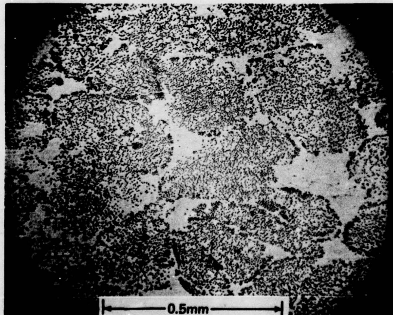
Figure 2. SEM Photographs of 30 V/o GR/Al Plate Sliced Transverse to the Fiber Direction (3) at Two Magnifications: (a) 30X Illustrating the Sample Plate Boundaries and Random Fiber Bundle Arrangements; and (b) 100X Illustrating the Al Infiltrated Array of Fibers in Each Bundle.
