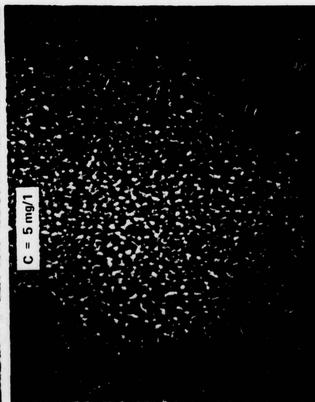
FIGURE 5. Scanning Electron Micrographs of Polyamide Membrane at Time = 45 Days (14,000x)
