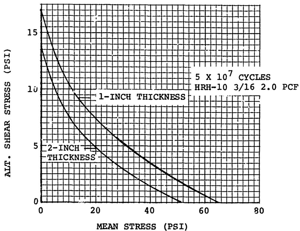
Figure 100. Nomex Honeycomb Goodman Diagram, Shear
