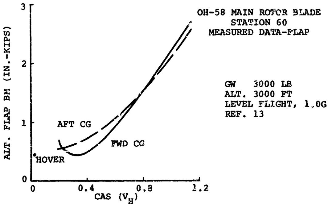
Figure 104. Alternating Flap Bending Moment Vs. Airspeed
