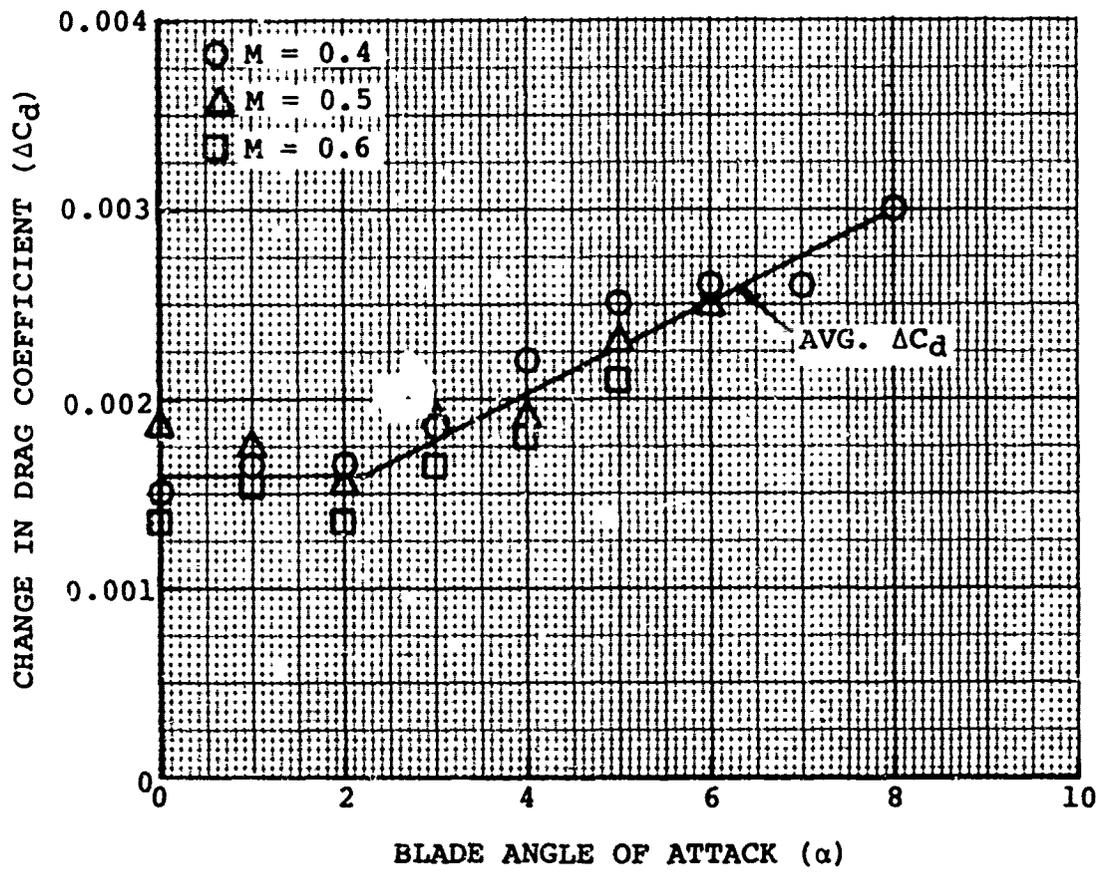
Figure 17. Drag Increments Applied to 0012 Data
