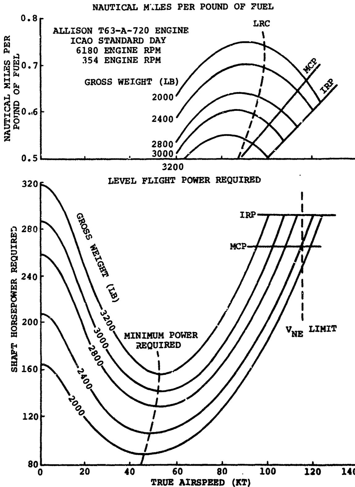
Figure 87. Level Flight Performance 10,000 Feet
