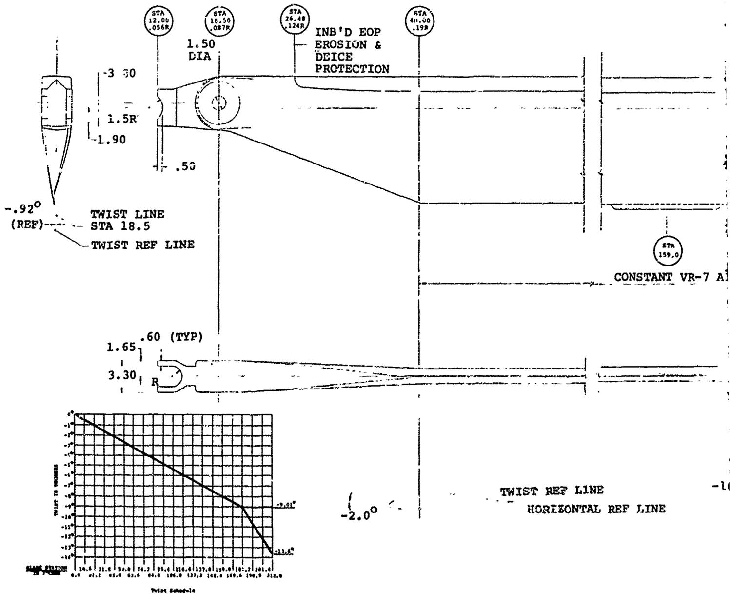
Figure 4. OH-58C/A Composite Blade Geometry
