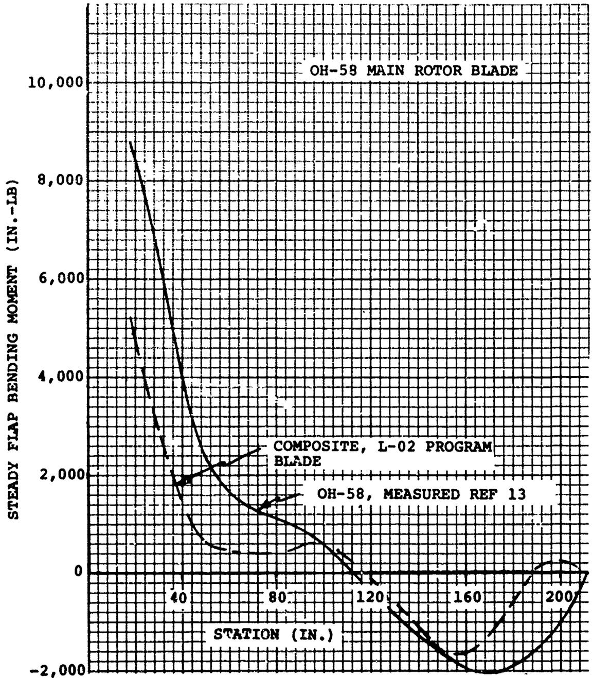
Figure 112. Steady Flap Bending Moment-Spanwise Distribution
