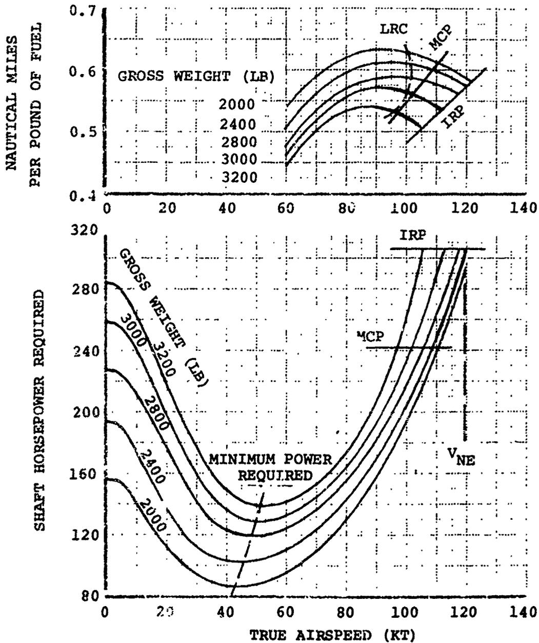
Figure 90. Level Flight Performance, 4000 Ft, 95°F,
