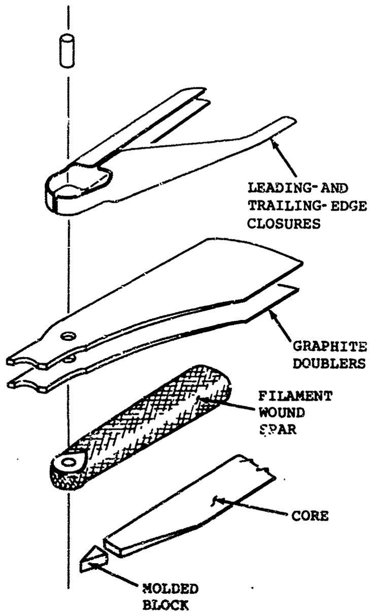
Figure 12. Filament Wound Root End Design
