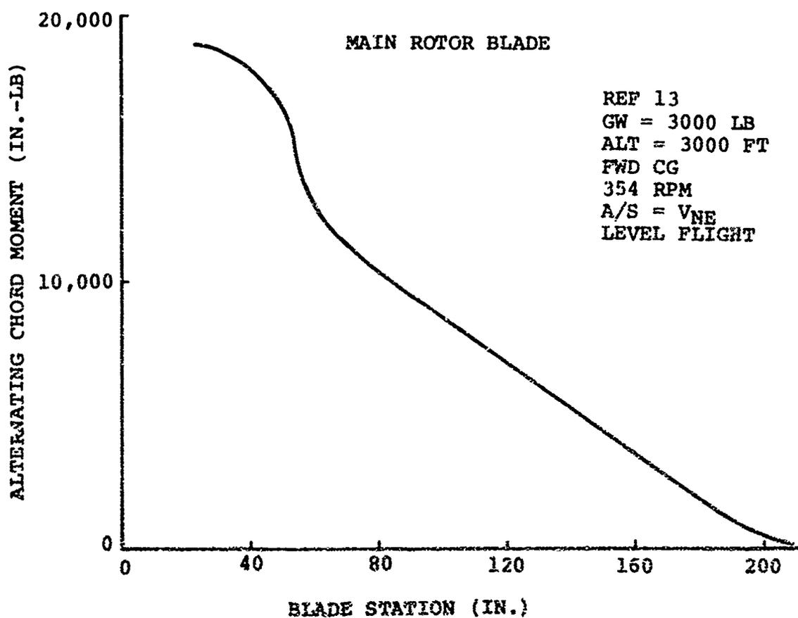
Figure 109. Measured Alternating Chordwise Bending Moment Model 205A-1
