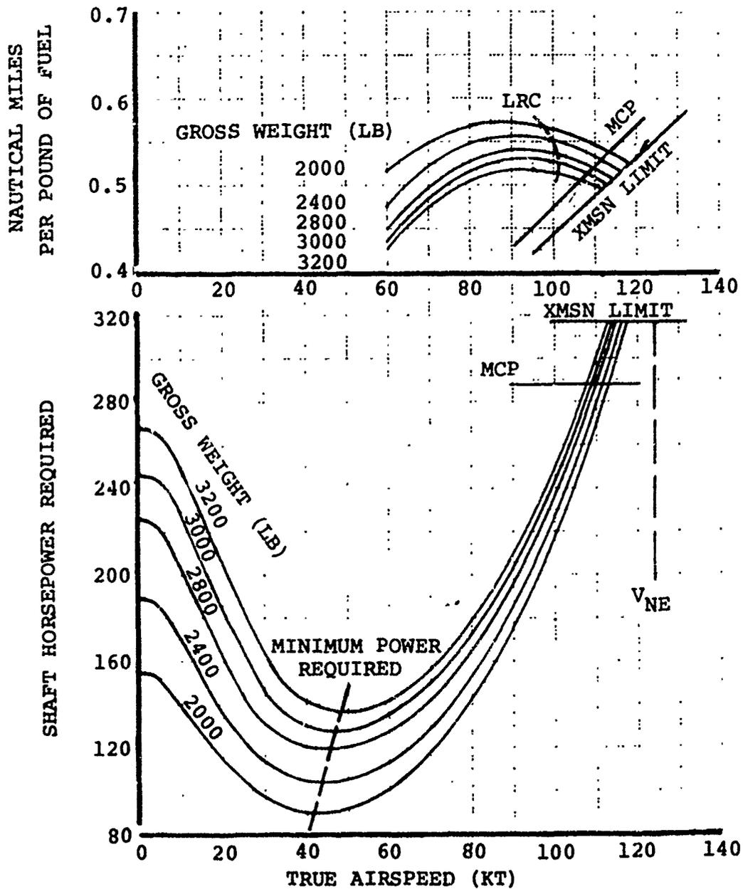
Figure 88. Level Flight Performance, Sea Level, 95°F, Composite Blades
