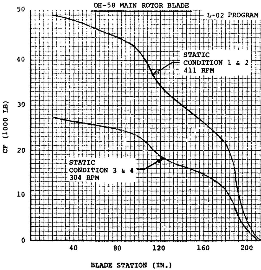
Figure 103. Spanwise Distribution of Centrifugal Force, 304 & 411 rpm
