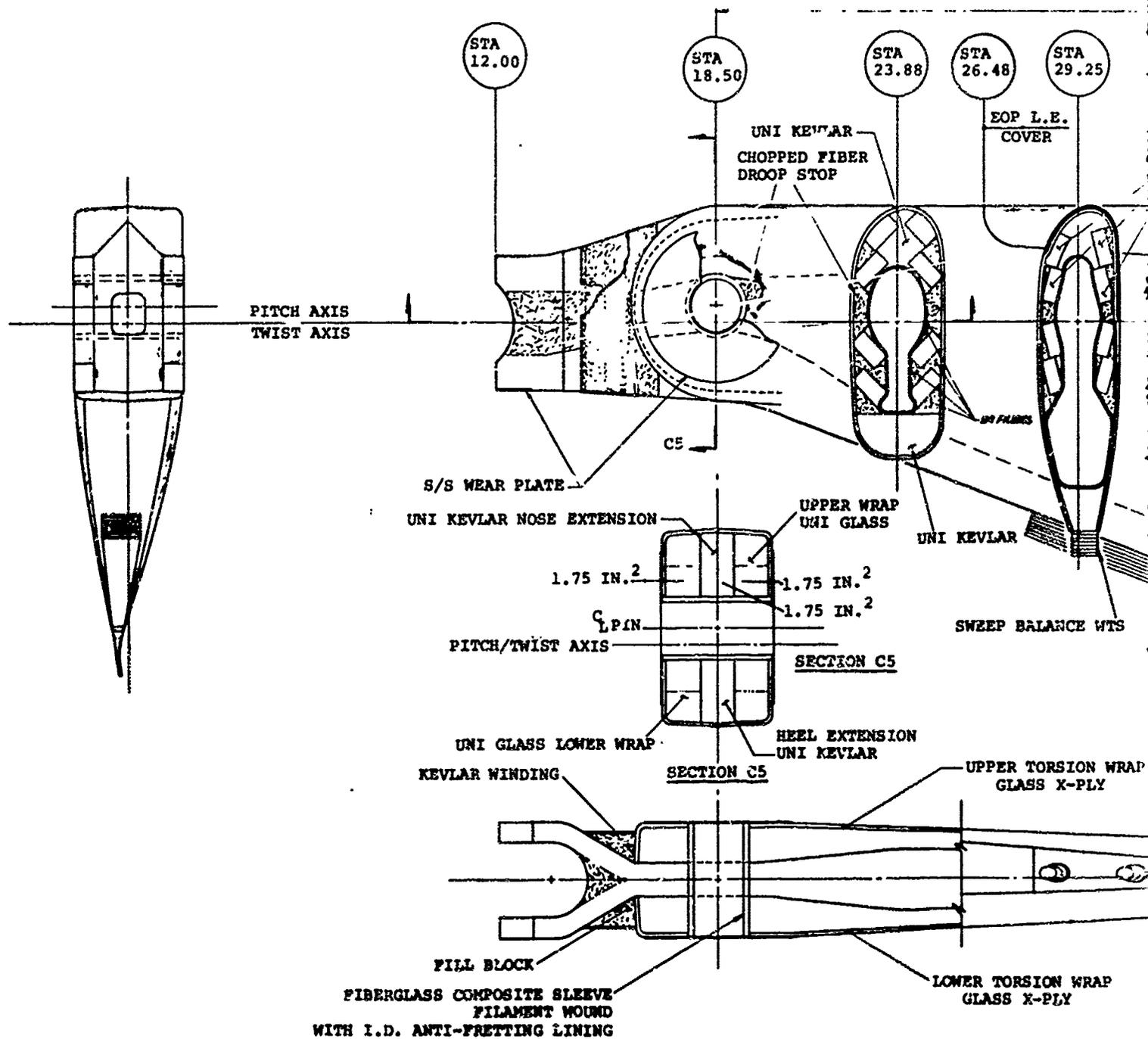
Figure 2. Details of Inboard OH-58C/A Composite Blade
