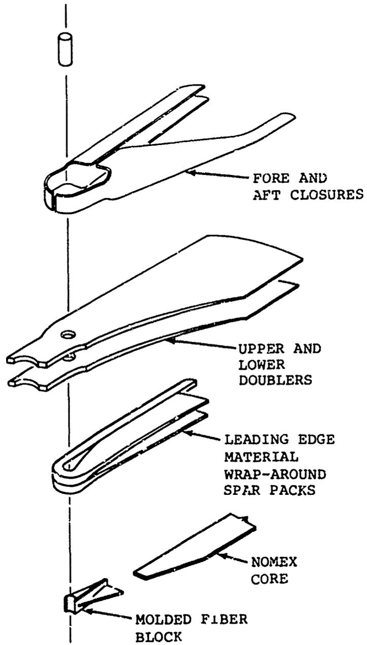
Figure 10. Nose-Wrap Root End Design
