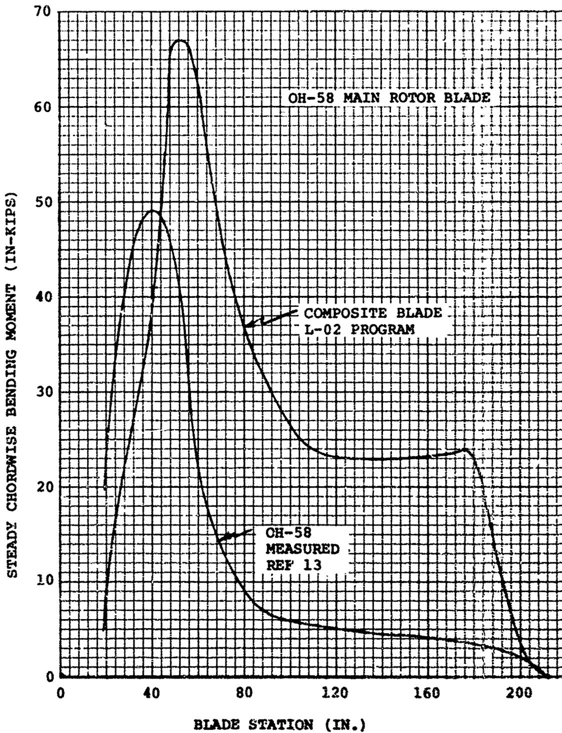
Figure 113. Steady Chord Bending Moment Spanwise Distribution
