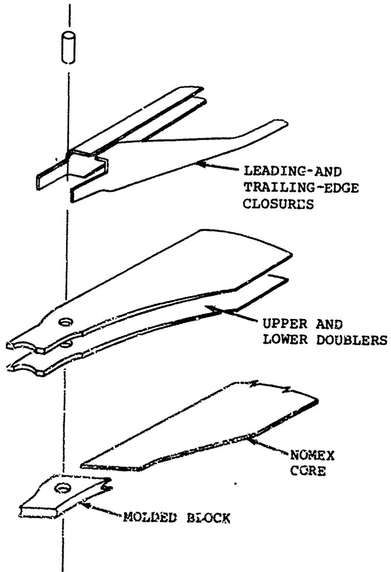
Figure 13. Laminate Root End Design
