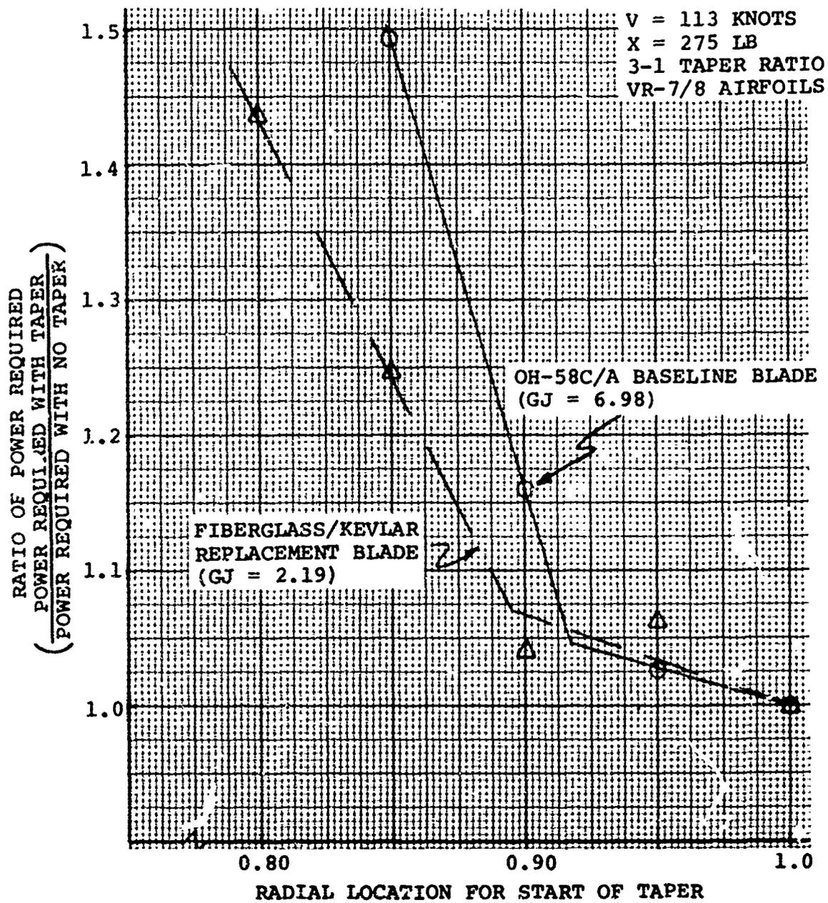
Figure 39. OH-58 C/A Stall Flutter Inception vs. Taper Location
