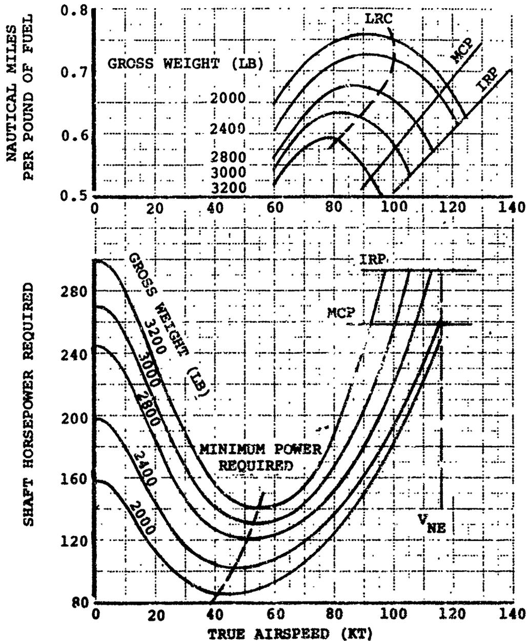
Figure . Level Flight Performance, 10000 Ft, Standard Day Composite Blades
