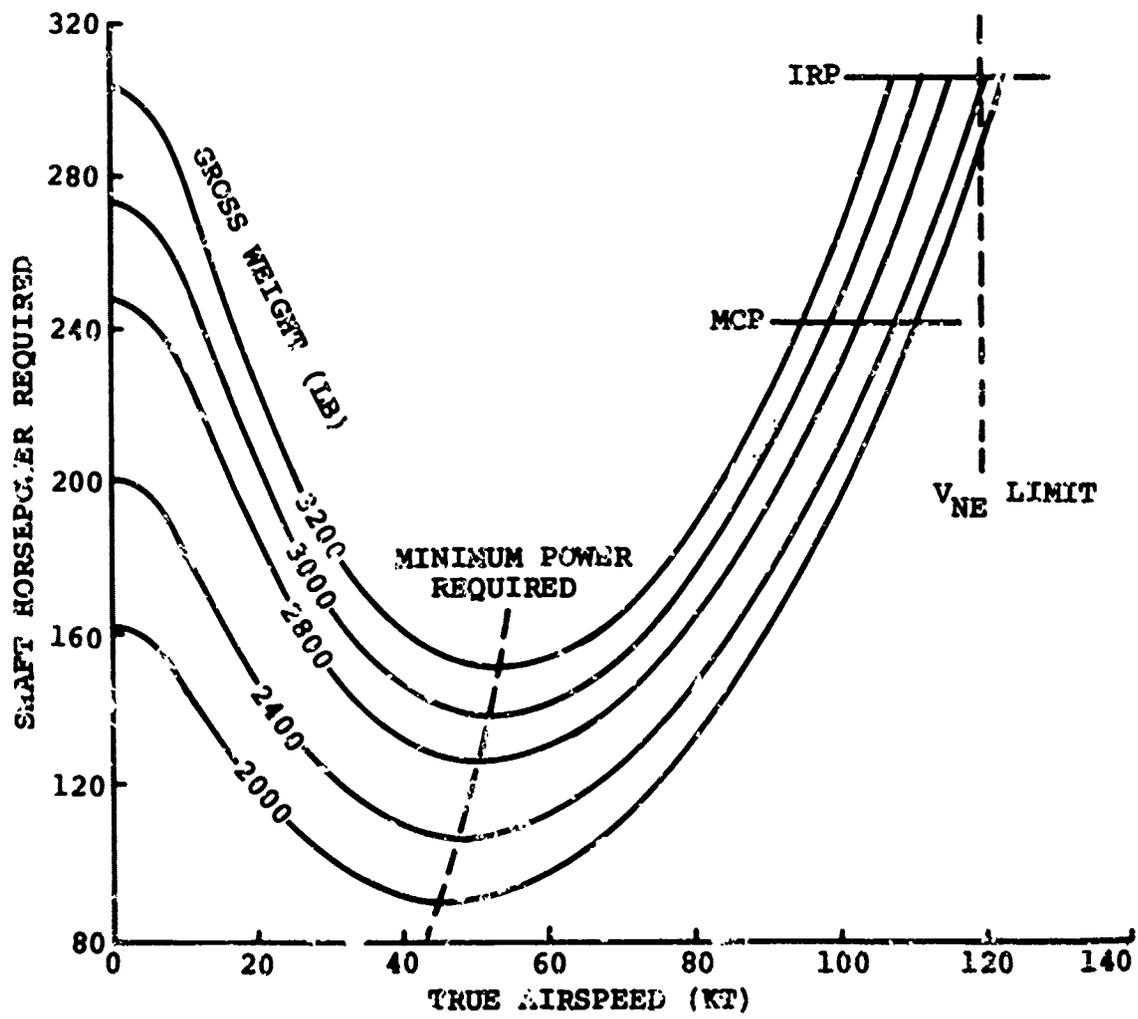
Figure 91. Level Flight Performance, 4000 Feet,
