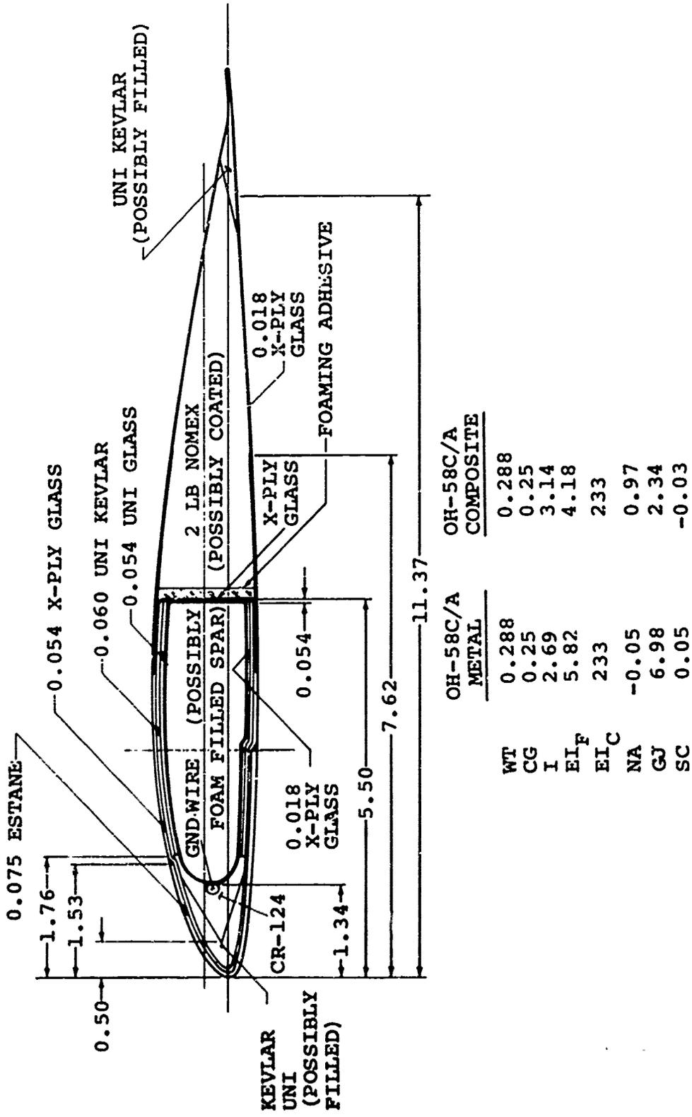
Figure 1. OH-58C/A Composite Rotor Airfoil Cross Section and Comparative Section Properties
