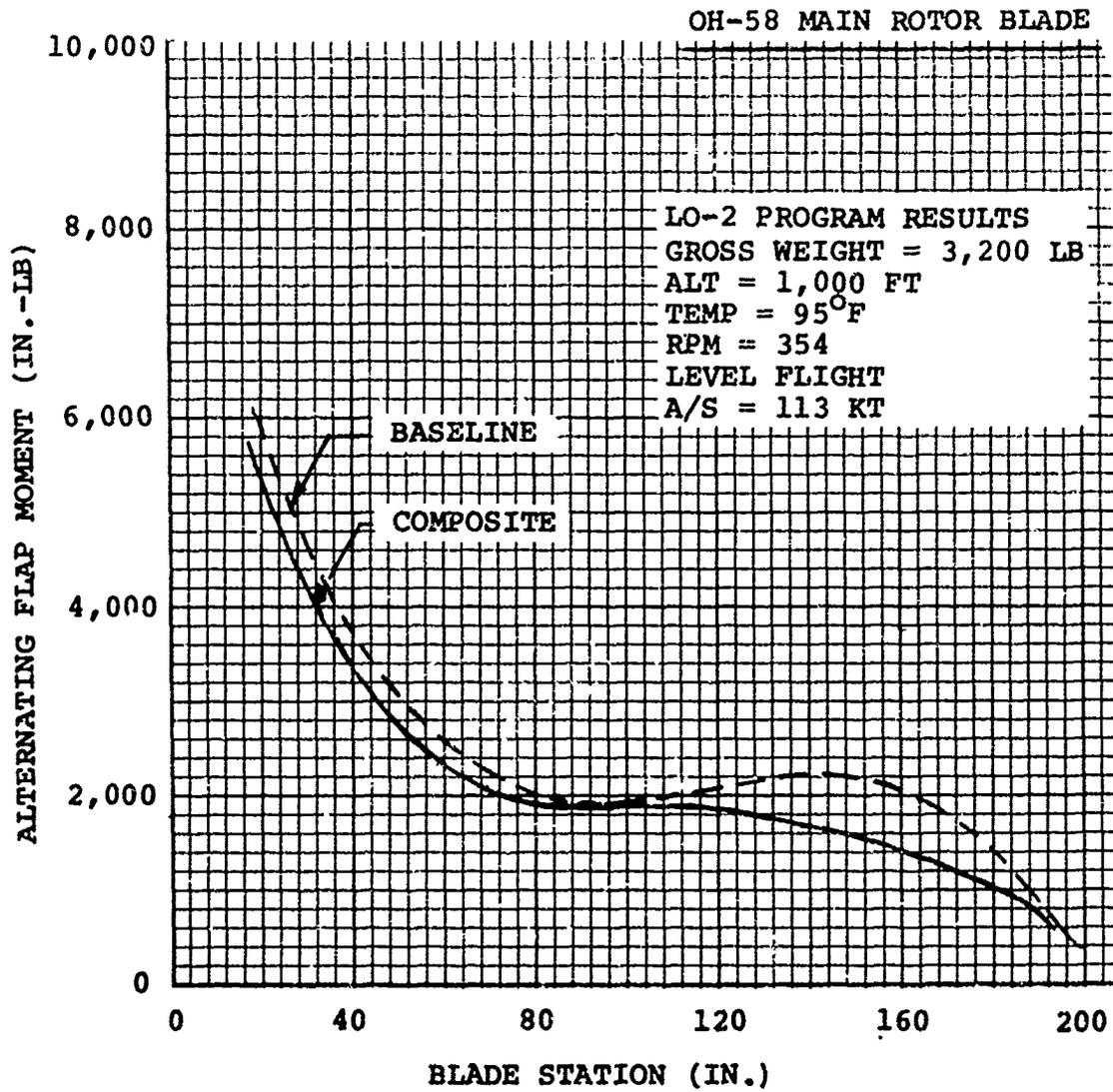
Figure 111. Calculated Alternating Flapwise Bending Moments
