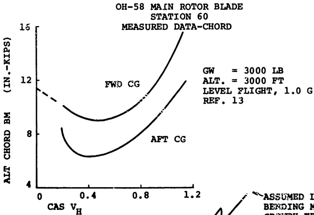
Figure 106. Alternating Chord Moment Vs Airspeed
