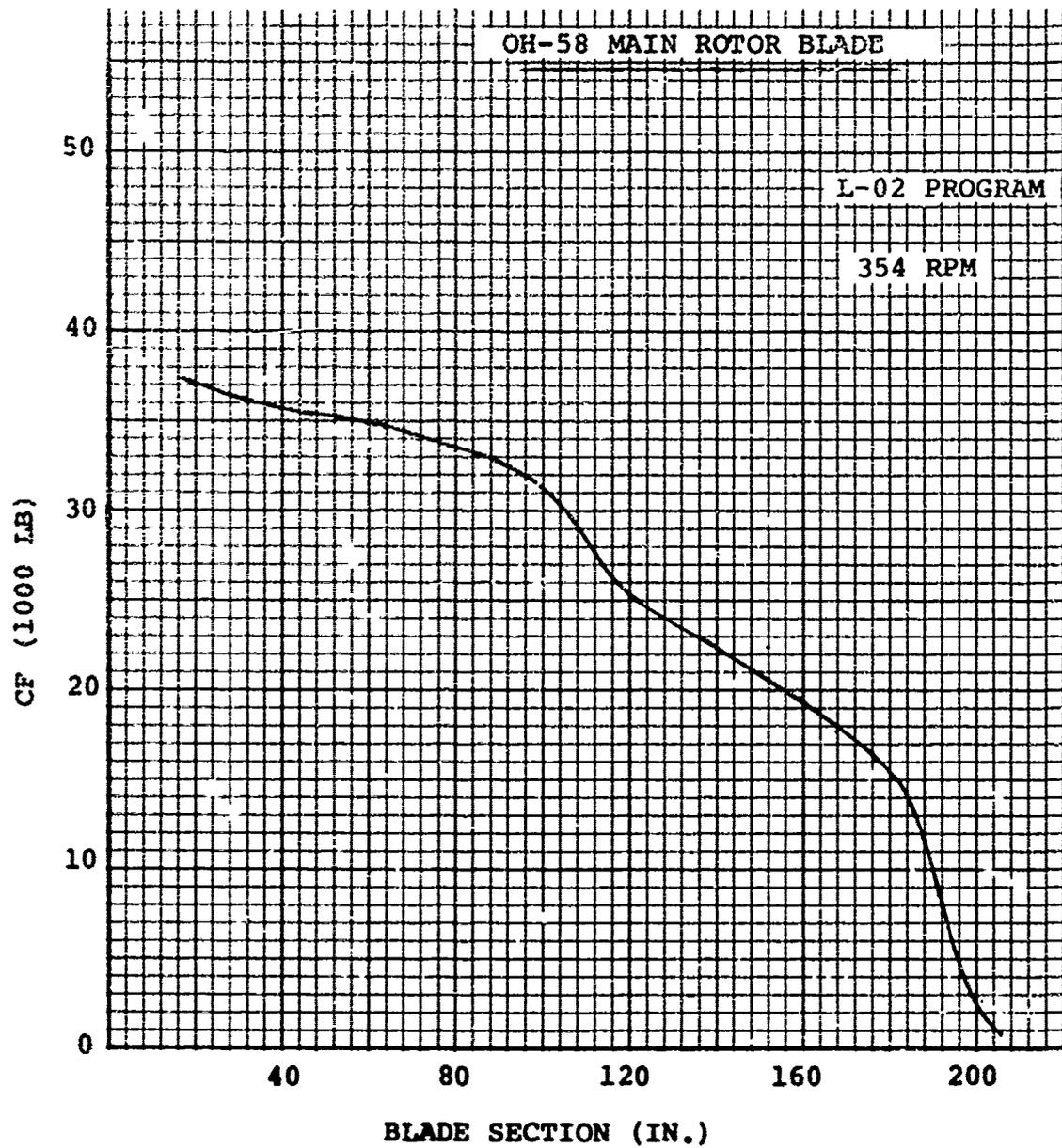
Figure 114. Spanwise Distribution of Centrifugal Force-Composite Blade
