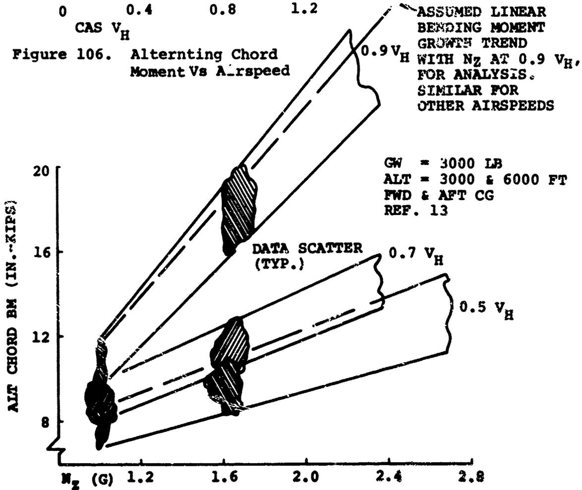
Figure 107. Alternating Chord Moment Vs Maneuver Load Factor
