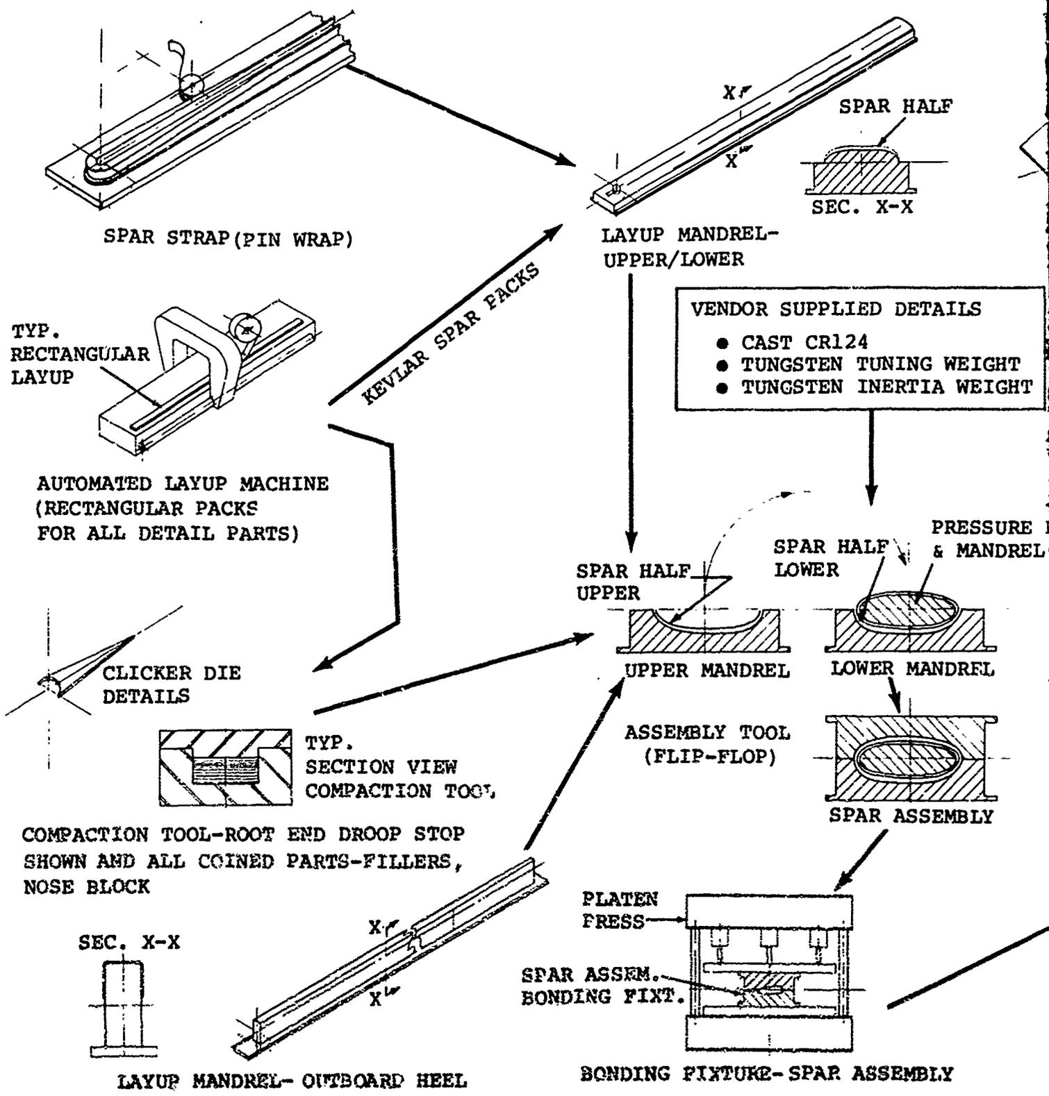
Figure 40. Manufacturing Plan Flow Chart
