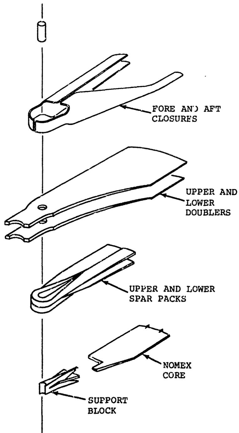
Figure 9. Spar Wrap Root End Design
