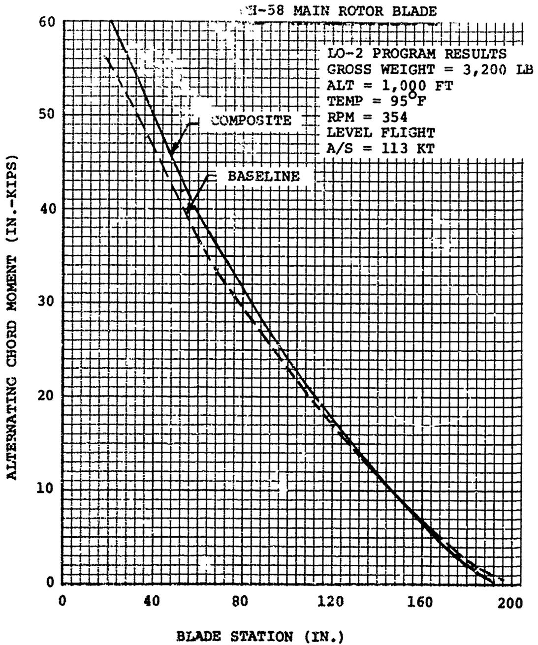
Figure 110. Calculated Alternating Chordwise Bending Moments
