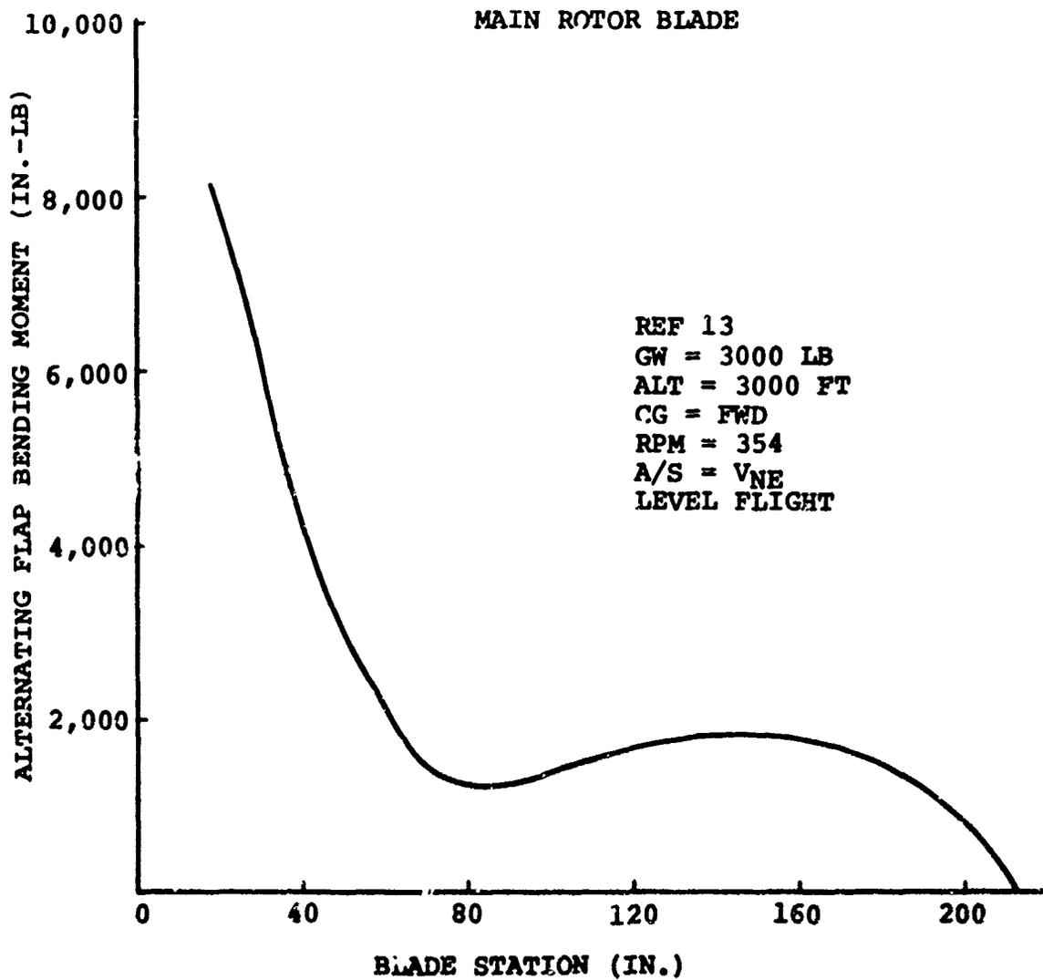
Figure 108. Measured Alternating Flapwise Bending Moment Model 206A-1
