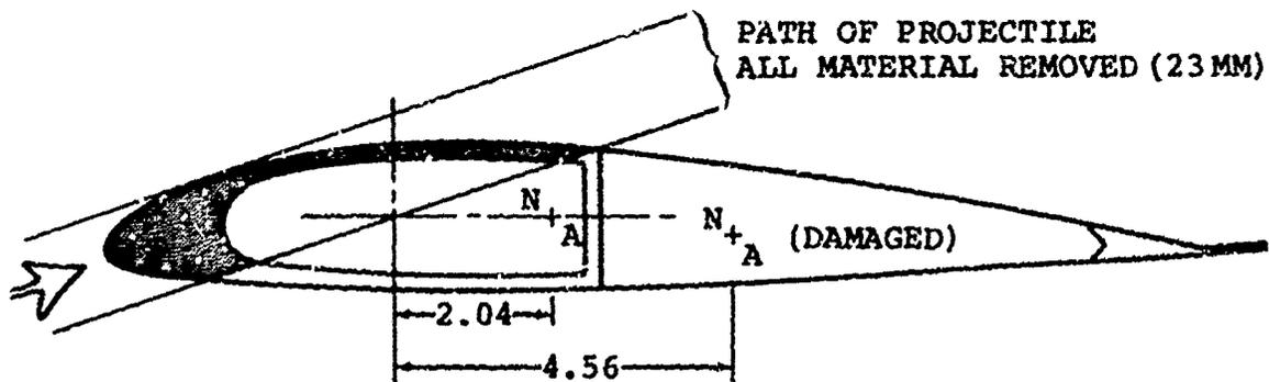
CONSIDER HIT AT BLADE STA 53 (.25R). JUST BEFORE SPAR MATERIAL BUILDUP FOR INCREASED STIFFNESS AT ROOT, BUT WITH PARTIAL TRAILING EDGE BUILDUP.
