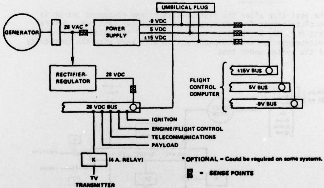
Figure 38. MINI-RPV LVDC With Boxes (Single Output)
