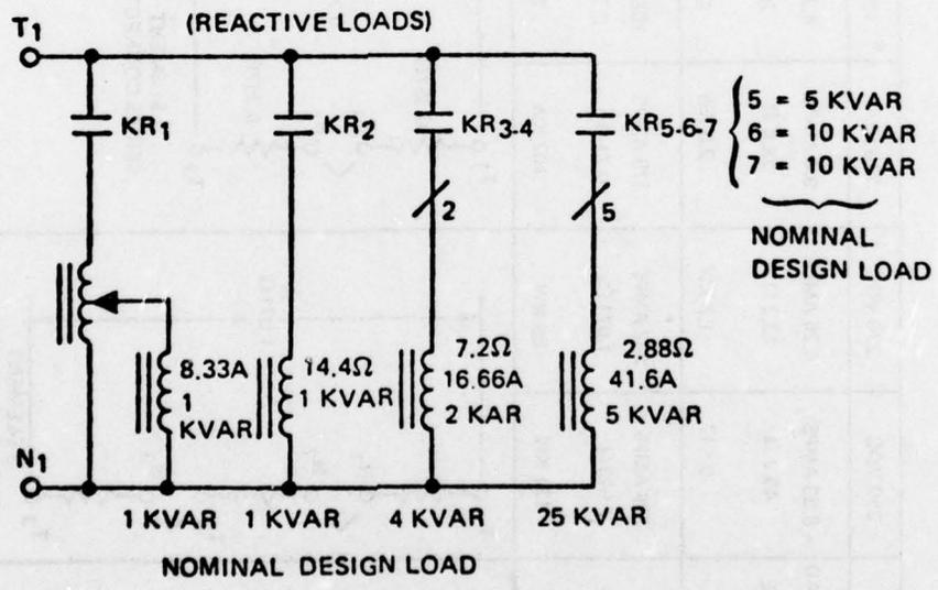
Figure 19. Individual Phase Load Bank Characteristics
