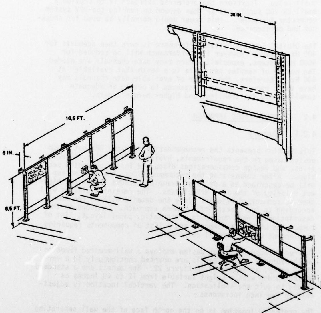
Figure 22. Hot Bench Design Wall Mounted Frame
