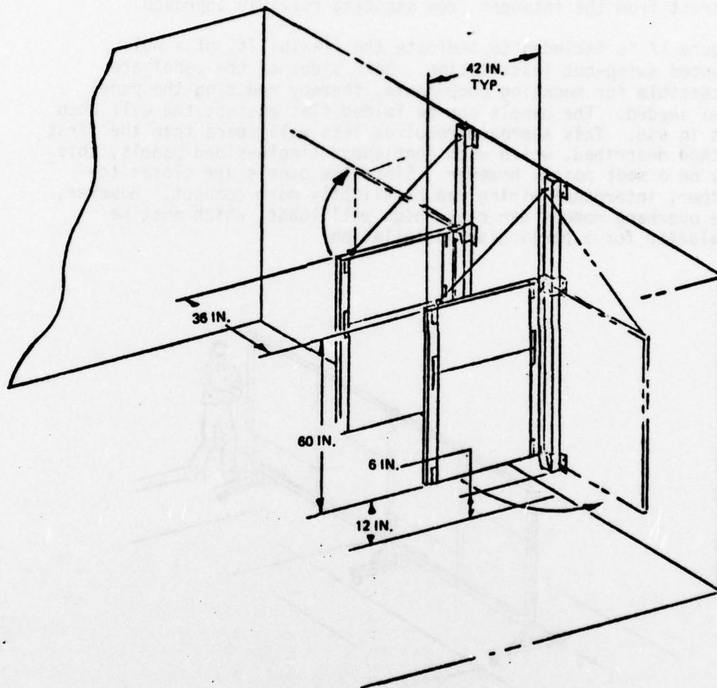
Figure 17. Swing-out Mockup Configuration
