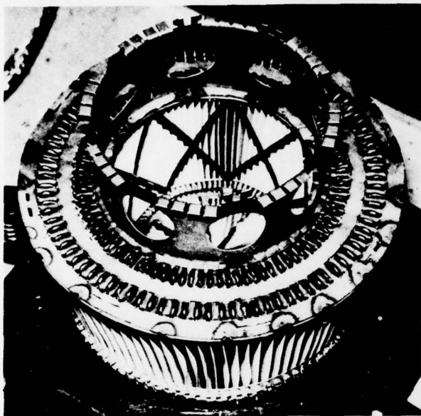
Figure 8. Cathode vanes individually welded to current feed ring.
