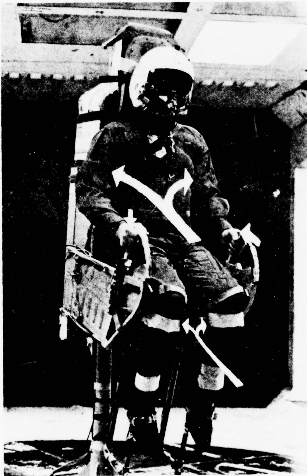
Figure 5. Some sites of flow stagnation for an ejection seat occupant sitting in the ACES-II Seat (See arrows).
