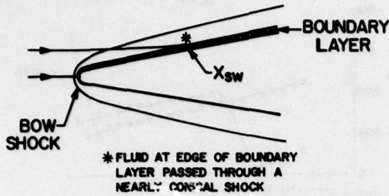
Figure 7 A schematic illustration of flow over a slender, blunt cone.
