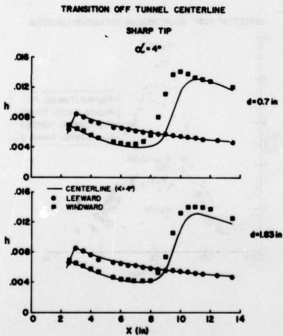
Figure 4 Heat transfer coefficient distributions for the sharp cone with a 4-degree bent sting at three positions.
