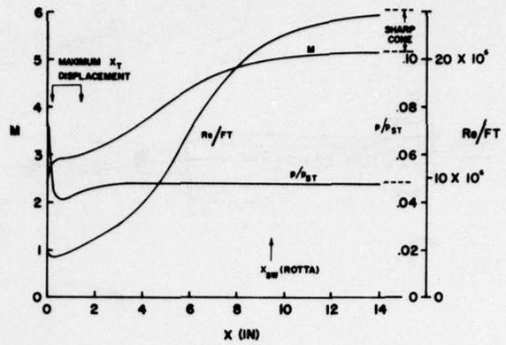
Figure 9 Calculations of local flow properties on a 8-degree half angle cone with 2% bluntness ( $R_N=0.04$  inches) at  $M_\infty = 5.9$
