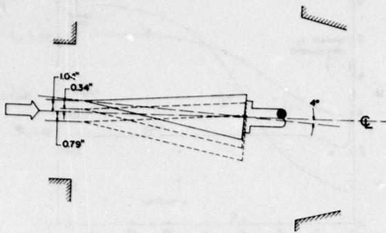
Figure 3 Sharp cone positions with a 4-degree bent sting
