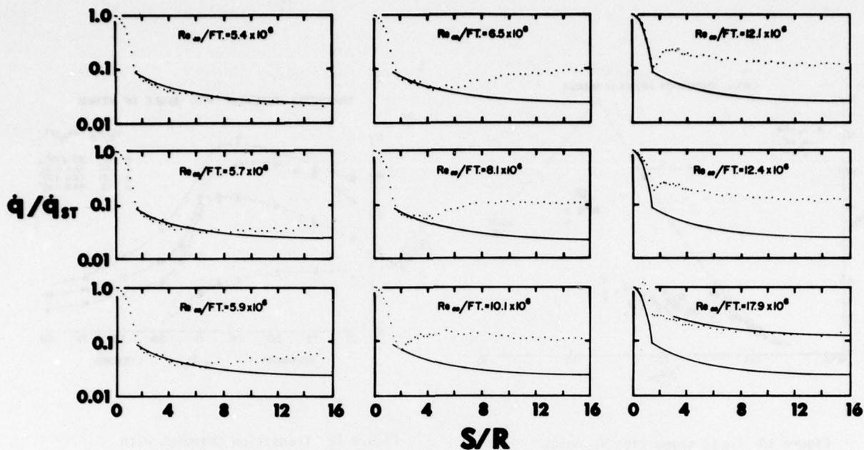
Figure 11 Transition movement from cone frustum to nose tip on a 7-degree half angle cone at  $M_\infty = 9.1$
