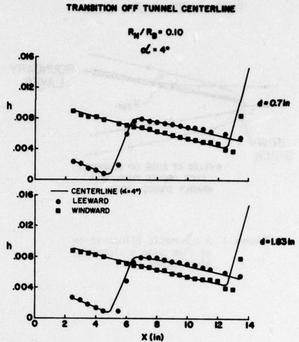
Figure 5 Heat transfer coefficient distributions for the 10% blunt cone with a 4-degree bent sting at three positions
