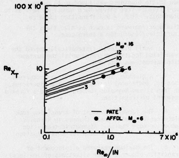
Figure 1 Effect of Mach number and unit Reynolds number on sharp cone transition for small size wind tunnels ( $Re_x$  is the end of transition)  $x_T$  (from Pate<sup>3</sup>)
