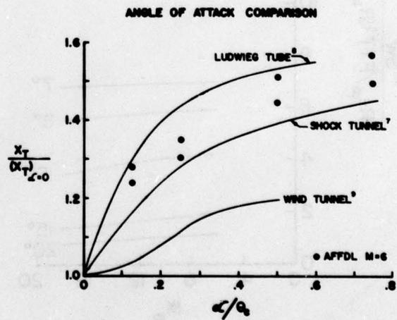
Figure 6 A comparison of the movement of transition on the windward ray of a sharp cone
