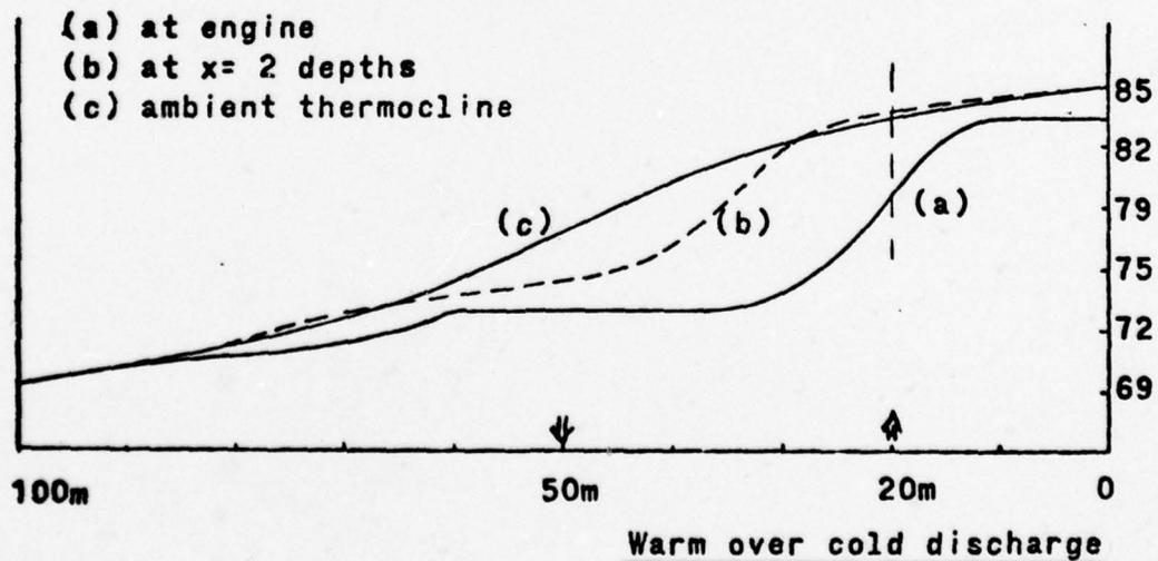
**Figure 2.** Thermocline deformations as a function of discharge configuration and horizontal distance from the power plant. The stratification is typical of the Gulf of Mexico in August.
