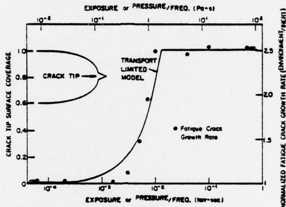
Fig. 9. Comparison between the observed fatigue crack growth response, for 2219-T851 aluminum alloy tested in water vapor at room temperature, and production of a transport-limited model. (After Wei and coworkers, 1979.)
