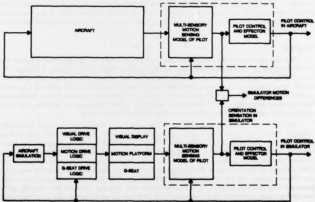
Figure 2. Sensory modeling approach to simulator planning.
