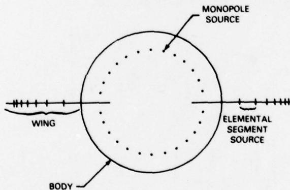
Fig. 10 - Choice of sources for missile cross-section profile
