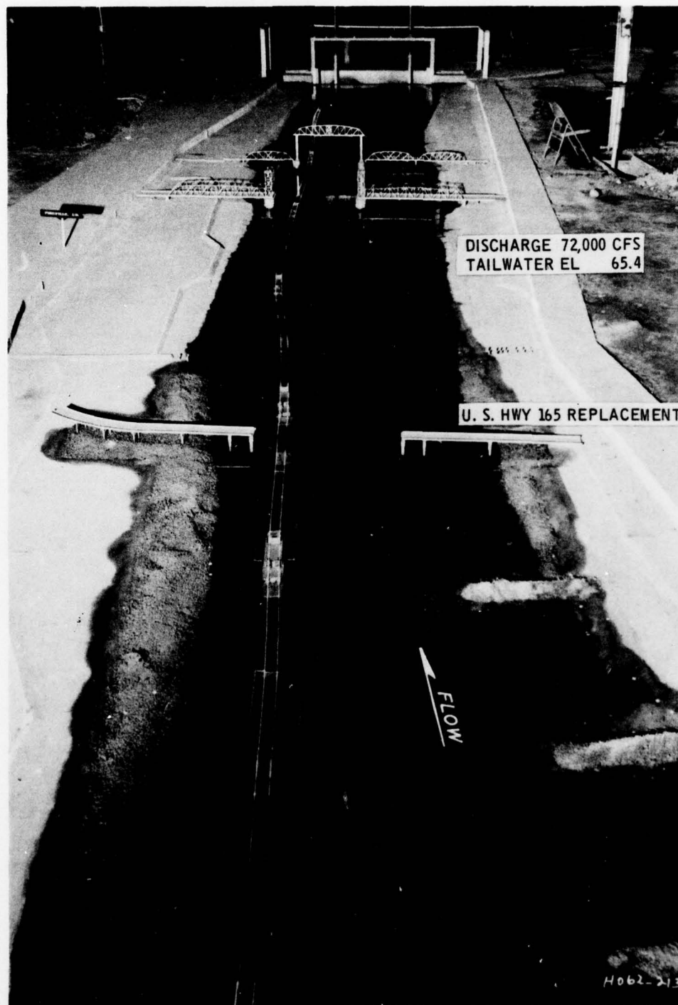
Photo 14. Plan H; Discharge 72,000 cfs, Tailwater el 65.4. Path of downbound tow approaching and passing through the bridges in the lower reach along the left side of the navigation channel. Note tendency for tow to be moved to the left after passing the U. S. Highway 165 replacement bridge
