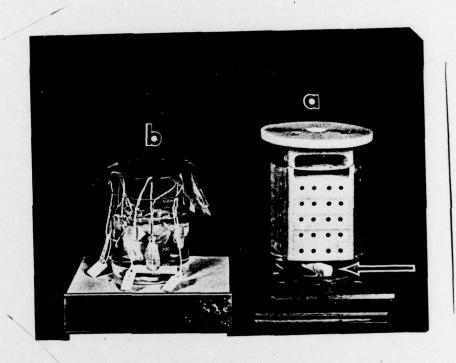
FIGURE 1 The decalcification cabinet (a) in position next to the previously used gauze-wrap technique (b). Note the numerously dispersed openings and the magnetic stirrer (arrow).
