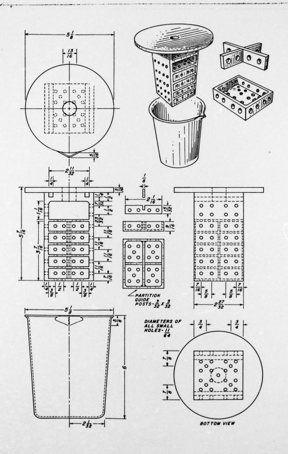
FIGURE 6 Detailed plans for fabrication of the decalcification cabinet.
