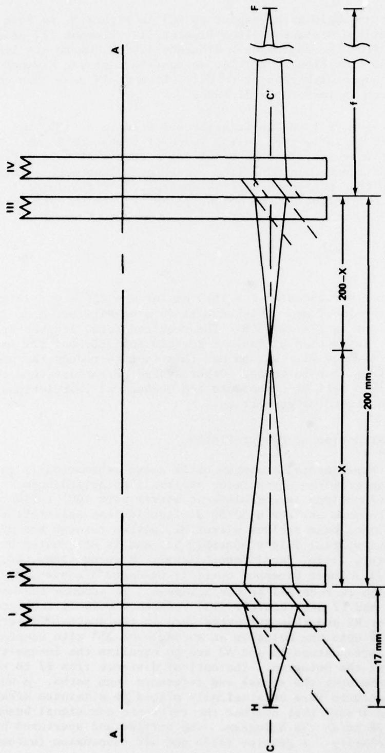
Figure 5. One lens group of the holographic zoom lens system with an input object H and an output image F. (The spacing between I and II and the spacing between II and IV are greatly exaggerated.)
