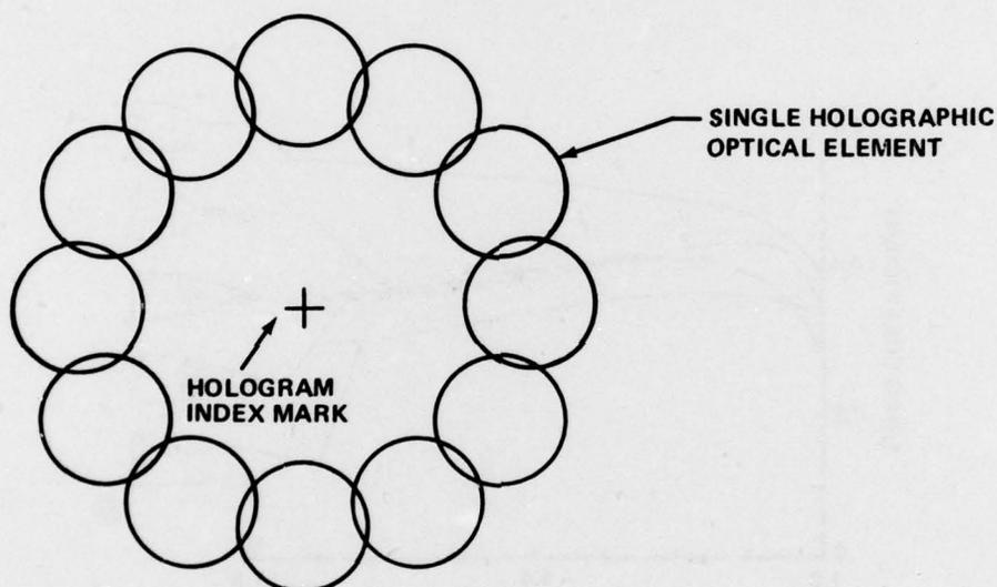
Figure 4. Design selected for demonstrator (12 discrete elements).
