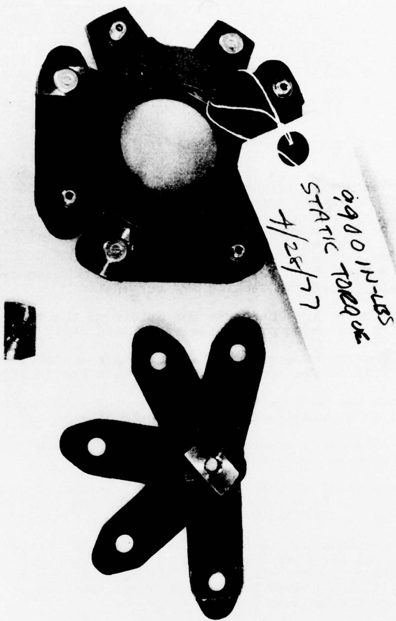
Figure 75. Static Torque Test - Composite Strap Coupling.
