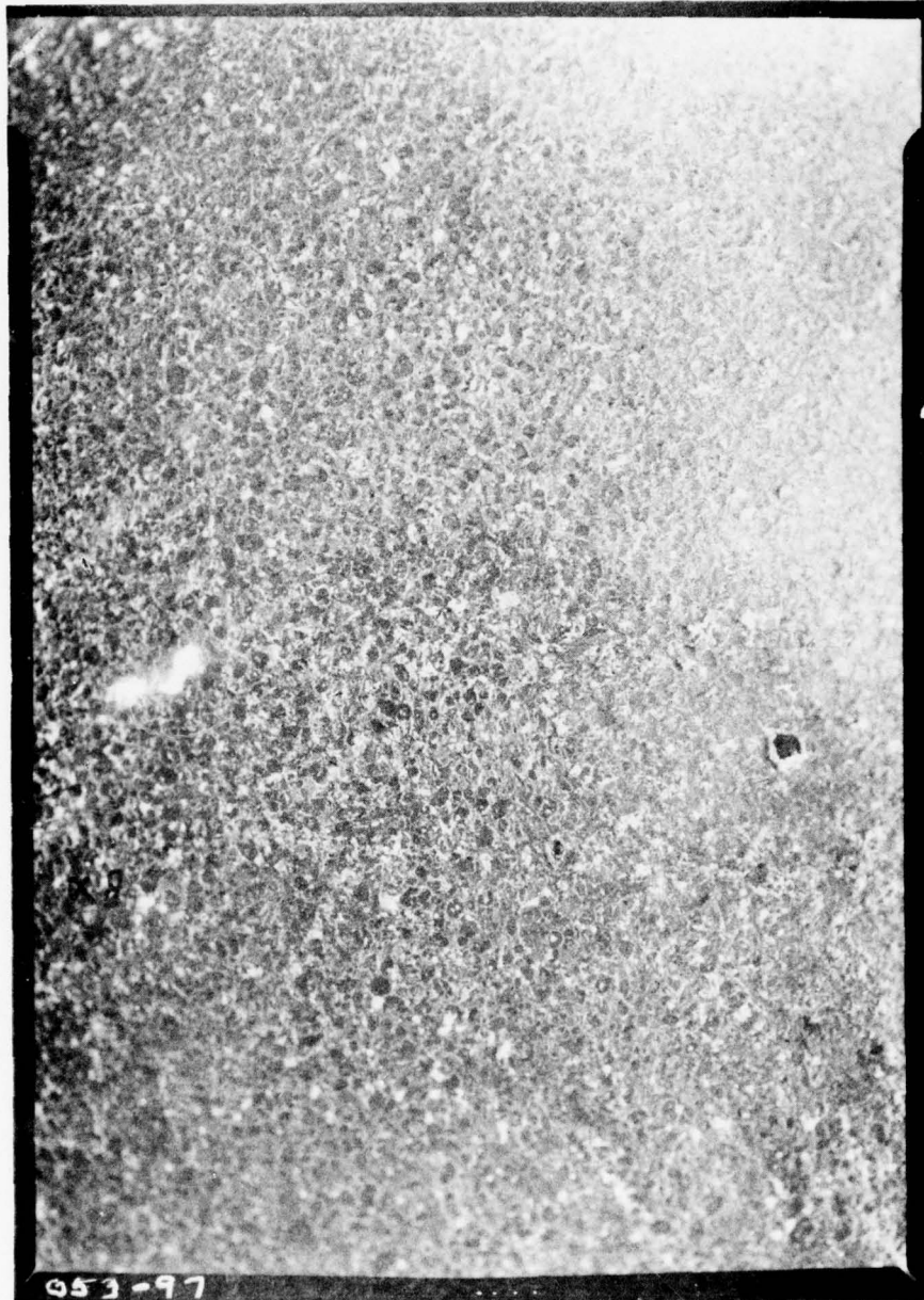
Figure 15. Etched surface casting of batch process Comp B Lot 053-97 (8X).
