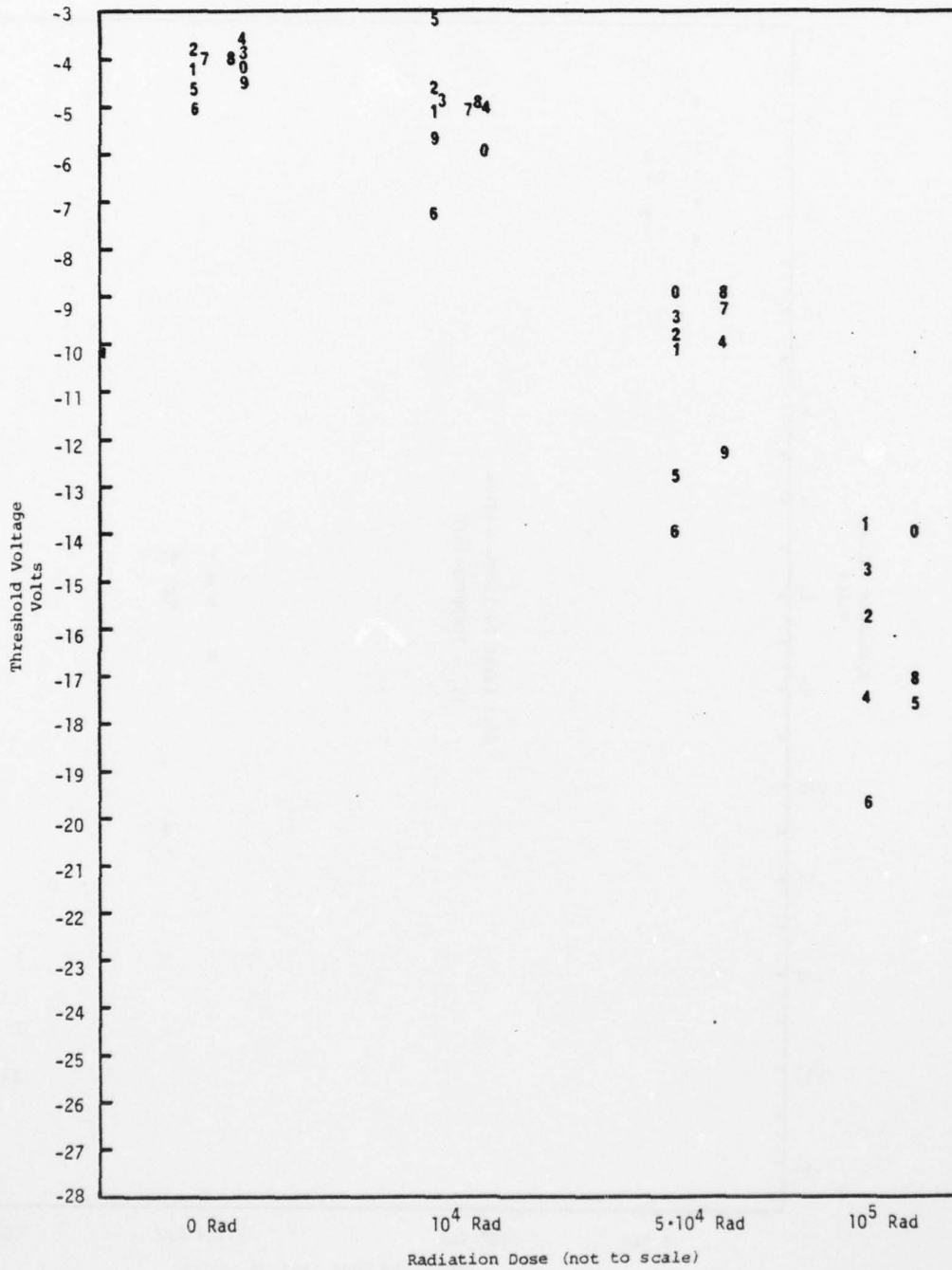
Figure 38. Threshold Voltage vs. Radiation Dose for 3N174 MOSFETs as Derived from Curve Tracer Data.
